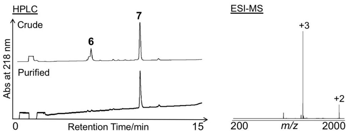
**Figure S2:** HPLC chromatogram and ESI-MS spectrum of **7**. ESI-MS:  $m/z$  calcd for  $C_{165}H_{245}N_{19}O_{83}$ :  $[M+H]^+$  3822.83, observed (deconvoluted): 3822.60;  $[M+2H]^{2+}$  1912.42, found for 1912.3;  $[M+3H]^{3+}$  1275.28, found for 1275.10.
