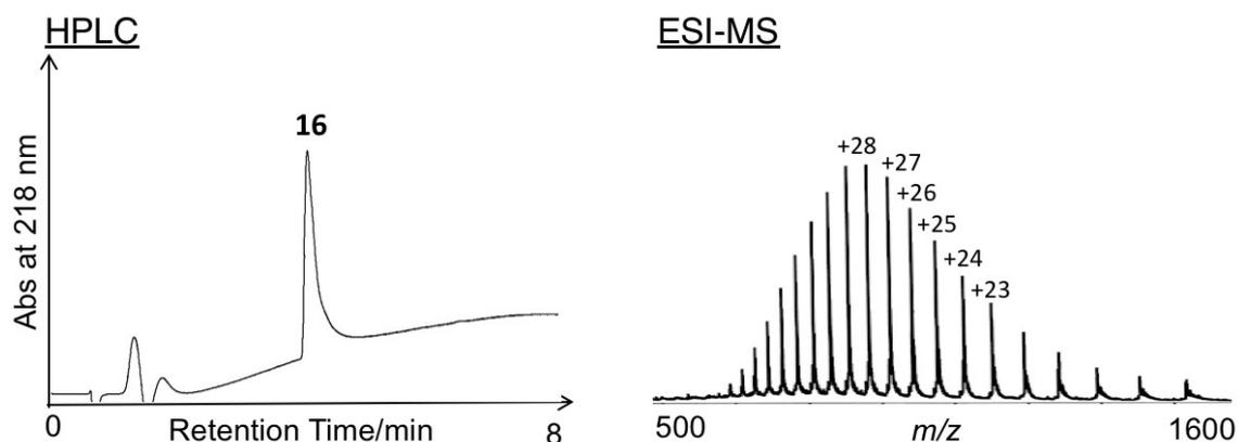
**Figure S13:** HPLC chromatogram and ESI-MS spectrum of 16. ESI-MS:  $m/z$  calcd for C<sub>972</sub>H<sub>1528</sub>N<sub>280</sub>O<sub>281</sub>S<sub>8</sub>: [M+H]<sup>+</sup> 21875.16, observed (deconvoluted): 21872.55; [M+27H]<sup>27+</sup> 811.19, found for 811.09.
