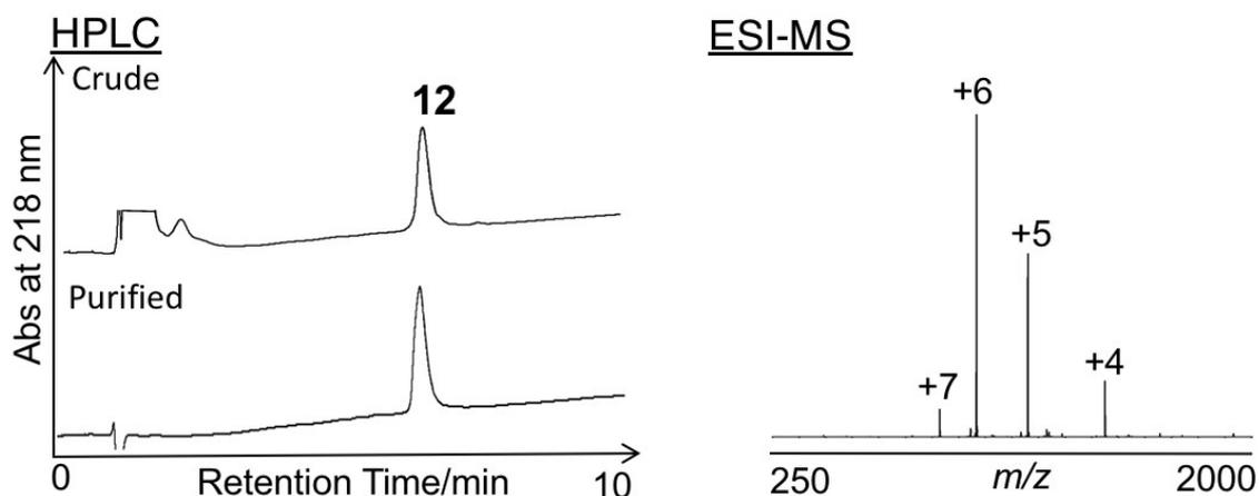
**Figure S7:** HPLC chromatogram and ESI-MS spectrum of **12**. ESI-MS:  $m/z$  calcd for  $C_{254}H_{395}N_{67}O_{80}S_4$ :  $[M+H]^+$  5795.58, observed (deconvoluted): 5795.08;  $[M+4H]^{4+}$  1449.90, found for 1449.72;  $[M+5H]^{5+}$  1160.12, found for 1159.98;  $[M+6H]^{6+}$  966.85, found for 966.82;  $[M+7H]^{7+}$  828.94, found for 828.84.
