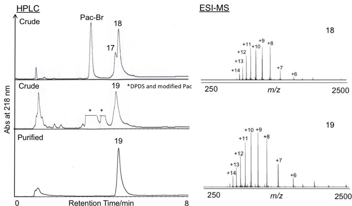
**Figure S15:** HPLC chromatogram and ESI-MS spectrum of Pac-protected Thz-Segment-D **18** and Cys-Segment-D **19**. ESI-MS:  $m/z$  calcd for **18**;  $C_{447}H_{689}N_{123}O_{114}S_3$ :  $[M+H]^+$  9706.36, observed (deconvoluted): 9706.07;  $[M+6H]^{6+}$  1618.73, found for 1618.51;  $[M+8H]^{8+}$  1214.30, found for 1214.14;  $[M+11H]^{11+}$  883.40, found for 883.37.
