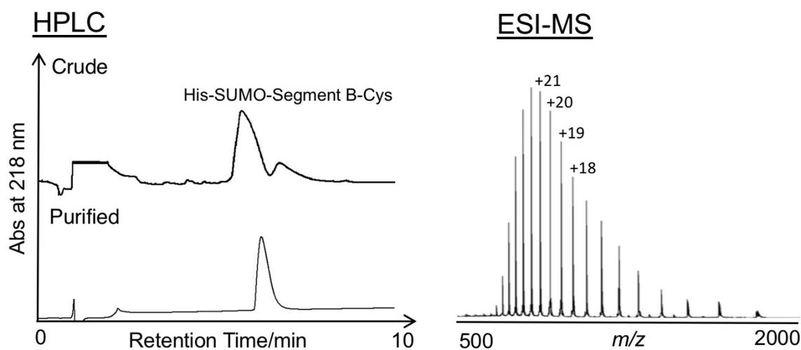
**Figure S5:** HPLC chromatogram and ESI-MS spectrum of His-SUMO-Segment B-Cys. ESI-MS:  $m/z$  calcd for  $[M+H]^+$  18053.04, observed (deconvoluted): 18052.31;  $[M+18H]^{18+}$  1003.95, found for 1003.90;  $[M+19H]^{19+}$  951.16, found for 951.12;  $[M+20H]^{20+}$  903.65, found for 903.61;  $[M+21H]^{21+}$  860.67, found for 860.63.
