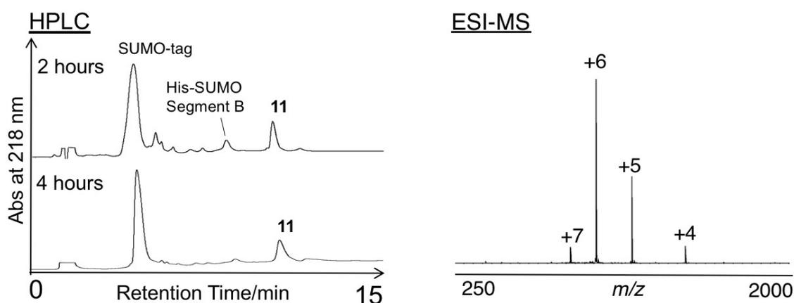
**Figure S6:** HPLC chromatogram and ESI-MS spectrum of **11**. ESI-MS:  $m/z$  calcd for  $\text{C}_{253}\text{H}_{396}\text{N}_{66}\text{O}_{80}\text{S}_4$ :  $[\text{M}+\text{H}]^+$  5770.57, observed (deconvoluted): 5769.72;  $[\text{M}+4\text{H}]^{4+}$  1443.64, found for 1443.34;  $[\text{M}+5\text{H}]^{5+}$  1155.11, found for 1154.87;  $[\text{M}+6\text{H}]^{6+}$  962.76, found for 962.56.
