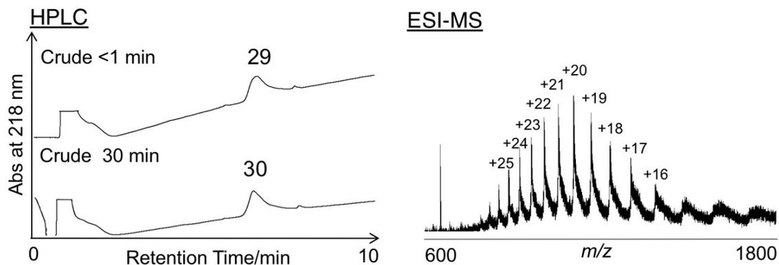
**Figure S21:** HPLC chromatogram and ESI-MS spectrum of **30**. HRMS (ESI):  $m/z$  calcd for  $C_{992}H_{1544}N_{252}O_{313}S_7$ :  $[M+H]^+$  22233.1350, observed: 22233.7281.  $[M+18H]^{18+}$  1236.1742, found for 1236.1626;  $[M+19H]^{19+}$  1171.1650, found for 1171.1214;  $[M+20H]^{20+}$  1112.6568, found for 1112.6975;  $[M+21H]^{21+}$  1059.7207, found for 1059.7156;  $[M+22H]^{22+}$  1011.5971, found for 1011.5603.
