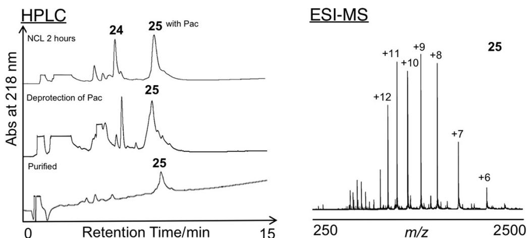
**Figure S17:** HPLC chromatogram and ESI-MS spectrum of **25**. HRMS (ESI):  $m/z$  calcd for C<sub>554</sub>H<sub>865</sub>N<sub>131</sub>O<sub>200</sub>S<sub>5</sub>: [M+H]<sup>+</sup>, 12721.0310, observed (deconvoluted): 12721.0048. [M+6H]<sup>6+</sup> 2121.1718 found for 2121.1708; [M+7H]<sup>7+</sup> 1818.2901, found for 1818.2934; [M+8H]<sup>8+</sup> 1591.1289, found for 1591.1265; [M+9H]<sup>9+</sup> 1414.4479, found for 1414.4444; [M+11H]<sup>11+</sup> 1157.4574, found for 1157.4529.
