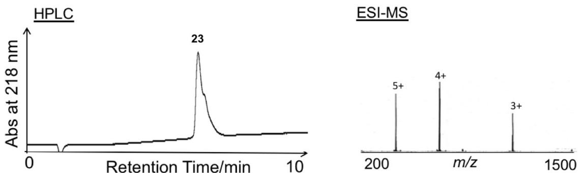
**Figure S12:** The HPLC profile and ESI-MS spectra of IFN- $\beta$ -(1-30) Segment A-hydrazide **23**. ESI-MS:  $m/z$  calcd for  $C_{165}H_{255}N_{47}O_{44}S_2$ :  $[M+H]^+$  3665.26, observed (deconvoluted): 3665.03;  $[M+3H]^{3+}$  1222.75, found for 1222.61;  $[M+4H]^{4+}$  917.32, found for 917.21;  $[M+5H]^{5+}$  734.05, found for 733.97.
