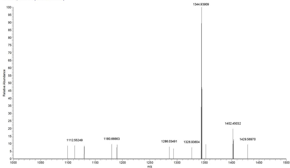
**Figure S5.** The ESI mass spectrum for 1:1 complex  $Z-1^{2+}@Q[7]$ .
