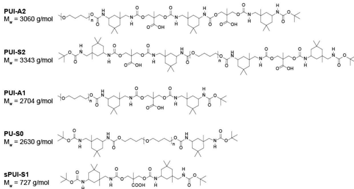
*Scheme S1: Molecular structures of the PU(I) materials as used in this study. The average molar mass of pTHF is about 2 kDa. Given molecular weight values are for pTHF chains with 28 THF-units. Note that the IPDA building blocks exist in multiple regio- and stereoisomers; this is not shown for brevity.*
