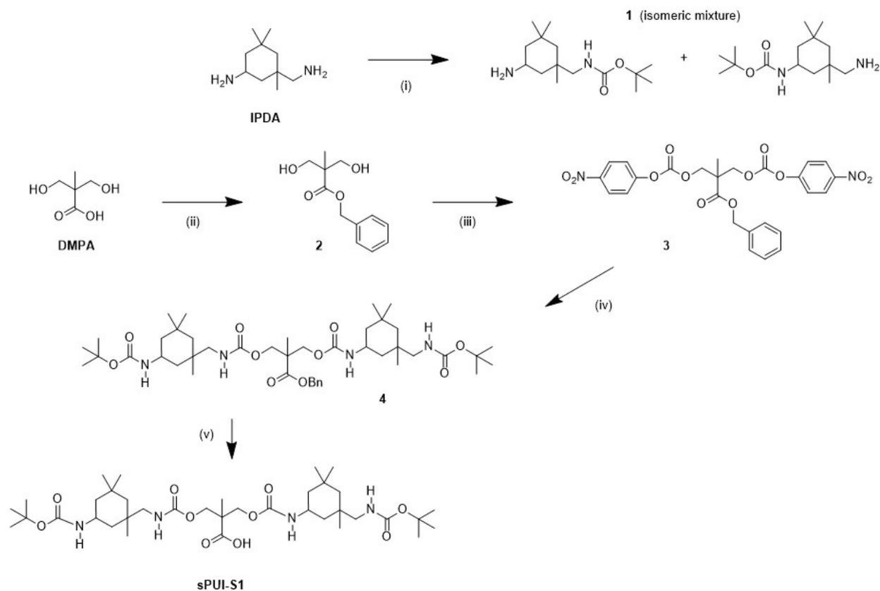
*Scheme S2: Synthesis route to small polyurethane ionomer sPUI-S1. (i) Boc-anhydride, DCM; (ii) BnBr, KOH, DMF, 100°C; (iii) 4-nitrophenyl chloroformate, pyridine, DCM; (iv) amine 1, pyridine, dioxane, reflux; (v) Pd/C, H<sub>2</sub>, iso-propanol. Note that the IPDA building blocks exist in multiple regio- and stereoisomers; this is not shown for brevity.*
