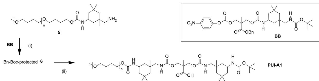
*Scheme S3: Synthesis route to the asymmetric polyether-urethane ionomer **PUI-A1**. (i) **BB**, pyridine, dioxane, reflux; (ii) Pd/C, H<sub>2</sub>, dioxane. Note that the IPDA building blocks exist in multiple regio- and stereoisomers; this is not shown for brevity.*
