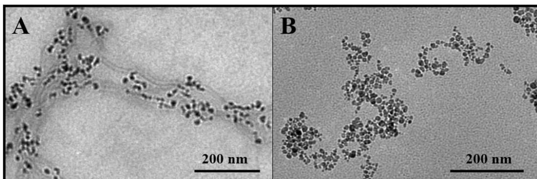
**Figure S5.** TEM images of (A)  $OPV_5-b-P2VP_{25}/Fe_3O_4@SiO_2$  and (B)  $OPV_5-b-P2VP_{27}/Fe_3O_4$  nanofibers after transferring into THF.
