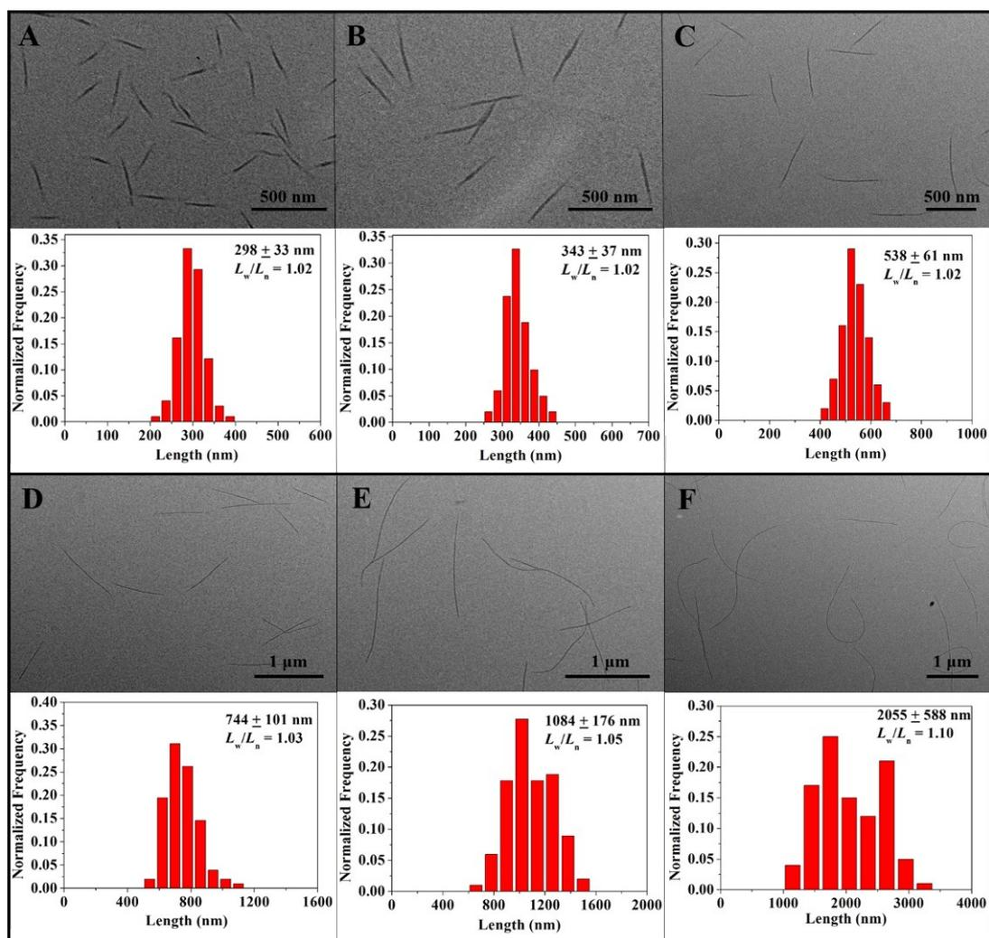
**Figure S3.** TEM images of uniform micelles of  $OPV_5$ -*b*- $P2VP_{25}$  formed by heating seed micelles at (A) 40°C, (B) 42°C, (C) 44°C, (D) 46°C, (E) 48°C and (F) 50°C, followed by cooling/aging at 23°C for 24 h.
