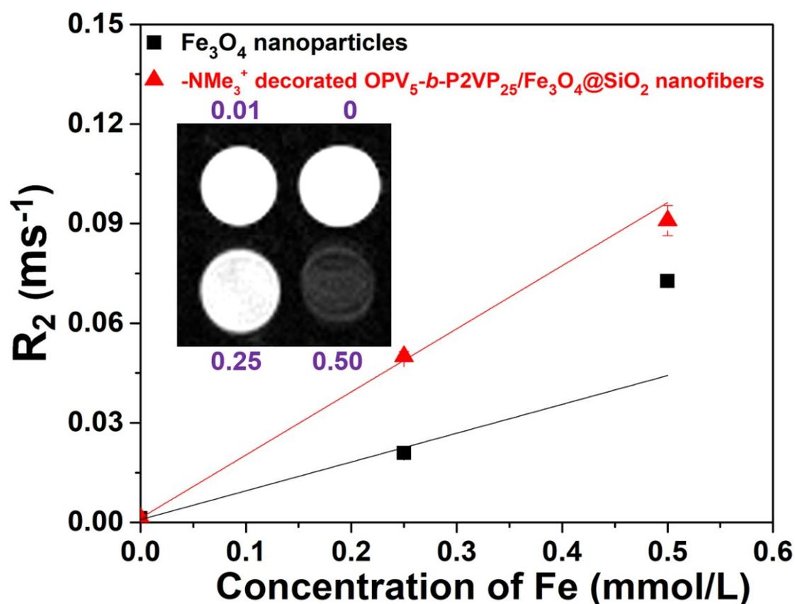
**Figure S7.** Plots of  $R_2$  MRI signal over  $\text{Fe}_3\text{O}_4$  nanoparticles and  $-\text{NMe}_3^+$  decorated OPV<sub>5</sub>-*b*-P2VP<sub>25</sub>/ $\text{Fe}_3\text{O}_4$ @ $\text{SiO}_2$  with series concentrations of Fe. The inset shows  $T_2$ -weighted MRI phantom images of  $\text{Fe}_3\text{O}_4$  nanoparticles with series concentrations of Fe.
