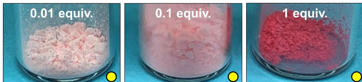
Figure S23. Image of the photoredox polymer catalyst EY-PMMA with 0.01, 0.1, and 1 equiv of EYMA after purification.
