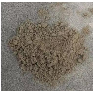
**Figure S6.** Dry powder of 1,3-Bis(2-isocyanato-2-propyl)benzene x ethylenediamine capsules.
