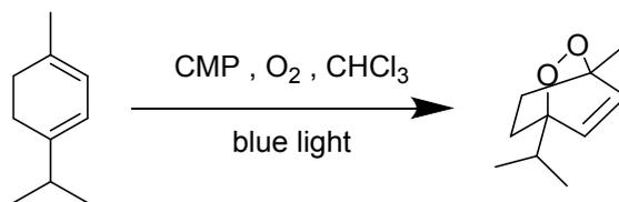
Reaction conditions:  $\alpha$ -terpinene (0.5mmol), photocatalyst (2.45mg, 0.5% mmol),  $CHCl_3$ (5mL), air, 24W blue LED lamp, room temperature (RT), 3h; Conversion was determined by  $^1H$  NMR.
