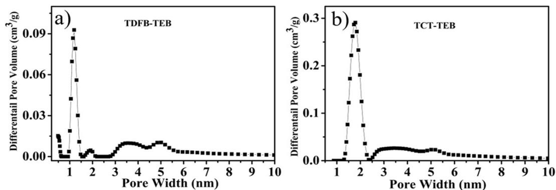
Figure S7. Pore size distribution of a) TDFB-TEB and b) TCT-TEB.
