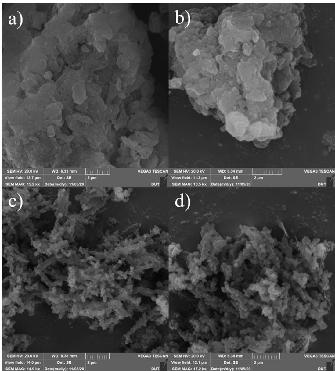
**Figure S9.** SEM images of a), b) TDFB-TEB and c), d) TCT-TEB.
