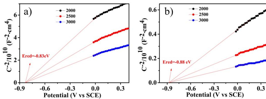
Figure S11. Mott-Schottky plots of a) TDFB-TEB and b) TCT-TEB.
