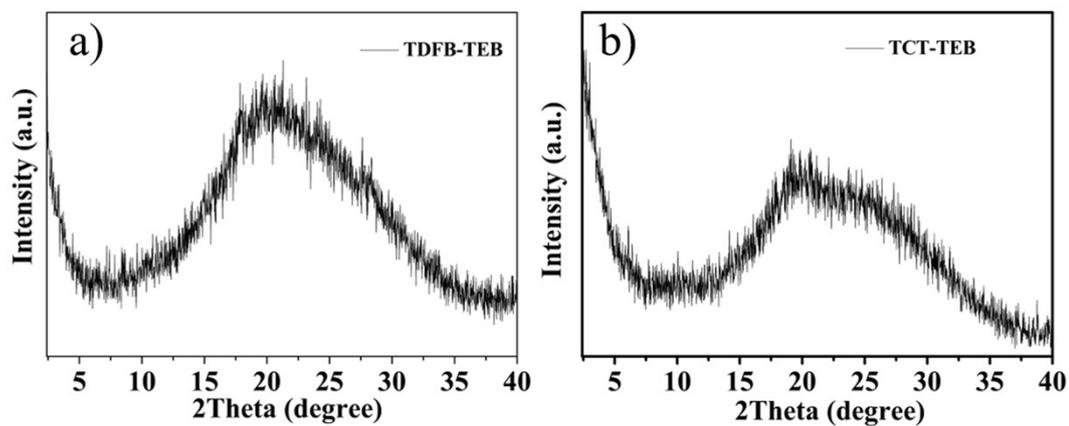
Figure S10. Powder X-ray diffraction pattern of a) TDFB-TEB and b) TCT-TEB.
