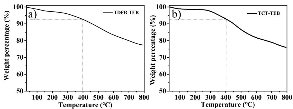
Figure S8. Thermogravimetric analysis of a) TDFB-TEB and b) TCT-TEB.
