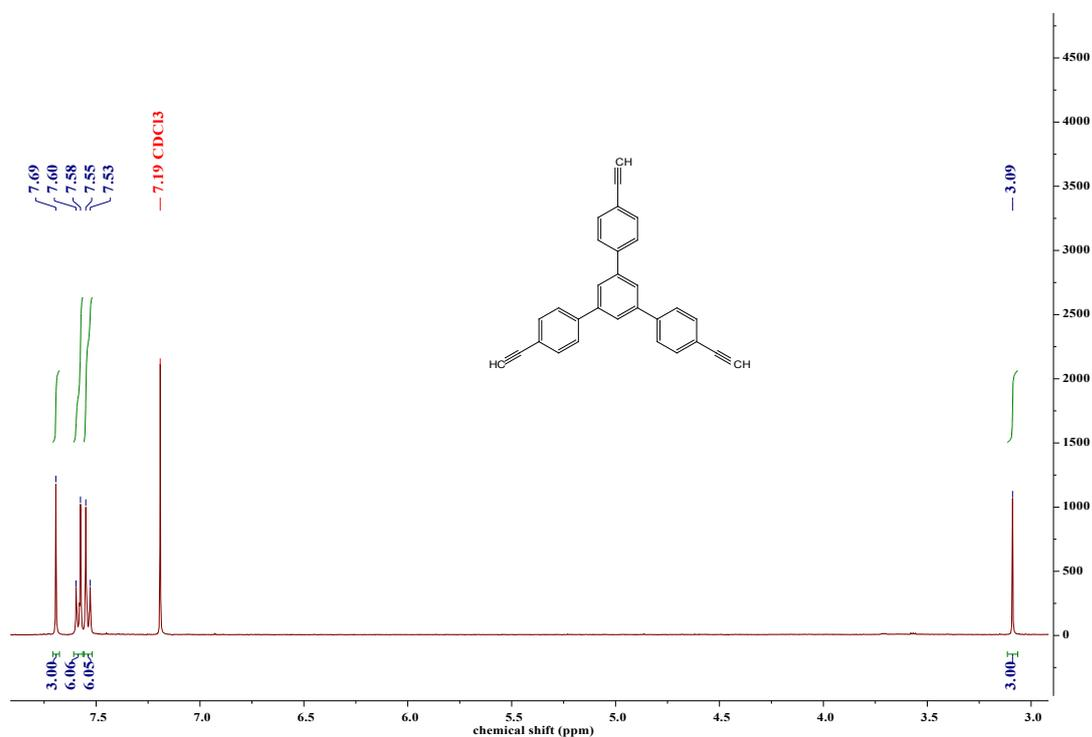
**Figure S5.**  $^1H$  NMR spectrum ( $CDCl_3$ , 400 MHz, rt) of TEB.
