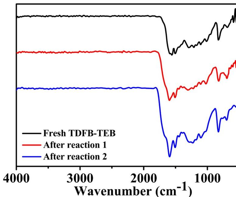
**Figure S15.** The FT-IR spectra of the fresh and recovered **TDFB-TEB**. (Reaction 1 is the oxidative amine coupling, reaction 2 is the sulfides oxidation.)
