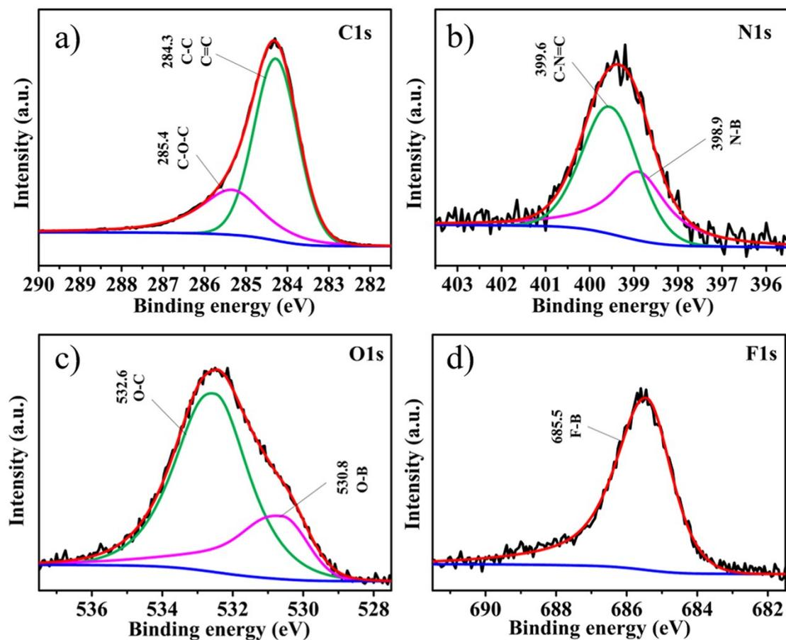
**Figure S6.** a) C 1s region XPS spectrum, b) N 1s region XPS spectrum, c) O 1s region XPS spectrum, and d) F 1s region XPS spectrum of **TDFB-TEB** before photocatalysis.
