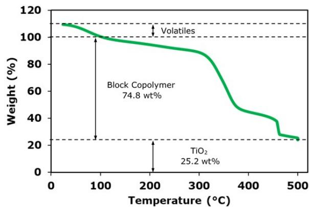
**Figure S2:** TGA data for the calcination of the polymer-TiO<sub>2</sub> composite material. Weight percentage is scaled to exclude volatiles. The mass loss at 450 °C is attributed to degradation of the remaining PDMS-MA stabiliser.
