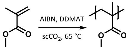
**Scheme S1:** Reaction scheme for synthesis of the PMMA macro-RAFT agent.
