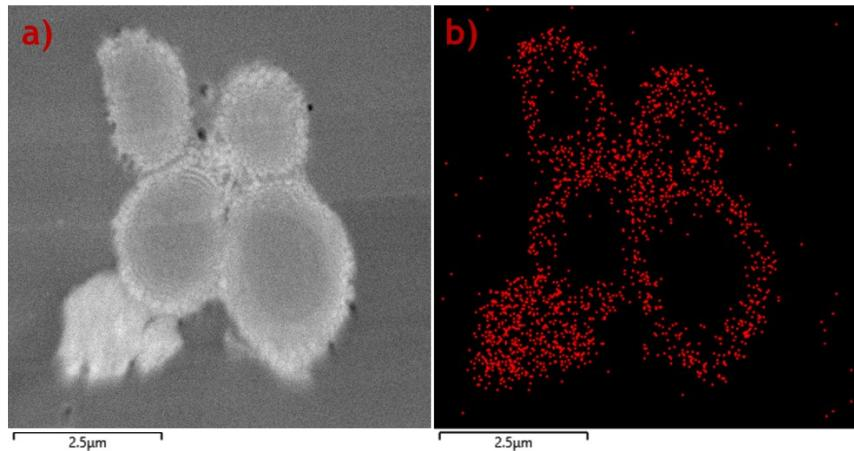
**Figure S1:** Elemental mapping of the polymer-TiO<sub>2</sub> composite material. (a) dark-field STEM micrograph and (b) corresponding elemental map with high concentration of elemental titanium highlighted as red pixels.
