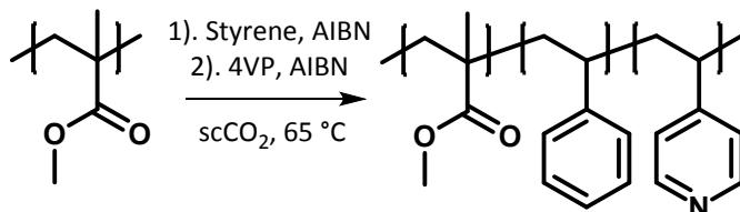
**Scheme S2:** Reaction scheme for synthesis of the ABC triblock copolymer.
