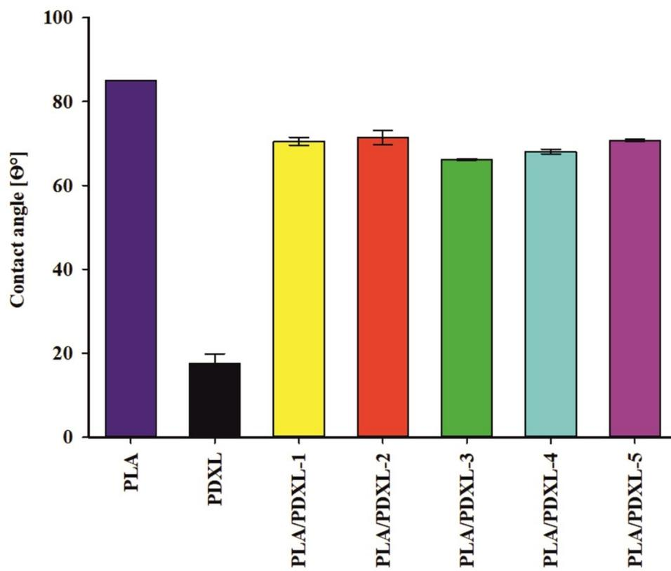
**Figure 6S.** Contact angles measured for of neat PLA and PDXL and PLA/PDXL copolymers with different content of comonomers (films on a glass plate with water as a reference liquid)
