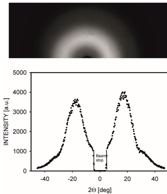
**Figure 5S.** Wide angle X-ray scattering (WAXS) analysis of sample containing 7% mol of DXL unit at PLA chain (PLA/PDXL-1)
