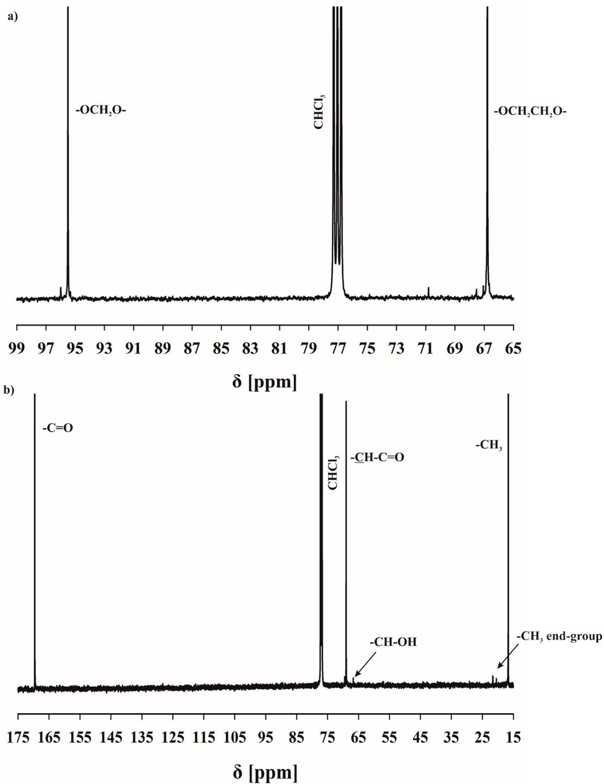
**Figure 3S.** <sup>13</sup>C NMR spectrum of a) DXL and b) LA homopolymer (500 MHz, CDCl<sub>3</sub>)
