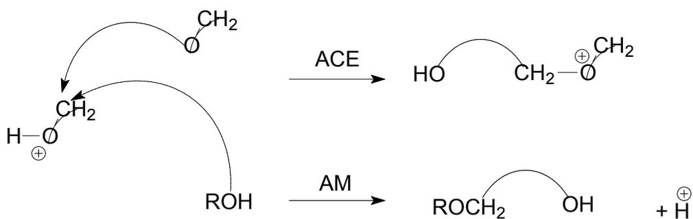
**Scheme 1.** Propagation according activated chain end (ACE) mechanism versus activated monomer (AM) mechanism in cationic polymerization of heterocyclic monomers. In order to enhance the contribution of AM, the instantaneous concentration of the non-protonated monomer should be kept as low as possible (monomer should be introduced slowly to the polymerization mixture).
