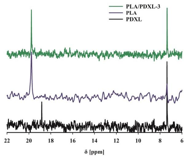
**Figure 4S.**  $^{29}\text{Si}$  NMR spectra of: green line: PLA homopolymer, blue line : PDXL homopolymer, black line: PLA/PDXL-3 copolymer.
