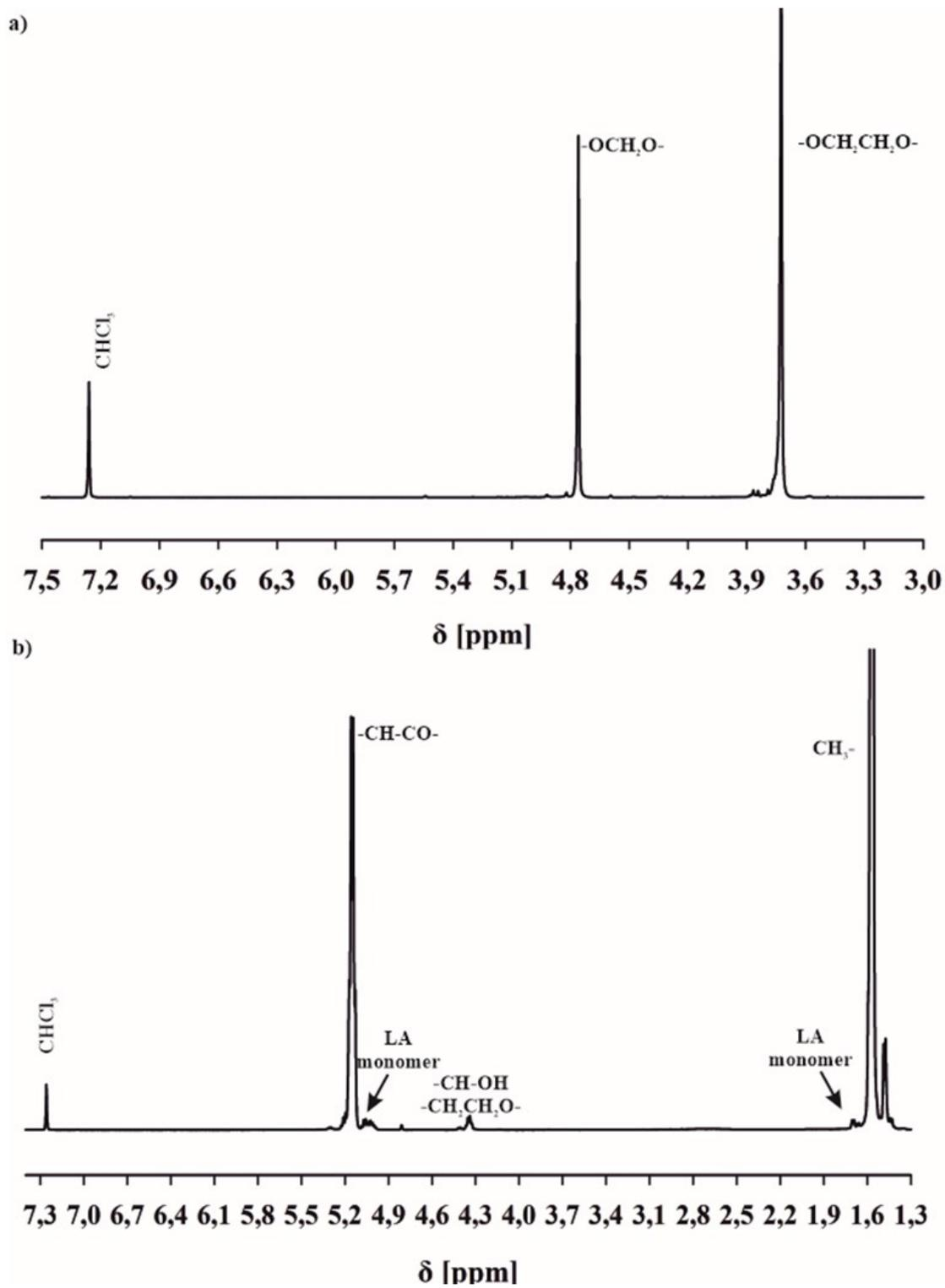
**Figure 2S.** <sup>1</sup>H NMR spectrum of a) DXL and b) LA homopolymer (500 MHz, CDCl<sub>3</sub>)
