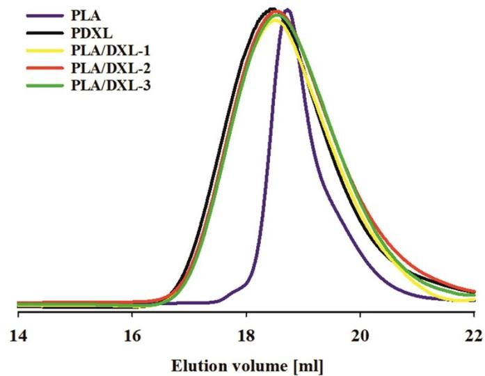
**Figure 1S.** Representative GPC traces of purified PLA, PDXL and PLA/PDXL copolymers
