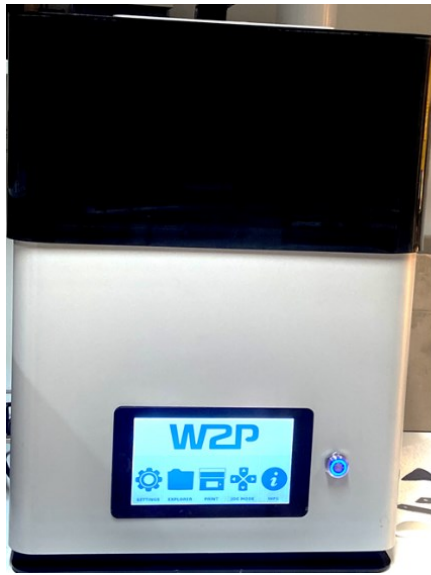
Figure S5 – Photograph of the dual-wavelength DLP 3D-printer prototype (with 405 and 365 nm light sources) from way2production and additional technical specifications of the prototype.
