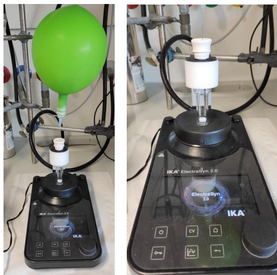
Figure S1. A fully commercial IKA ElectraSyn 2.0 setup involving an undivided cell was used for the electrochemically-initiated polymerization of reactive monomers.
