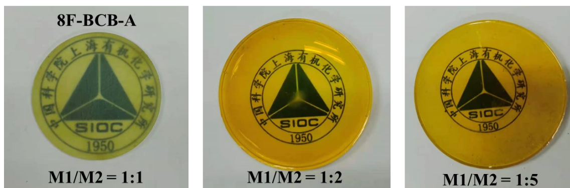
Figure S12. The images of cured resins in different molar ratios of M1 to M2 .
