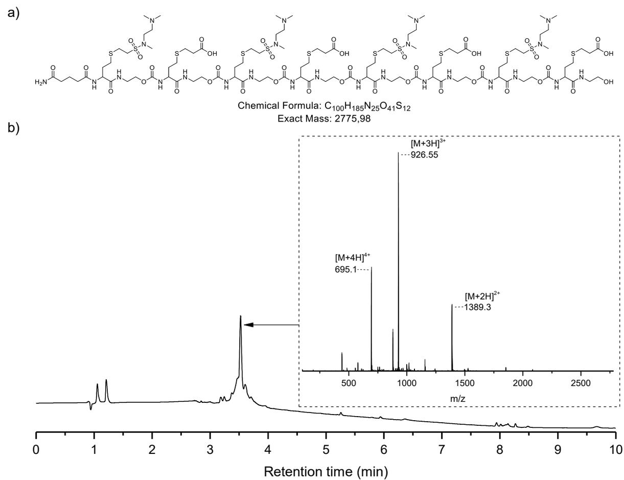
**Figure S9:** Octamer (*alt*)-CACACACA synthesised manually: a) molecular structure, b) LCMS analysis ( $\lambda = 214$  nm).
