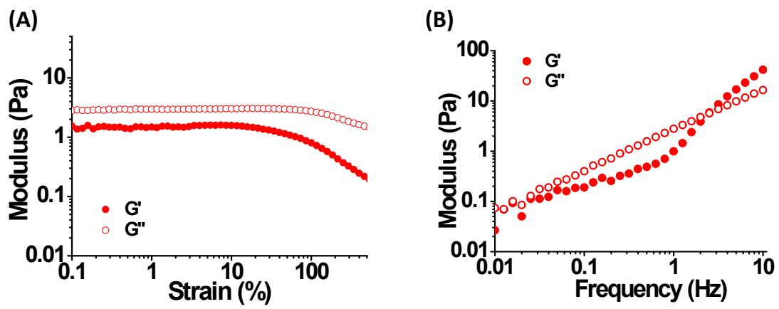
**Figure S6.** Strain-sweep (A) and frequency-sweep (B) rheology data for the concentrated MG-8MAA-1.0GMA. The frequency used in (A) is 1.0 Hz and the strain used in (B) is 1.0%. The MG concentration and pH were 14% and 7.4, respectively.
