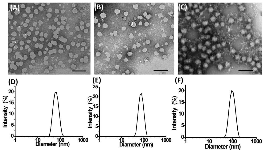
**Figure S3.** TEM images for (A) MG-8MAA-1.0GMA, (B) MG-16MAA-2.5GMA and (C) MG-32MAA-13GMA. DLS size distributions for (D) MG-8MAA-1.0GMA, (E) MG-16MAA-2.5GMA and (E) MG-32MAA-13GMA. The dispersion used in (D) - (F) had a pH 5.4 and the temperature was 60 °C.
