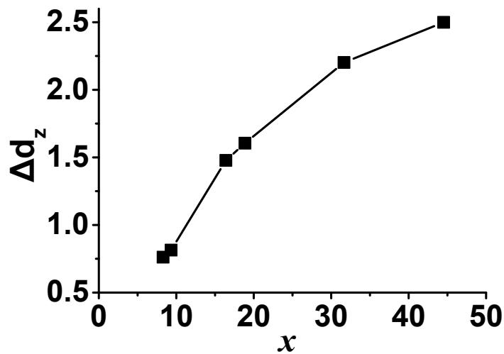
**Figure S4.** The change ratio of  $d_z$  ( $\Delta d_z$ ) vs. MAA content of all MGs.  $\Delta d_z = (d_{z \text{ (pH 7.4)}} - d_{z \text{ (pH 5.0)}}) / d_{z \text{ (pH 5.0)}}$ .
