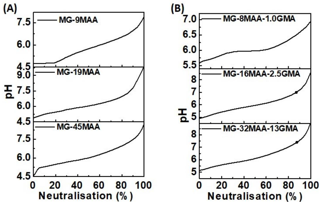
**Figure S1.** Potentiometric titration data for the MG- $x$ MAA and functionalised MG- $x$ MAA- $y$ GMA dispersions. The apparent  $pK_a$  values were obtained from the pH corresponding to 50% neutralisation.
