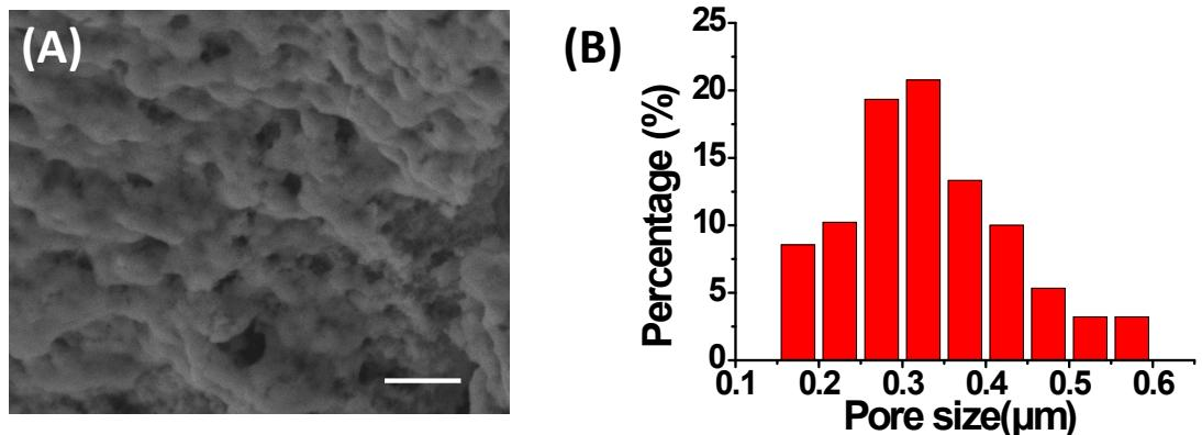
**Figure S9. (A)** SEM image of DX MG-32MAA-13GMA/Fe<sup>3+</sup>. The scale bar is 2 μm and the average pore size is 0.31 μm. **(B)** Pore size distribution for the gel.
