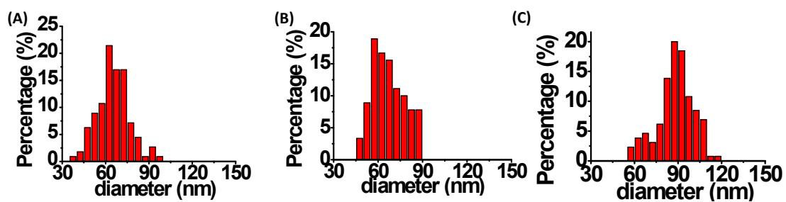
**Figure S2.** The size distributions of TEM for MG-9MAA **(A)**, MG-19MAA **(B)**, MG-45MAA **(C)**.
