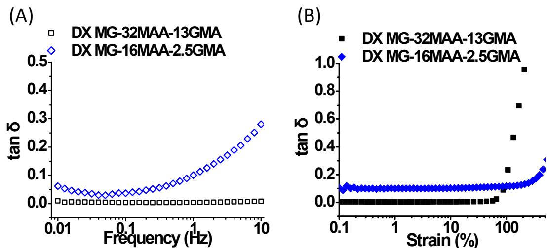
**Figure S8.**  $\tan \delta$  vs. frequency (A) and  $\tan \delta$  vs. strain (B) for DX MGs.  $\tan \delta = G''/G'$ . The strain used in (A) is 1.0% and the frequency used in (B) is 1.0 Hz.
