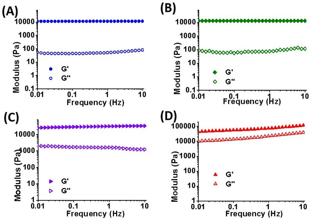
**Figure S10.** Frequency-sweep rheology data for the DX MG-32MAA-13GMA immersed into ionic solution of (A) NaCl, (B) MgCl<sub>2</sub>, (C) AlCl<sub>3</sub>, (D) FeCl<sub>3</sub>. The strain used for all figure is 1.0%
