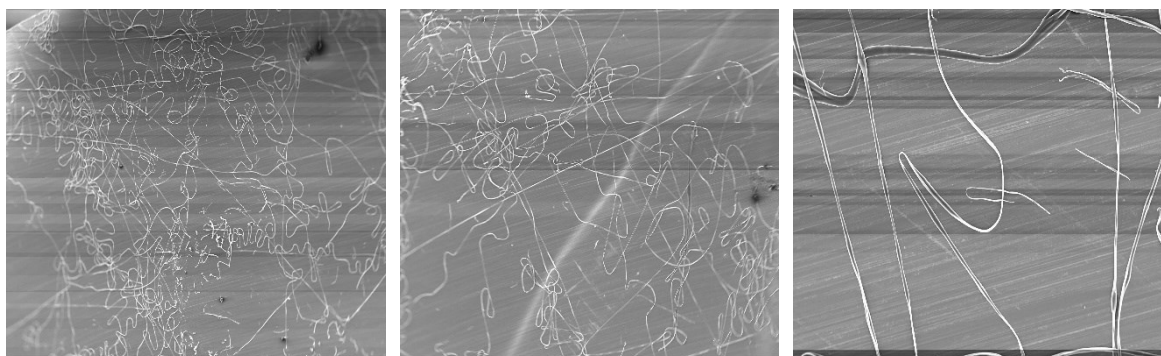
Figure S22: SEM image of the morphology of electrospun SPU 1. Planar Electrode; Working Distance 25 cms, Working Voltage 12 kV, Temperature room-box 28.9 °C, Syringe 31.2 °C Relative Humidity 34 %, Mean Feature Regular fibres 18.5 \mu\text{m} ., Polymer Concentration 20 % in dichloromethane. Motor Voltage 3.8 V, Needle Size 22G \times \frac{1}{2} .
