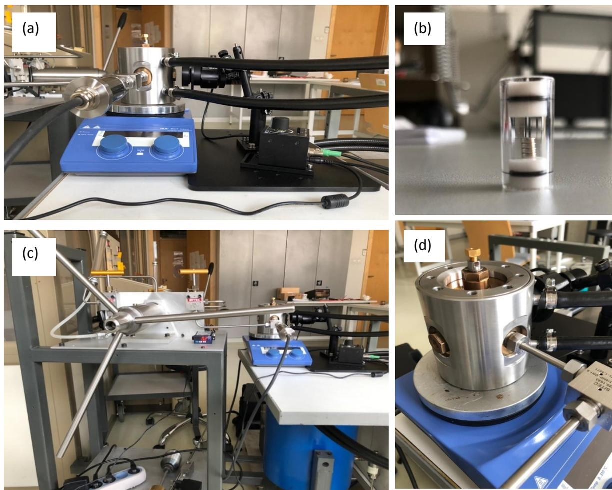
Fig S1. High-pressure equipment, (a) optical pressure chamber and light source, (b) quartz ampule with a stirrer, (c) pressure generator, pressure chamber and light source, (d) optical pressure chamber with Sapphire windows
