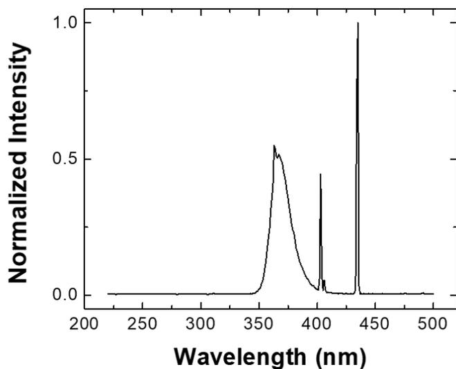
**Figure S 12.** Normalized emission spectrum of the UV light source (UV nail gel-curing lamp).
