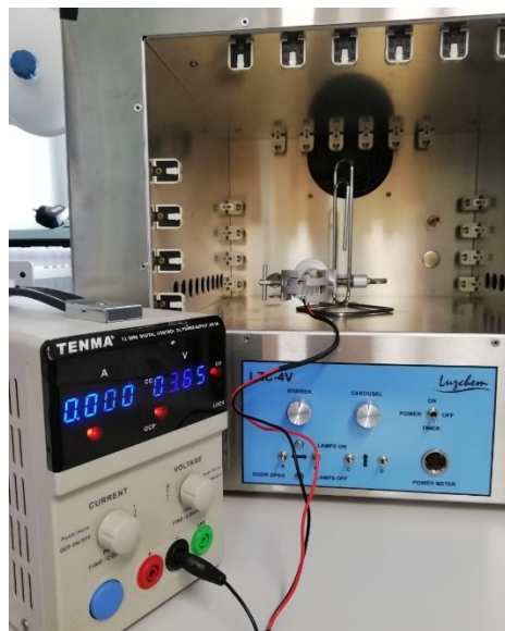
Figure S21: Experimental setup for irradiation with LED ( \lambda = 365 \text{ nm} ) with variable power source in photoreactor.
