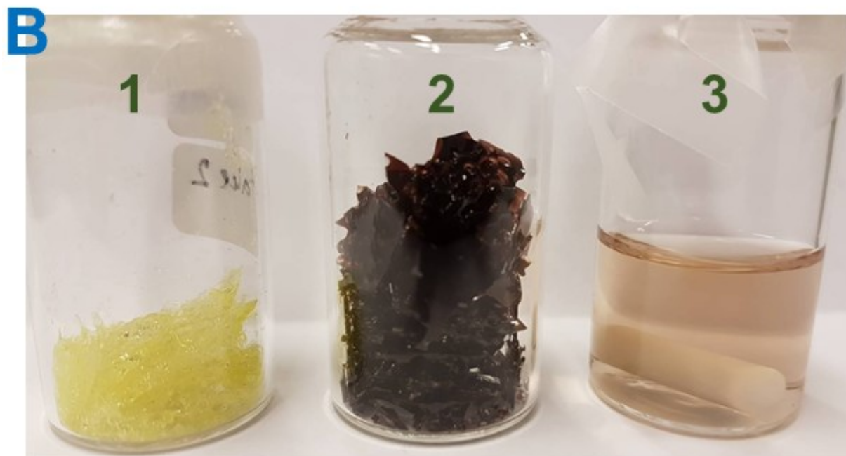
Figure S6. A: comparison of NMR spectra of the product of polymerization of non-neutralized H-AMPS in DMSO before and after oven drying at 80 °C. The appearance of new peaks after drying may be a sign of decomposition B: Appearance of PAMPS-RAFT macroCTA synthesized by the method involving Et 3 N ( B1 ), and by polymerizing H-AMPS acid in DMSO ( B2 ). The change in color from yellow to dark red/brown was a consequence of drying the polymer in an oven. Et 3 N-AMPS polymer was processed in the same way and did not change its appearance. The discolored product is soluble in water ( B3 ), the solution being characterized by a foul smell.
