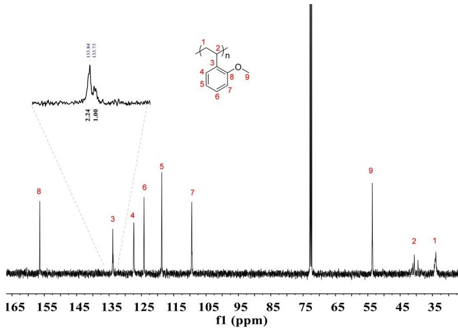
**Figure S20.**  $^{13}\text{C}$  NMR spectrum of poly(*o*MOS) (entry 2, Table 2) (100 MHz,  $\text{C}_2\text{D}_2\text{Cl}_4$ , 100 °C)
