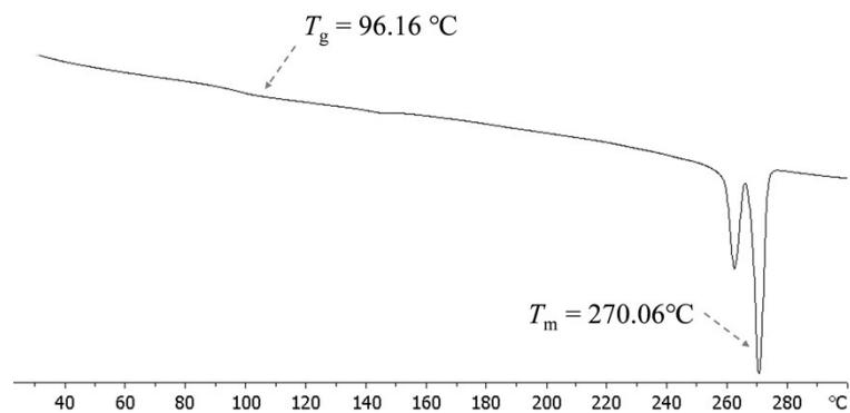
**Figure S44.** DSC curve of polystyrene (entry 1, Table 2)
