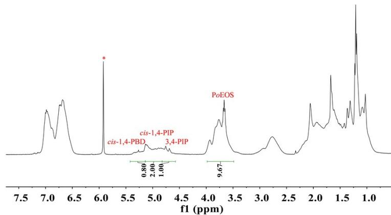
**Figure S5.** <sup>1</sup>H NMR spectrum of poly(*o*EOS-IP-BD) (entry 8, Table 1) (400 MHz, C<sub>2</sub>D<sub>2</sub>Cl<sub>4</sub>, 100 °C)
