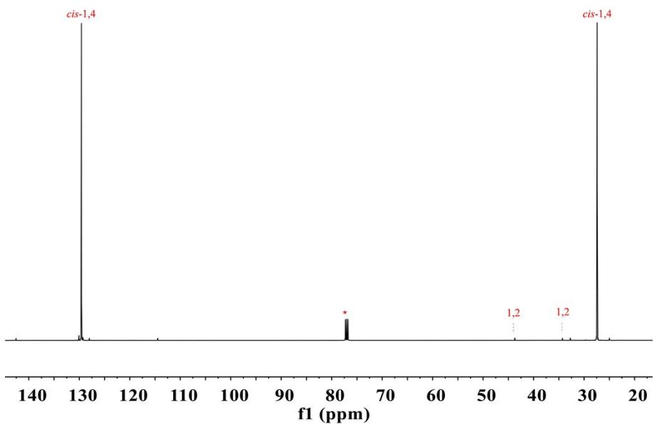
**Figure S23.**  $^{13}\text{C}$  NMR spectrum of PBD (500 MHz,  $\text{CDCl}_3$ , 25 °C)
