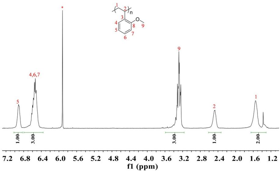
**Figure S7.** <sup>1</sup>H NMR spectrum of poly(*o*MOS) (entry 2, Table 2) (400 MHz, C<sub>2</sub>D<sub>2</sub>Cl<sub>4</sub>, 100 °C)
