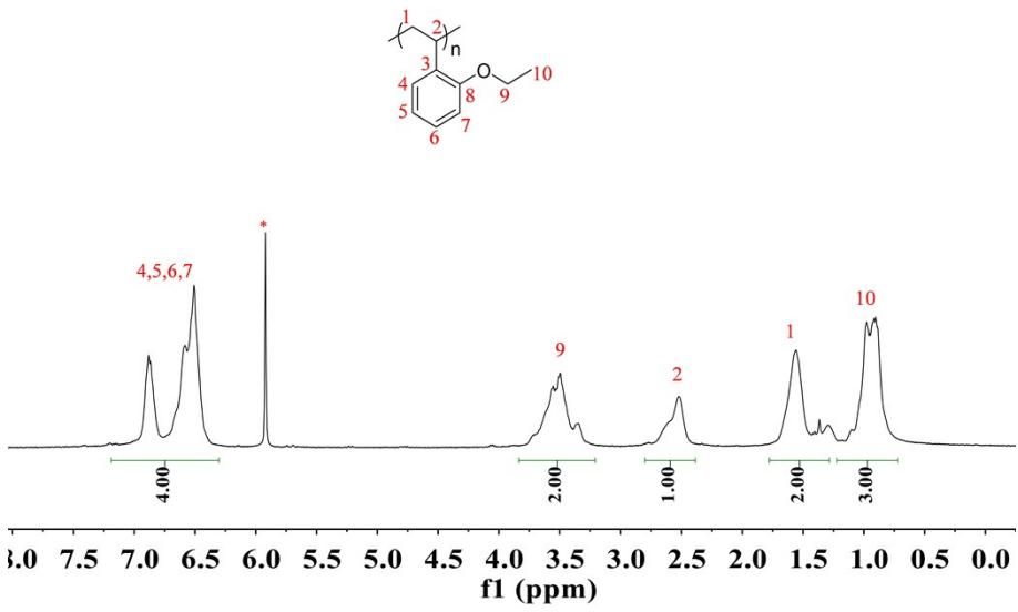
**Figure S8.** <sup>1</sup>H NMR spectrum of poly(*o*EOS) (entry 5, Table 2) (400 MHz, C<sub>2</sub>D<sub>2</sub>Cl<sub>4</sub>, 100 °C)
