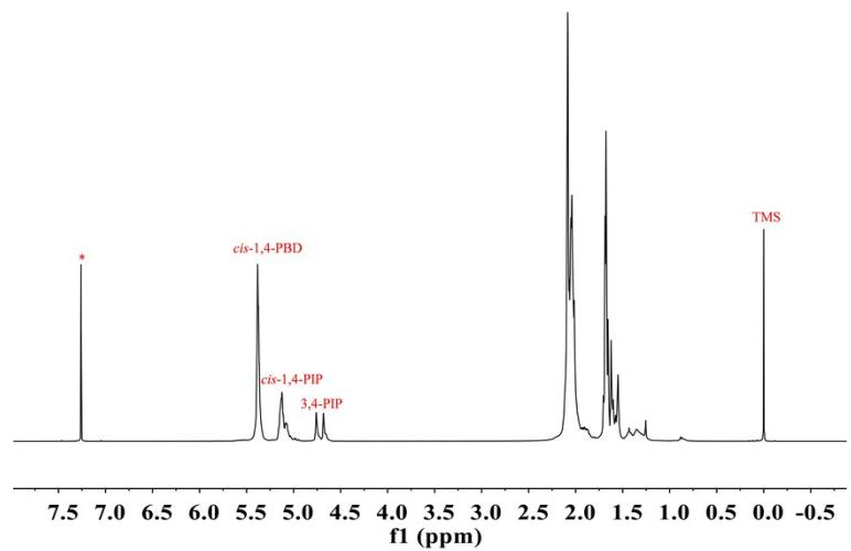
**Figure S12.** <sup>1</sup>H NMR spectrum of poly(BD-IP) (500 MHz, CDCl<sub>3</sub>, 25 °C)
