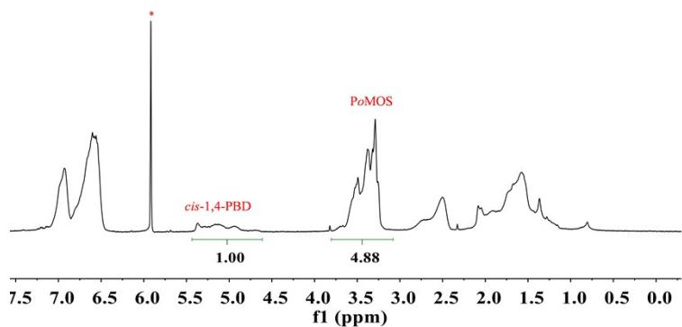
**Figure S6.** <sup>1</sup>H NMR spectrum of poly(*o*MOS-IP-BD) isolated in 1 min (400 MHz, C<sub>2</sub>D<sub>2</sub>Cl<sub>4</sub>, 100 °C)
