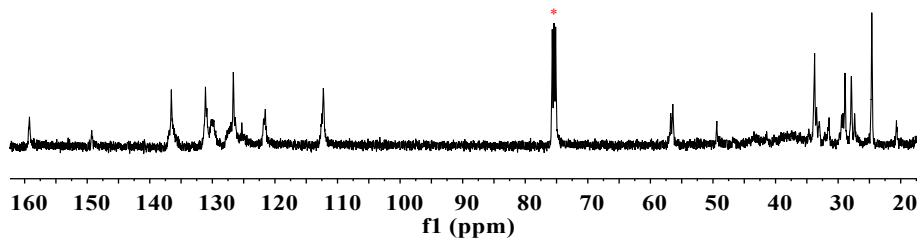
**Figure S13.** <sup>13</sup>C NMR spectrum of poly(*o*MOS-IP-BD) (entry 2, Table 1) (100 MHz, C<sub>2</sub>D<sub>2</sub>Cl<sub>4</sub>, 100 °C)
