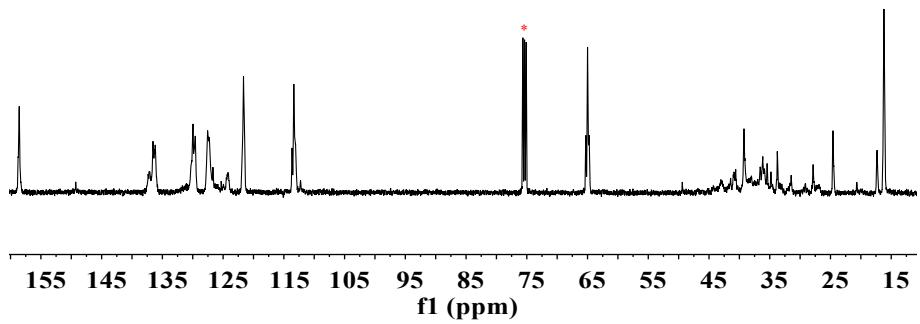
**Figure S17.** <sup>13</sup>C NMR spectrum of poly(*o*EOS-IP-BD) (entry 8, Table 1) (100 MHz, C<sub>2</sub>D<sub>2</sub>Cl<sub>4</sub>, 100 °C)
