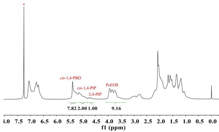
**Figure S9.** <sup>1</sup>H NMR spectrum of poly(*o*EOS-IP-BD) for uniaxial extension experiments (500 MHz, CDCl<sub>3</sub>, 25 °C)
