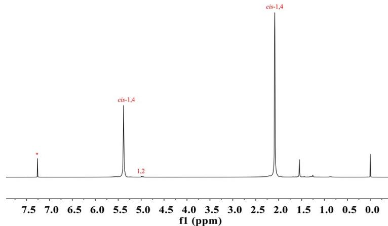
**Figure S10.** <sup>1</sup>H NMR spectrum of PBD (500 MHz, CDCl<sub>3</sub>, 25 °C)
