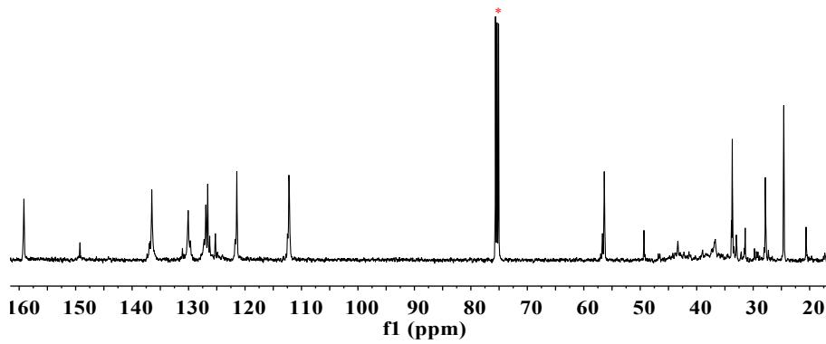
**Figure S15.** <sup>13</sup>C NMR spectrum of poly(*o*MOS-IP-BD) (entry 5, Table 1) (100 MHz, C<sub>2</sub>D<sub>2</sub>Cl<sub>4</sub>, 100 °C)
