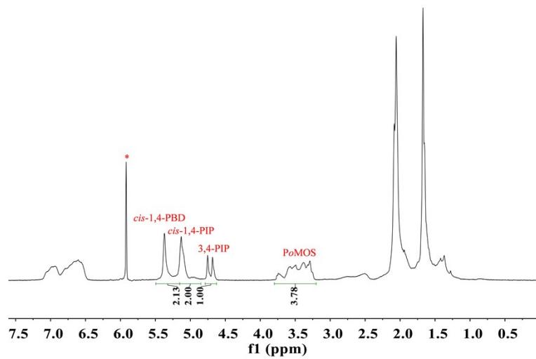
**Figure S1.** <sup>1</sup>H NMR spectrum of poly(*o*MOS-IP-BD) (entry 2, Table 1) (400 MHz,  $\text{C}_2\text{D}_2\text{Cl}_4$ , 100 °C)
