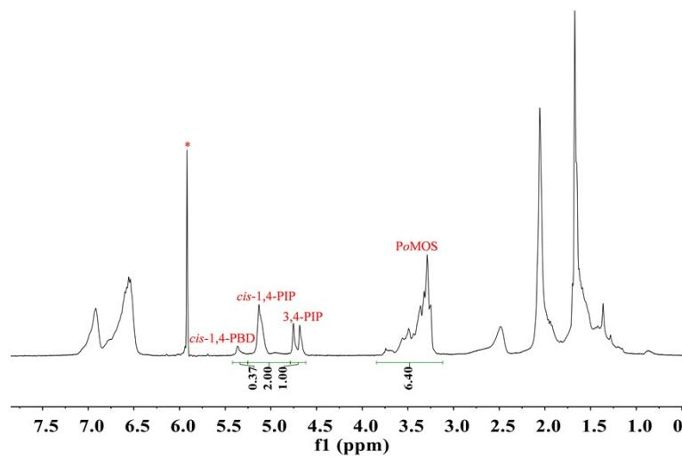
**Figure S3.** <sup>1</sup>H NMR spectrum of poly(*o*MOS-IP-BD) (entry 5, Table 1) (400 MHz,  $\text{C}_2\text{D}_2\text{Cl}_4$ , 100 °C)
