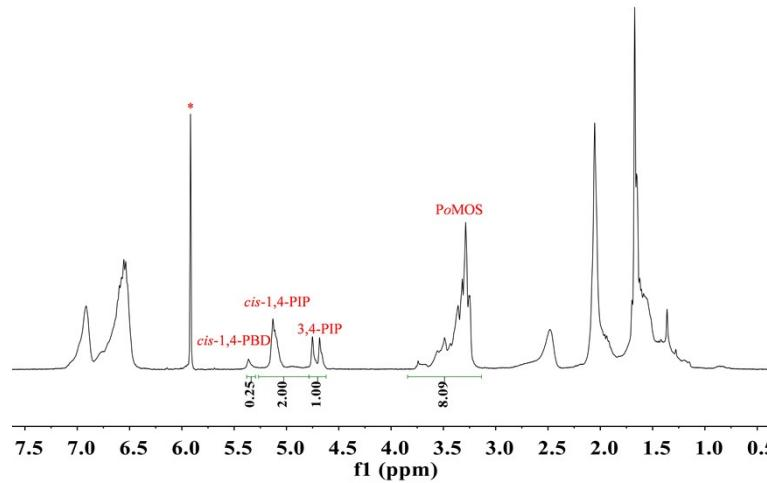
**Figure S4.** <sup>1</sup>H NMR spectrum of poly(*o*MOS-IP-BD) (entry 6, Table 1) (400 MHz,  $\text{C}_2\text{D}_2\text{Cl}_4$ , 100 °C)
