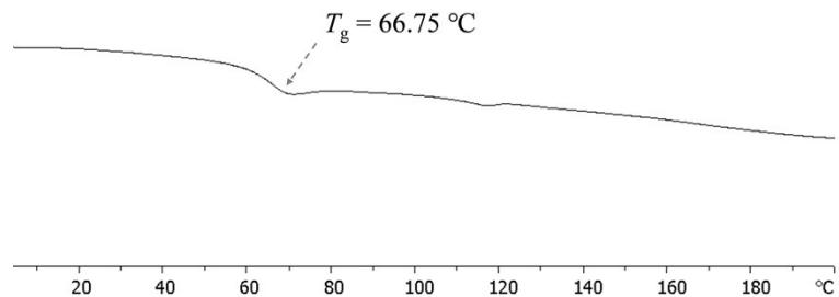
**Figure S43.** DSC curve of poly(*o*MOS-IP-BD) isolated in 1 min (entry 1, Table S1)
