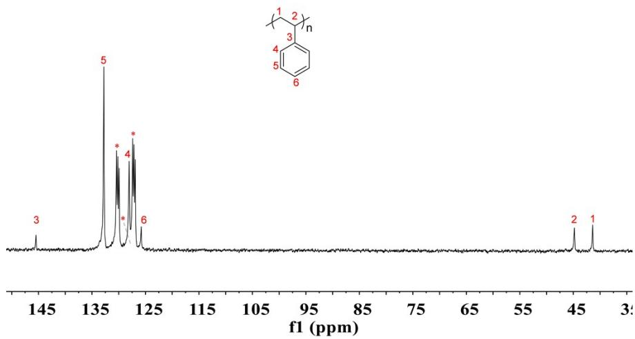
**Figure S19.**  $^{13}\text{C}$  NMR spectrum of polystyrene (entry 1, Table 2) (100 MHz,  $\text{C}_6\text{D}_4\text{Cl}_2$ , 100 °C)
