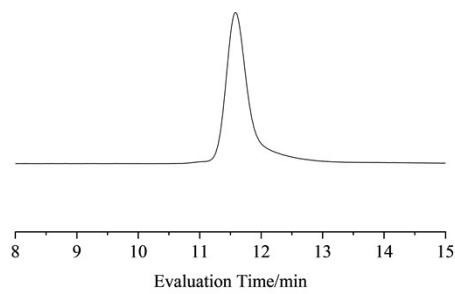
**Figure S34.** GPC curve of poly(*o*MOS-IP-BD) isolated in 1 min (entry 1, Table S1)
