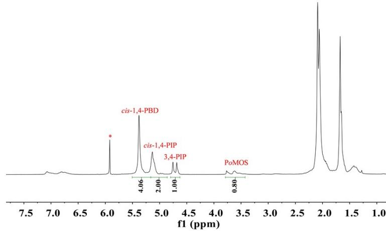
**Figure S2.** <sup>1</sup>H NMR spectrum of poly(*o*MOS-IP-BD) (entry 4, Table 1) (400 MHz,  $\text{C}_2\text{D}_2\text{Cl}_4$ , 100 °C)
