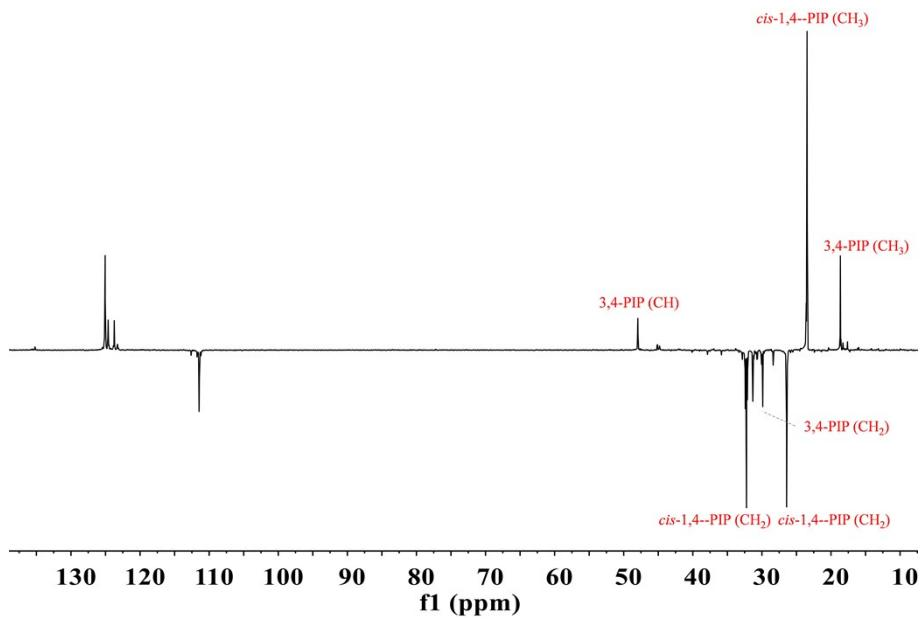
**Figure S25.** DEPT 135 spectrum of PIP (500 MHz, CDCl<sub>3</sub>, 25 °C)
