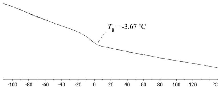
**Figure S48.** DSC curve of poly(*o*EOS-IP-BD) for uniaxial extension experiments
