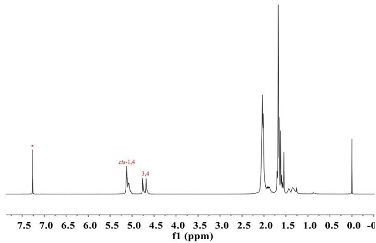
**Figure S11.** <sup>1</sup>H NMR spectrum of PIP (500 MHz, CDCl<sub>3</sub>, 25 °C)
