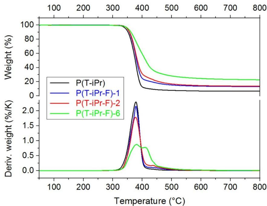
Figure ESI 35. TGA curves of the terpolyesters of series P(T-iPr-F).
