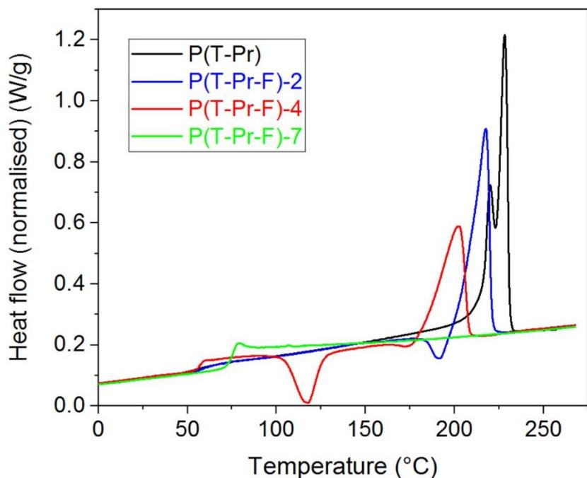
Figure ESI 29. DSC curves (2nd heating) of the terpolyesters of the P(T-Pr-F) series.
