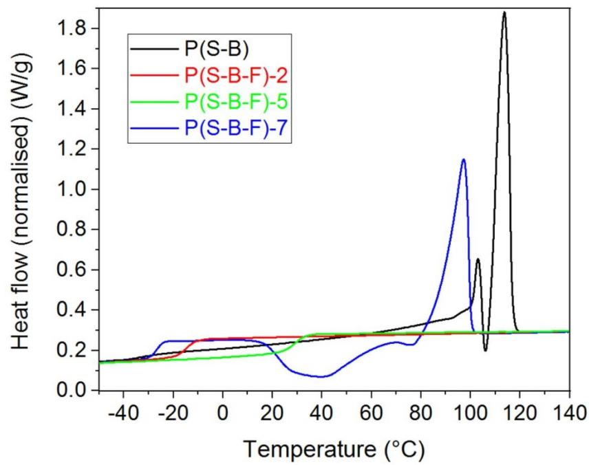
Figure ESI 32. DSC curves (2nd heating) of the terpolyesters of the P(S-B-F) series.
