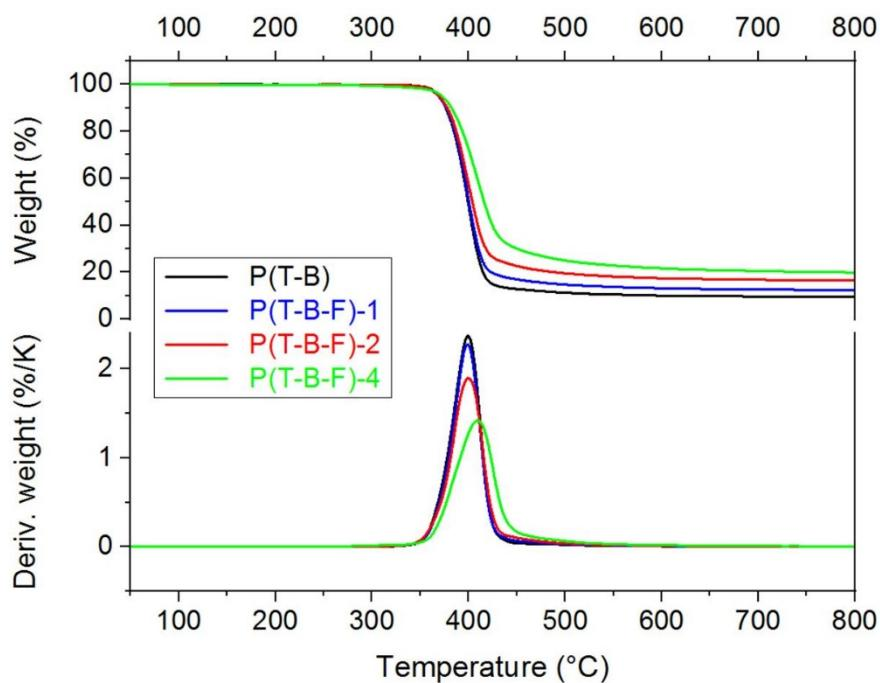
Figure ESI 36. TGA curves of the terpolyesters of series P(T-B-F).
