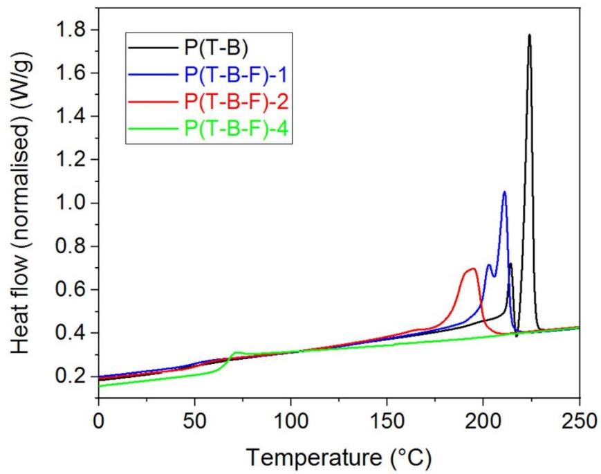
Figure ESI 31. DSC curves (2nd heating) of the terpolyesters of the P(T-B-F) series.
