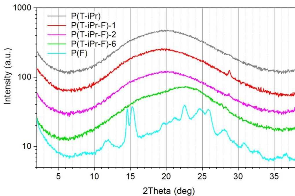
Figure ESI 27. WAXS curves of copolymers of the series  $P(T\text{-}iPr\text{-}F)$ .
