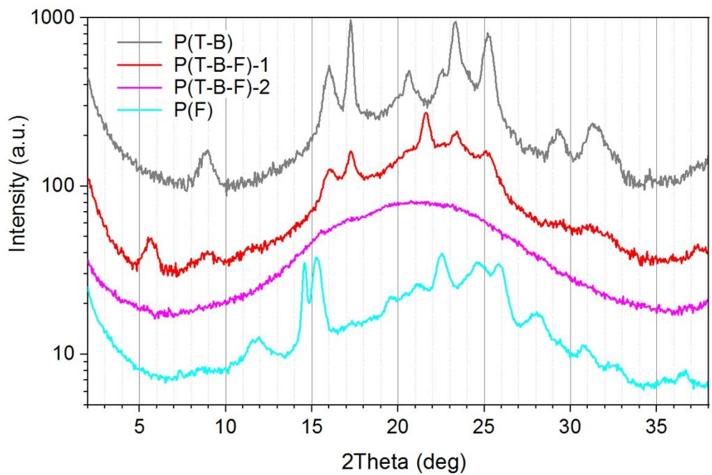
Figure ESI 28. WAXS curves of copolymers of the series P(T-B-F).
