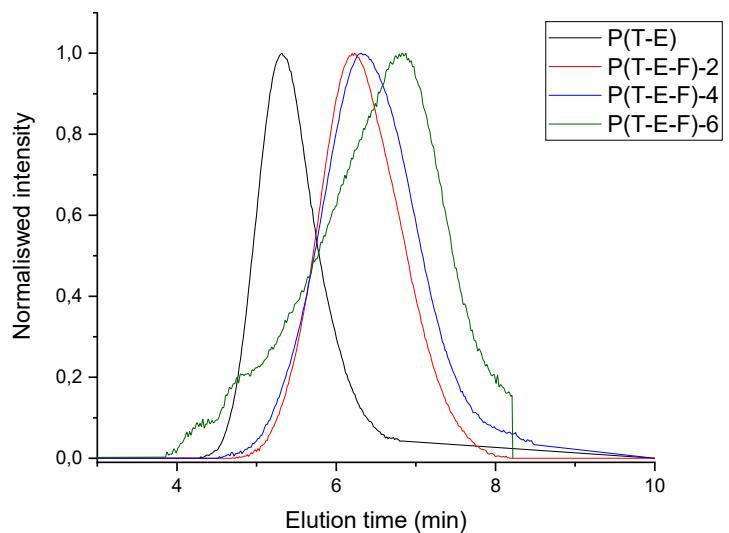
Figure ESI 21. SEC elution curves of the copolymers of the P(T-E-F) series.
