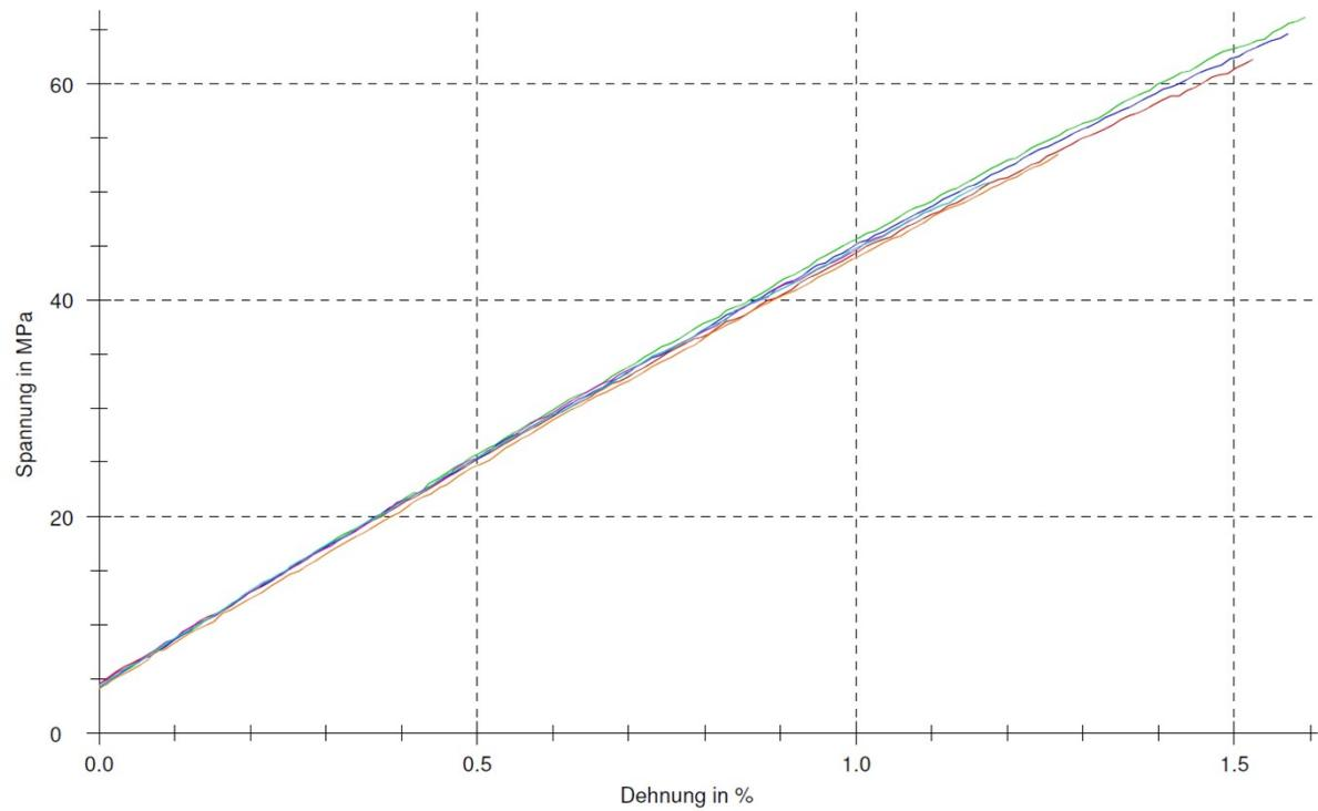
Figure ESI 42. Stress-strain curves of P(T-E-F)-2 fibres, EB treated (600 kGy).
