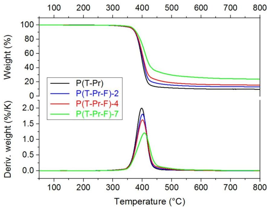
Figure ESI 34. TGA curves of the terpolyesters of series P(T-Pr-F).
