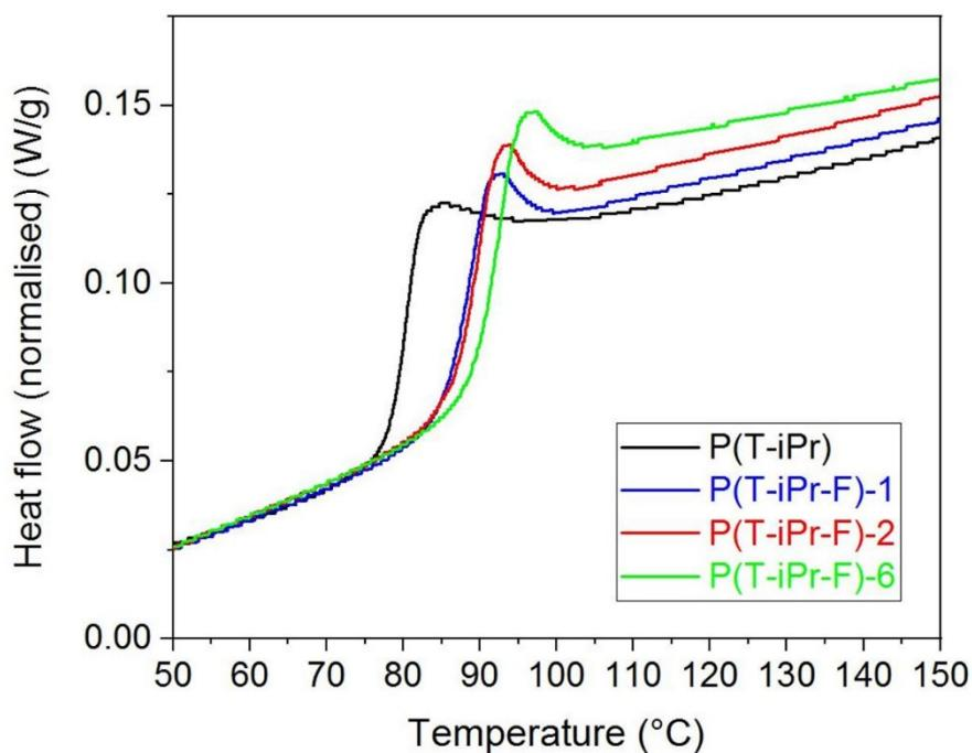
Figure ESI 30. DSC curves (2nd heating) of the terpolyesters of the P(T-iPr-F) series.
