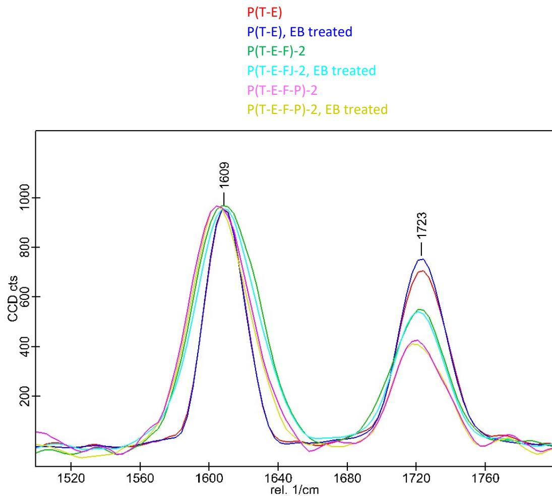
Figure ESI 40. Raman spectra (1500 – 1800 cm<sup>-1</sup>) of terpolyesters of the P(T-E-F) series before and after EB treatment
