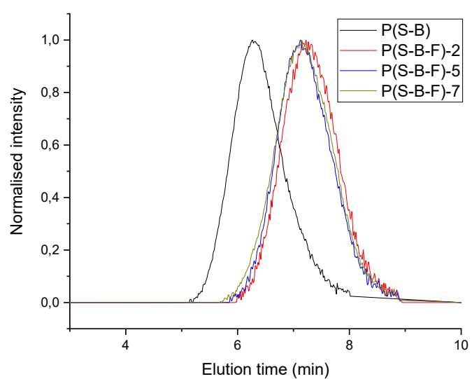
Figure ESI 25. SEC elution curves of the copolymers of the P(S-B-F) series
