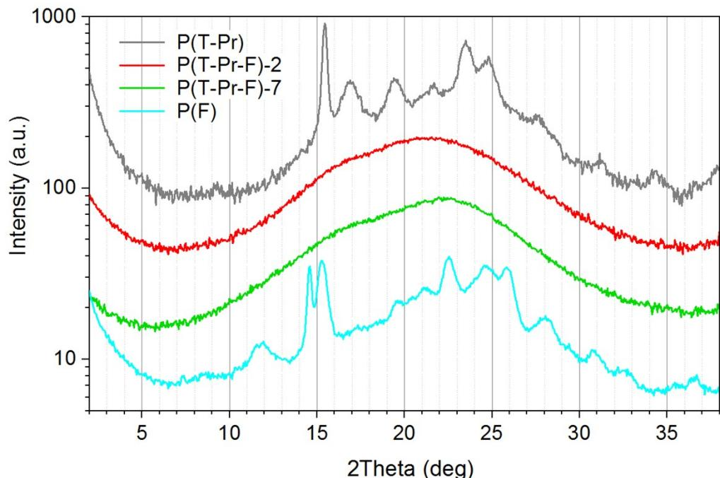
Figure ESI 26. WAXS curves of copolymers of the  $P(T\text{-}Pr\text{-}F)$  series.
