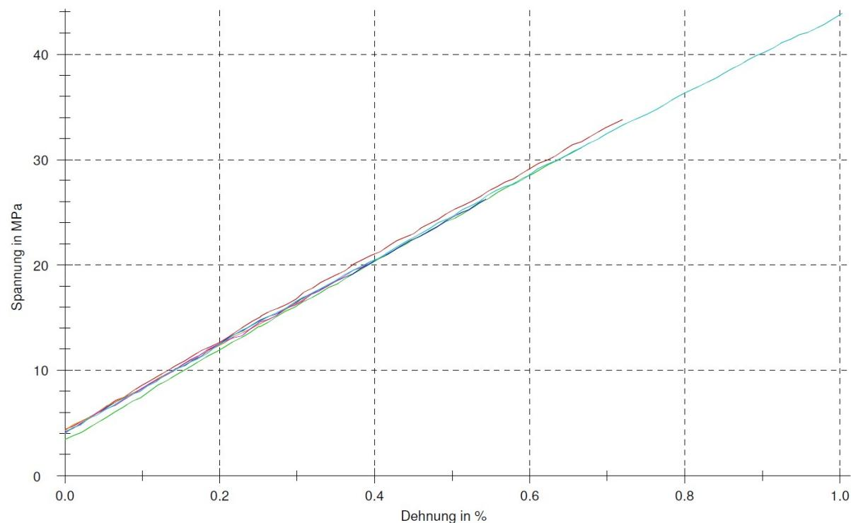
Figure ESI 41. Stress-strain curves of P(T-E-F)-2 fibres, as-spun.
