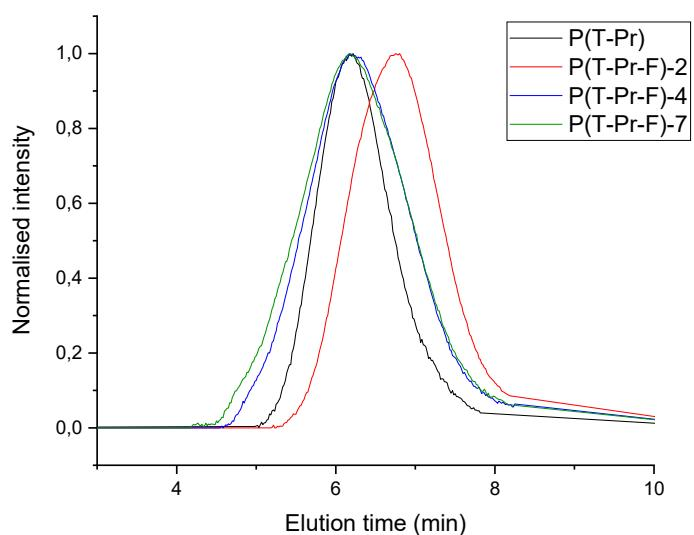
Figure ESI 22. SEC elution curves of the copolymers of the P(T-Pr-F) series.
