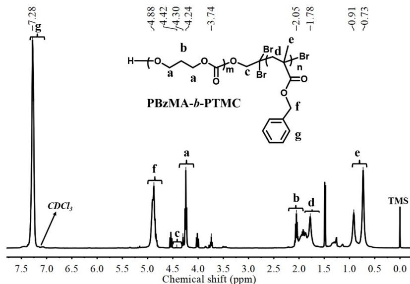
Figure S9 <sup>1</sup>H NMR spectrum of block copolymer PBzMA-*b*-PTMC was synthesized via “one-pot, one step” (entry 5, Table 2).
