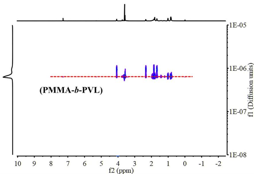
Figure S5  $^1\text{H}$  DOSY NMR spectrum of the block copolymer PMMA-*b*-PVL was synthesized via “one-pot, one step” (entry 4, Table 2).
