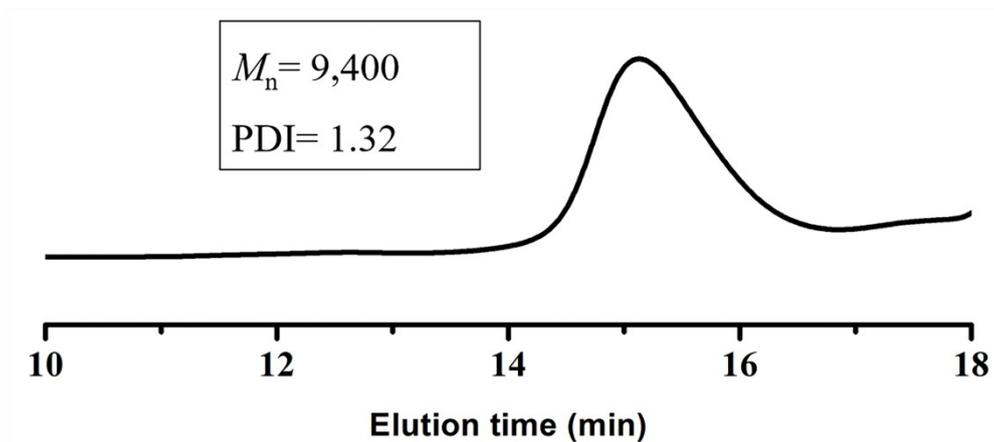
Figure S7 GPC trace of block copolymer PBzA-*b*-PTMC was synthesized via “one-pot, one step” (entry 5, Table 2).
