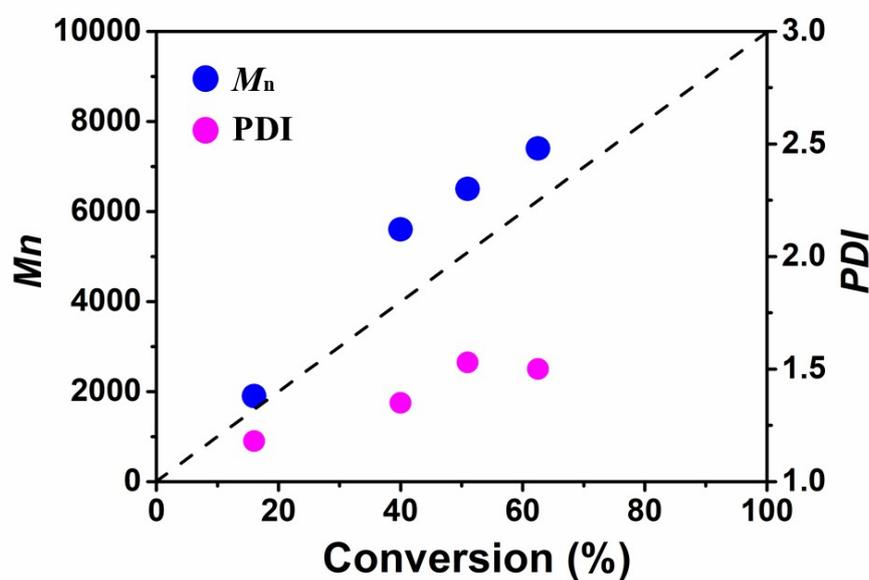
Figure S6 The number-average molecular weight ( $M_{n,\text{GPC}}$ ) and PDI versus monomer conversion of block copolymer PMMA-*b*-PVL.
