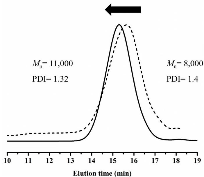
Figure S3 GPC traces of PMMA and block copolymer PMMA-*b*-PTMC (entry 2, Table 1).
