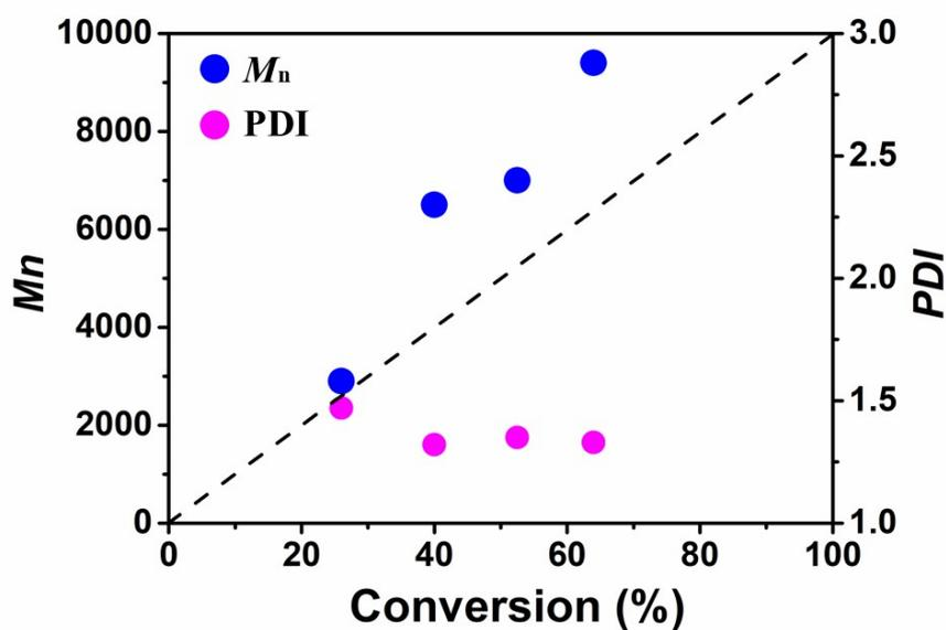
Figure S4 The number-average molecular weight ( $M_{n, \text{GPC}}$ ) and PDI versus monomer conversion of block copolymer PMMA-*b*-PTMC.
