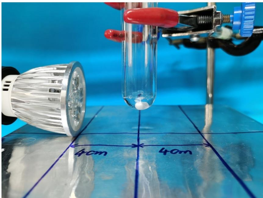
Figure S1 the picture of LED-light (the distance between the LED and the Schlenk tube is 4 centimeters).
