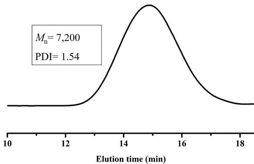
Figure S8 GPC trace of block copolymer PBzMA-*b*-PVL was synthesized via “one-pot, one step” (entry 6, Table 2).
