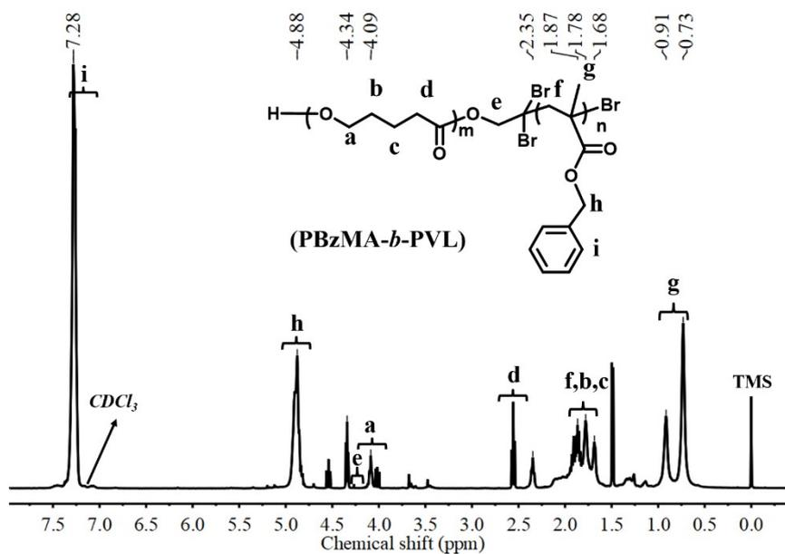
Figure S10 <sup>1</sup>H NMR spectrum of block copolymer PBzMA-*b*-PVL was synthesized via “one-pot, one step” (entry 6, Table 2).
