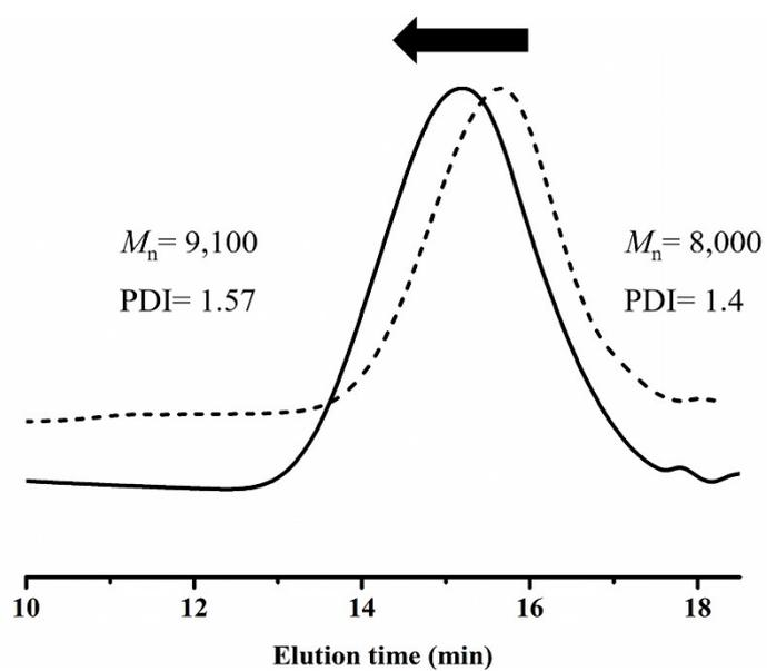
Figure S2 GPC traces of PMMA and block copolymer PMMA-*b*-PTMC (entry 1, Table 1).
