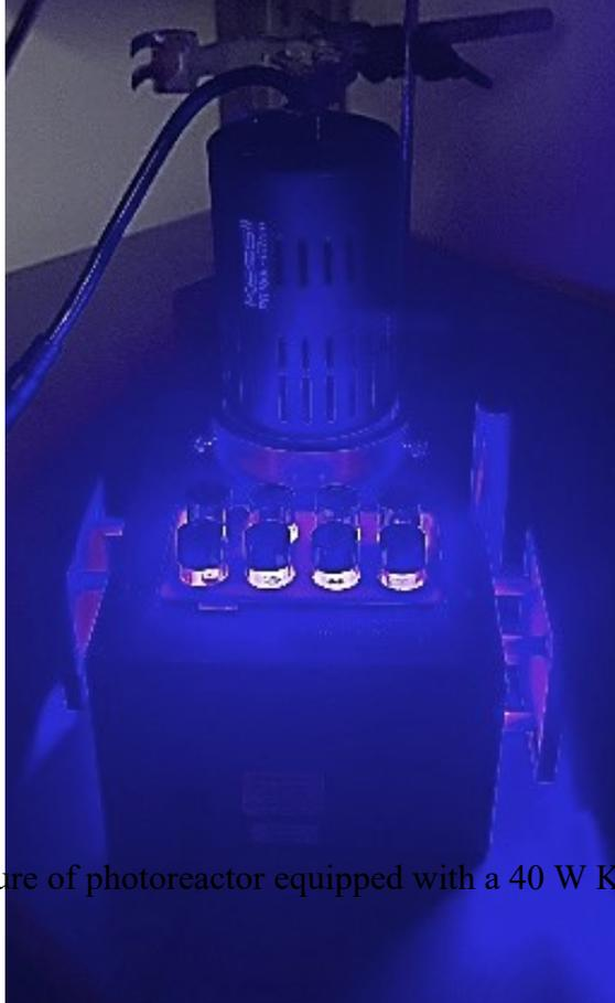
**Figure S9.** Picture of photoreactor equipped with a 40 W Kessil lamp.
