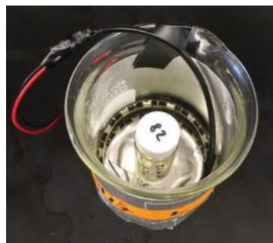
Figure S1. 400 mL white light LED beaker photoreactor for polymerizations.
