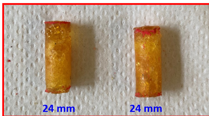
Figure S8. DoC of poly(TMPTA) with CTC 3 (2% wt) can reach 24 mm for 1.5 min (left) and 3 min (right) under 405 nm @LED irradiation.
