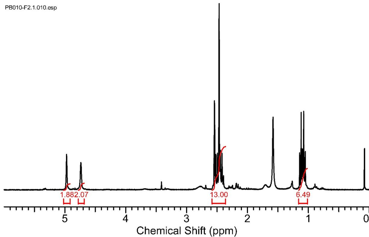
Figure ESI 3: <sup>1</sup>H-NMR spectrum of the BODIPY-diol compound (**3**) in CDCl<sub>3</sub>.
