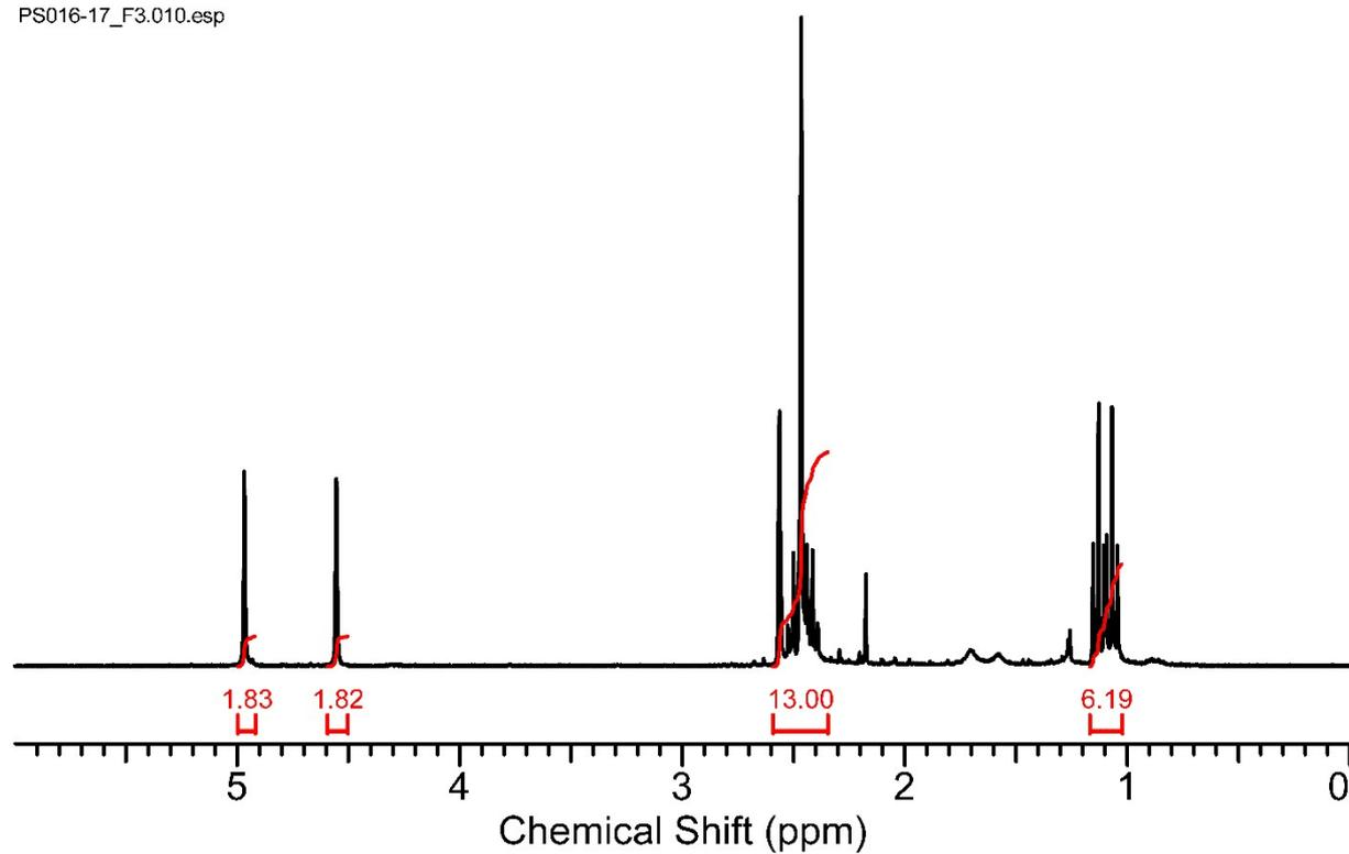
Figure ESI 5:  $^1\text{H}$ -NMR spectrum of BODIPY-azide compound (4) in  $\text{CDCl}_3$ .
