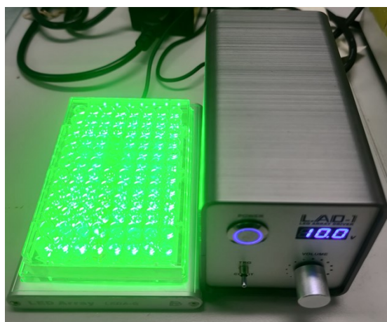
Figure S2. Digital image of the HT-PET RAFT wellplate polymerization setup.
