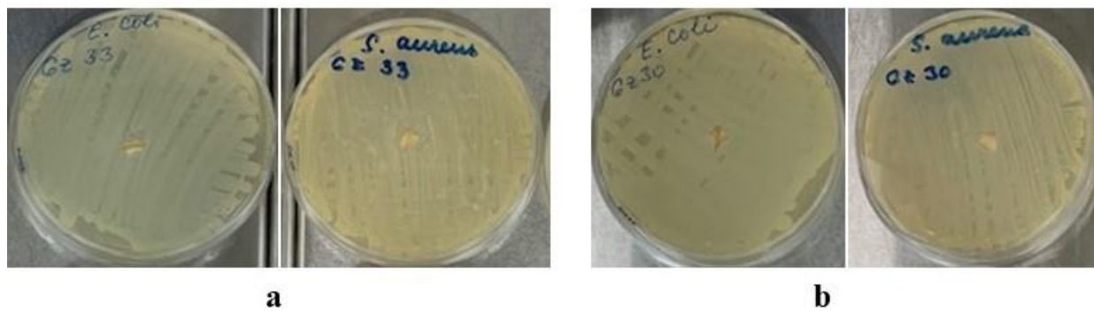
Figure S5. Antibacterial activity of small pieces of modified fabrics Cg19Q69 and Cg51Q100 against E. coli (a) and S. aureus (b) respectively, tested by Disk-diffusion Assay method for 24 hours at 37°C.
