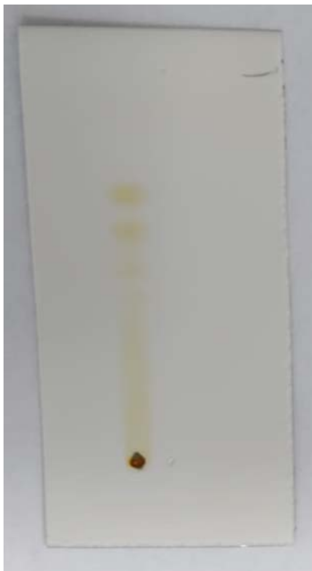
Fig. S8. TLC analysis using pentane:Et 2 O (20:1 v/v) as eluent for the reaction of p6-DT 20 (2.8 mM) with DTT (6.1 mM; 1.1 equiv. w.r.t. end-caps) and DBU (22 mM; 4.0 equiv. w.r.t. end-caps). Iodine dip was used to visualize spots. Top spot was isolated by preparative TLC (using the same eluent) and identified as 1,2,9,10-tetrathiacyclohexadecane on the basis of 1 H NMR and 13 C NMR.
