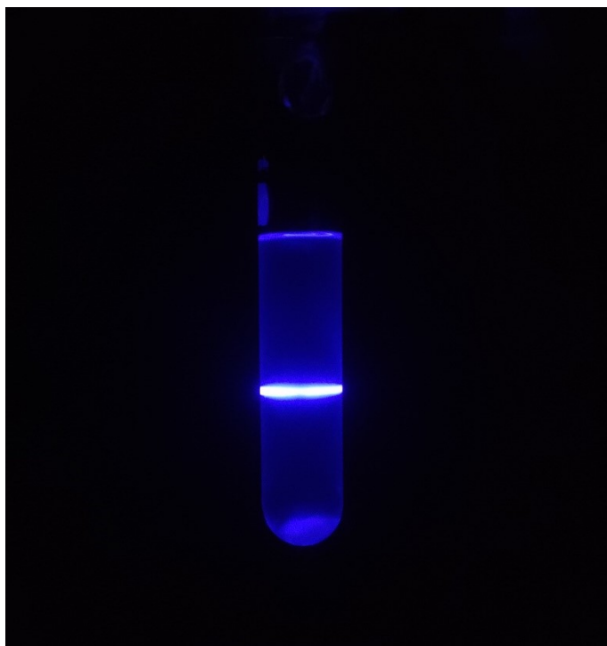
Fig S2. Blue fluorescence emitted from UCNPs under 980 nm NIR irradiation
