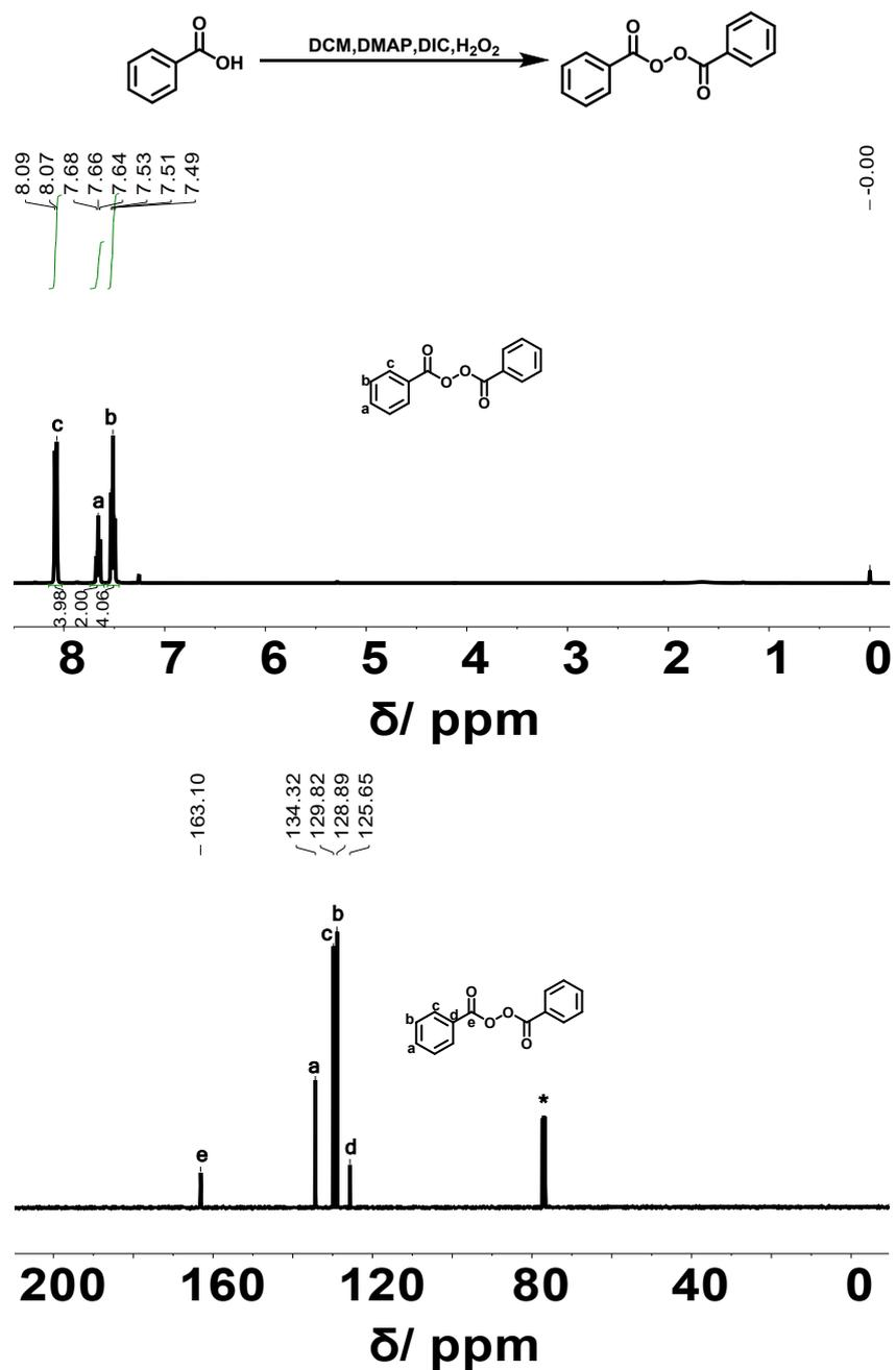
**Figure S1.** The strategy of converting benzoic acid to benzoyl peroxide and the  $^1\text{H}$  (400 MHz) NMR and  $^{13}\text{C}$  (100 MHz) NMR spectrum of benzoyl peroxide in  $\text{CDCl}_3$ . The solvent peaks are marked with asterisks.
