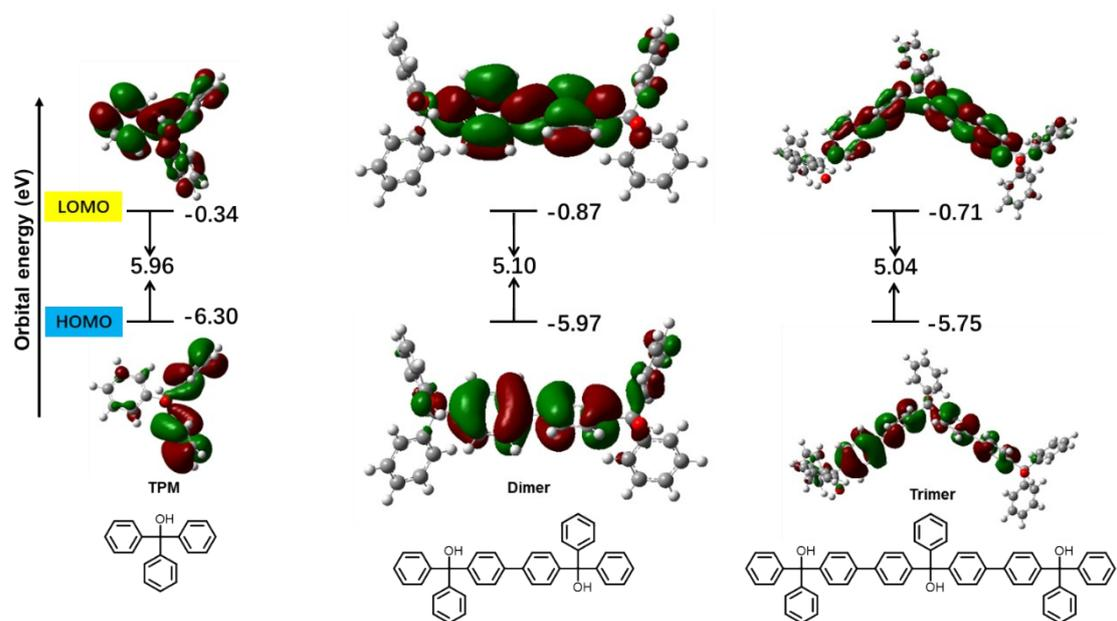
**Figure S15.** Electron cloud distributions and energy levels (eV) of TPM, dimer, trimer, in the geometry-optimized S1 state calculated by TD-DFT B3LYP/6-311G\*, Gaussian 09 program.
