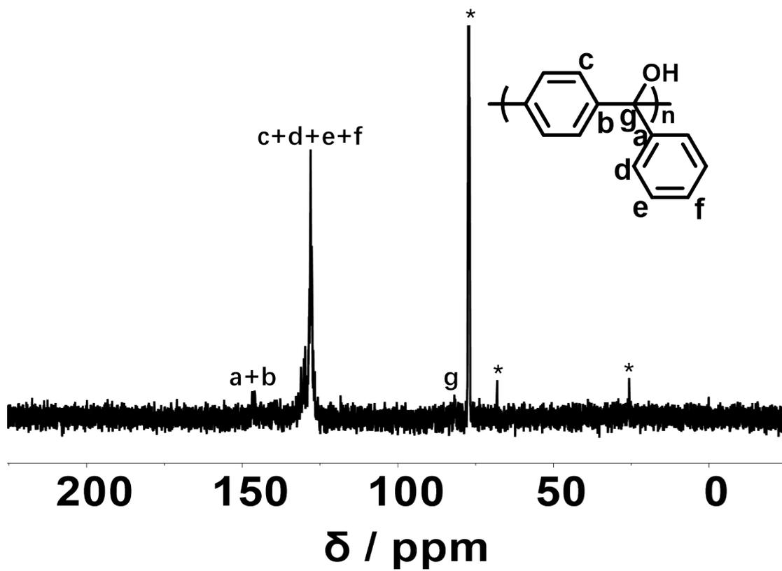
**Figure S3.**  $^{13}\text{C}$  (100 MHz) NMR spectrum of *p*-PTPM in  $\text{CDCl}_3$ . The solvent peaks are marked with asterisks.
