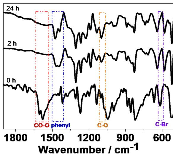
Figure S2. FT-IR spectra of polymerization kinetics.
