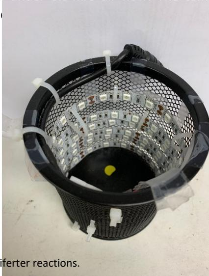
**Figure S1.** LED reactor used for photoiniferter reactions.
