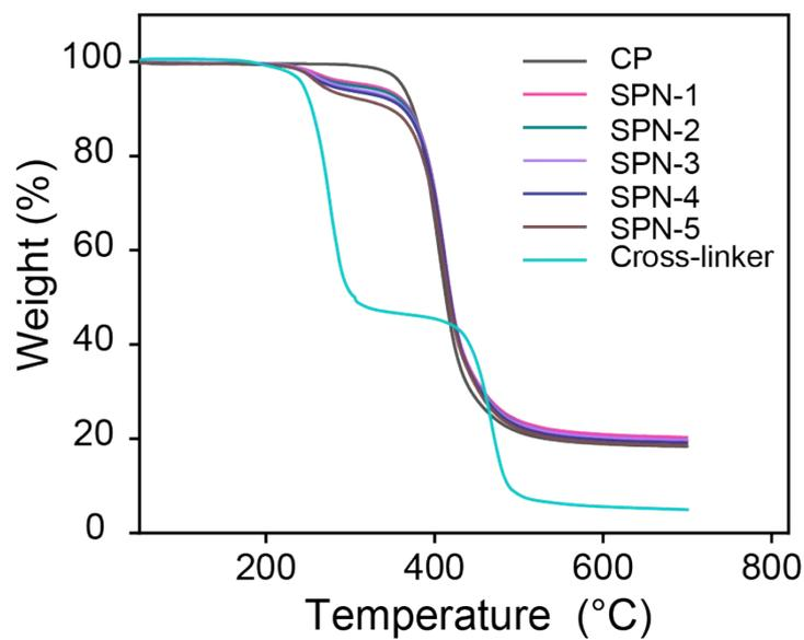
**Figure S13.** TGA curves of CP, SPNs-1–5 and cross-linker recorded under N<sub>2</sub> flow (50 mL/min) with a heating rate of 20 °C/min.
