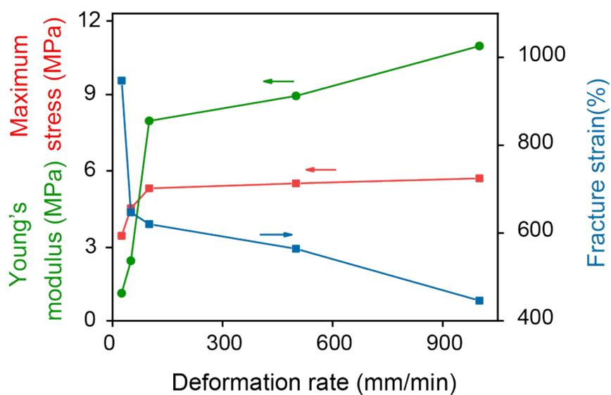
**Figure S14.** Deformation rate dependence of SPN-5 on maximum stress, Young's modulus and fracture strain calculated from their stress–strain curves in Fig 2d.
