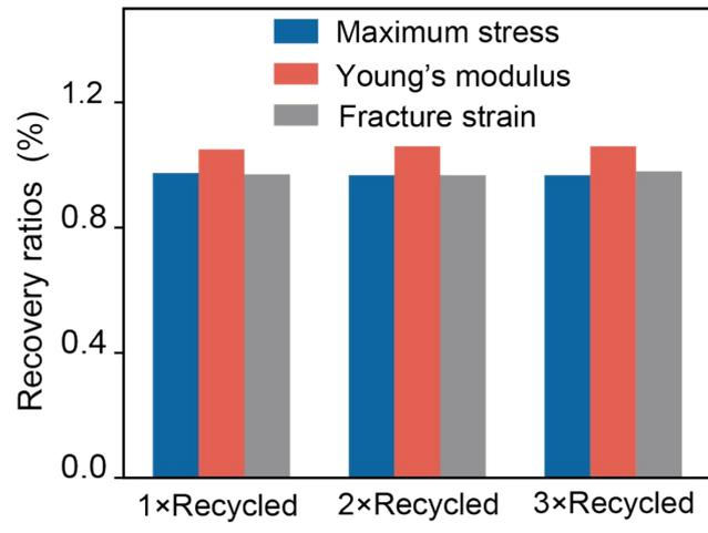
**Figure S15.** Recovery ratio of mechanical performance for recycled SPN-5 calculated from their stress–strain curves in Fig 4d.
