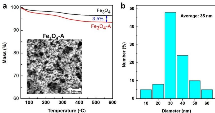
**Fig. S2.** (a) TGA curves of Fe<sub>3</sub>O<sub>4</sub> and Fe<sub>3</sub>O<sub>4</sub>-A (the insert showing the morphology of Fe<sub>3</sub>O<sub>4</sub>-A from SEM); (b) Diameter distribution of Fe<sub>3</sub>O<sub>4</sub>-A from SEM micrograph.
