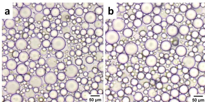
**Fig. S3.** Optical micrographs of (a) as-prepared HIPE (mPT-2) and (b) the HIPE after storage for a week.
