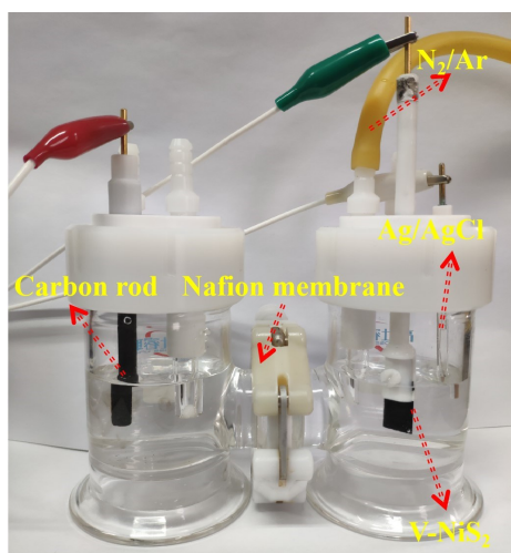
Figure S9. Gas-tight-two-compartment cell for NRR.
