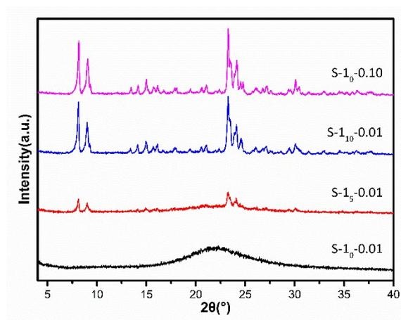
**Fig. S6** Experimental XRD patterns of the silicalite-1 crystallized from the initial reaction mixture with TPA<sup>+</sup>/SiO<sub>2</sub> ratio of 0.01 and seed loading of 0, 5, and 10 wt.% respecting to SiO<sub>2</sub>.
