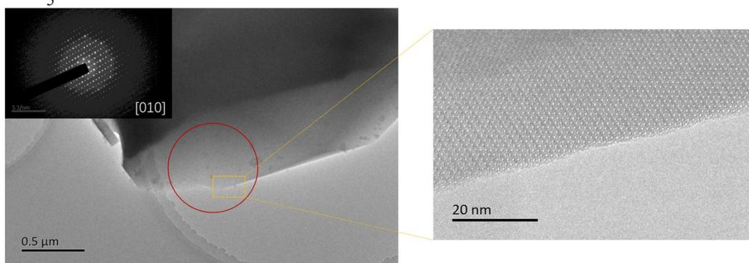
**Fig. S3** HRTEM images and selected area electron diffraction (SAED) of silicalite-1 crystallized from the initial reaction mixture with a TPA<sup>+</sup>/SiO<sub>2</sub> ratio of 0.035 and seed loading of 0, and 5 wt.% respecting to SiO<sub>2</sub>.
