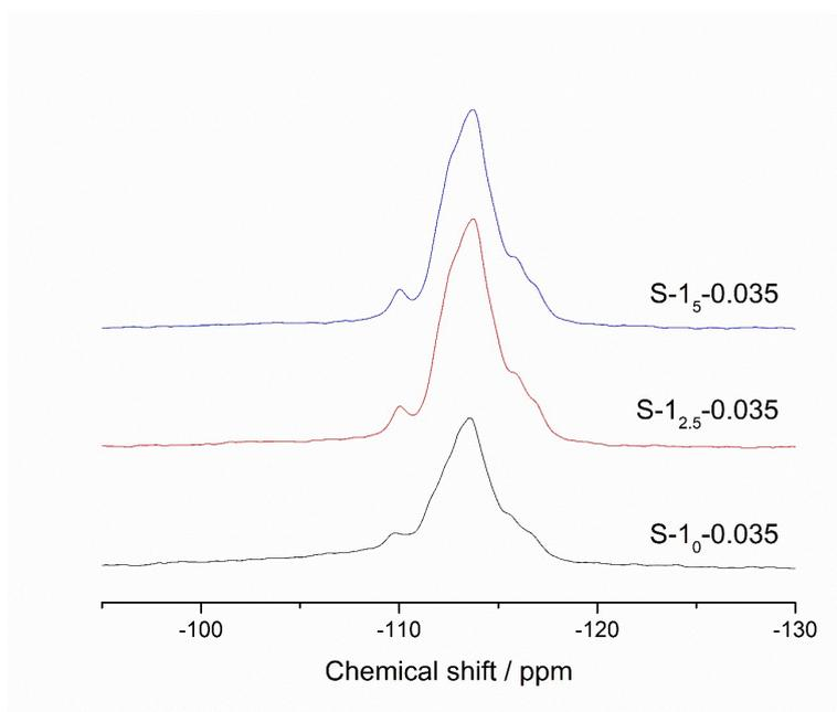
**Fig. S4** Solid-state  $^{29}\text{Si}$  MAS NMR spectra of silicalite-1 crystallized from the initial reaction mixture with a  $\text{TPA}^+/\text{SiO}_2$  ratio of 0.035 and seed loading of 0, 2.5, and 5 wt.% respecting to  $\text{SiO}_2$ .
