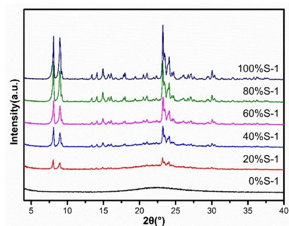
**Fig. S1** Experimental XRD patterns of the sample containing 0, 20, 40, 60, 80, and 100% standard silicalite-1 in amorphous silica.
