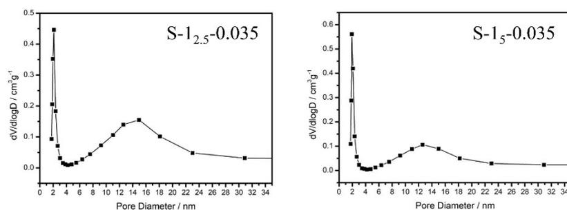
**Fig. S5** Pore size distribution of silicalite-1 crystallized from the initial reaction mixture with a  $\text{TPA}^+/\text{SiO}_2$  ratio of 0.035 and seed loading of 2.5, and 5 wt.% respecting to  $\text{SiO}_2$ .
