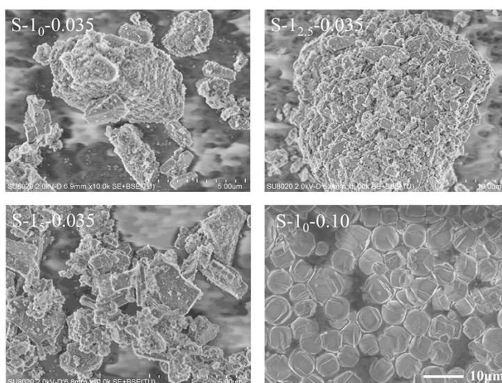
**Fig. S2** SEM images of silicalite-1 crystallized from the initial reaction mixture with a TPA<sup>+</sup>/SiO<sub>2</sub> ratio of 0.035 and seed loading of 0, 2.5, and 5 wt.% respecting to SiO<sub>2</sub> and a TPA<sup>+</sup>/SiO<sub>2</sub> ratio of 0.10 without seed.
