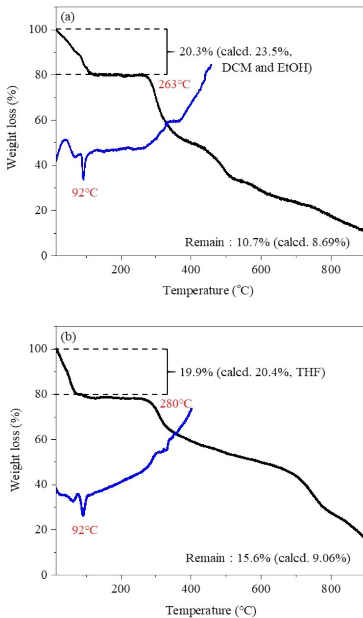
**Fig. S2** TGA and DSC overlays of  $3\text{CH}_2\text{Cl}_2 \cdot 2\text{C}_2\text{H}_5\text{OH}@\text{[CdI}_2\text{L]}$  (a) and  $4\text{C}_4\text{H}_8\text{O}@\text{[CdI}_2\text{L]}$  (b).
