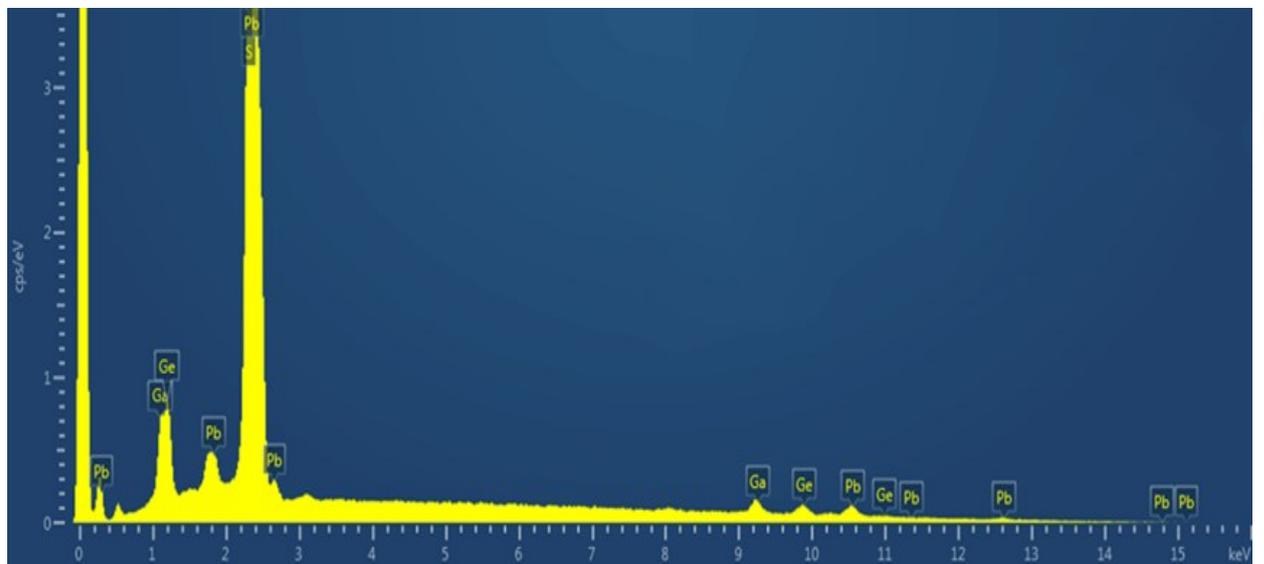
Fig. S2. EDS graph of  $\text{Pb}^{2+}$ -loaded material.
