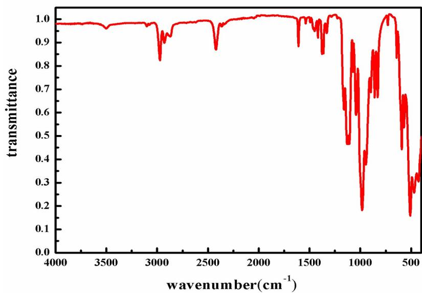
Figure S100. FTIR spectra for PTC-150.
