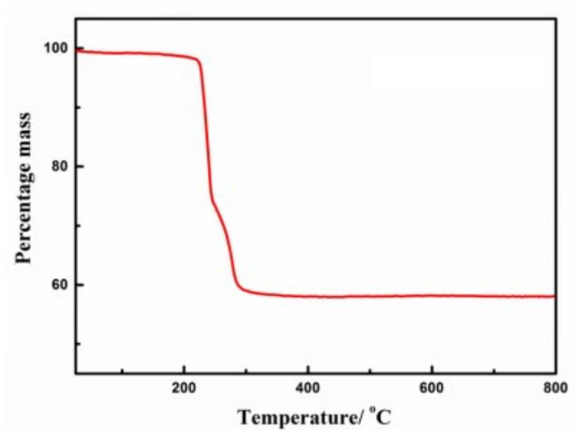
Figure S68. Thermal analysis of PTC-144
