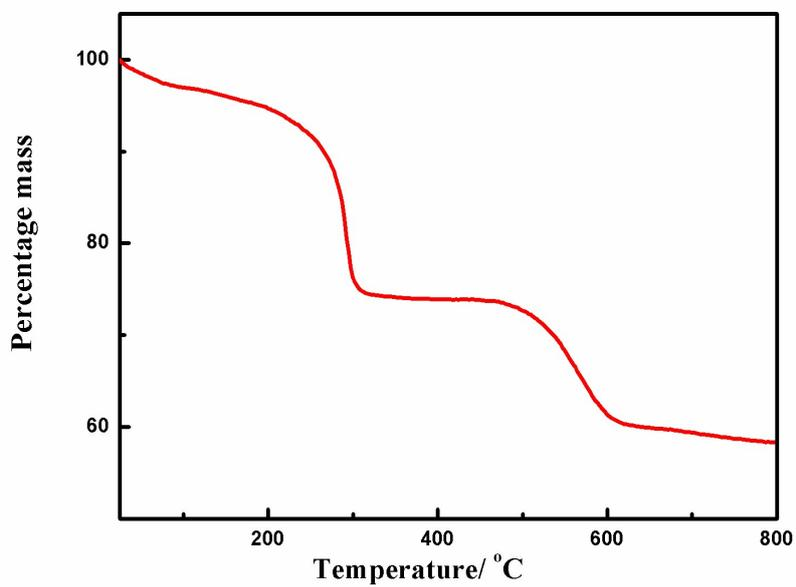
Figure S103. Thermal analysis of PTC-151
