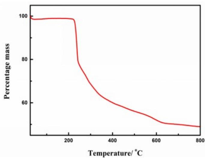
Figure S28. Thermal analysis of PTC-136
