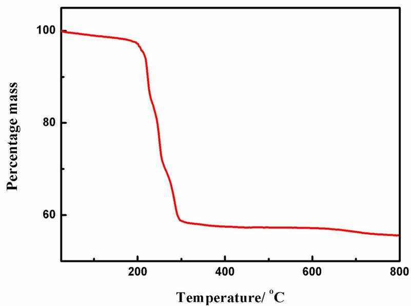
Figure S77. Thermal analysis of PTC-146
