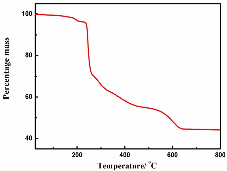
Figure S88. Thermal analysis of PTC-148
