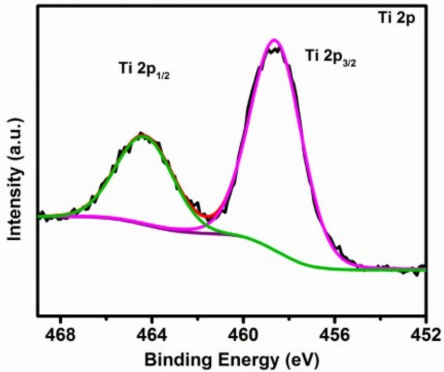
Figure S114.XPS for Ti2p for PTC-150
