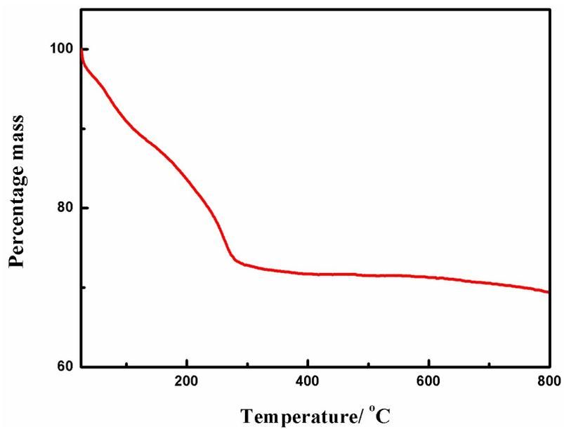
Figure S77. Thermal analysis of PTC-147
