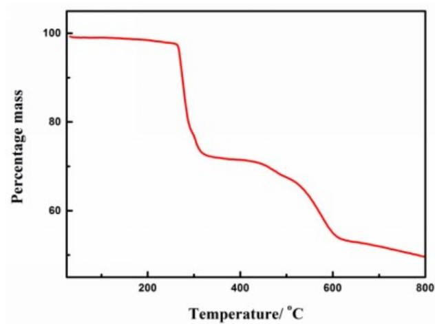
Figure S53. Thermal analysis of PTC-141
