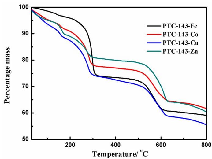
Figure S63. Thermal analysis of PTC-143
