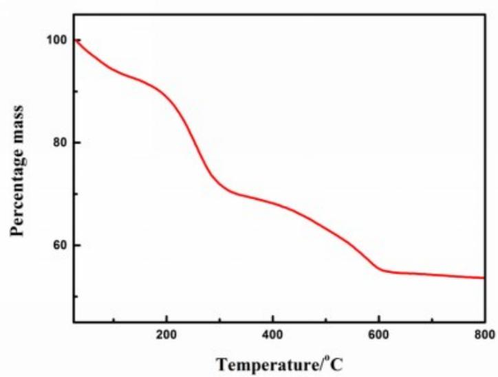
**Figure S13.** Thermal analysis of PTC-133
