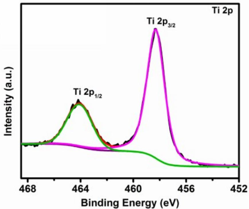
Figure S115.XPS for Ti2p for PTC-150A
