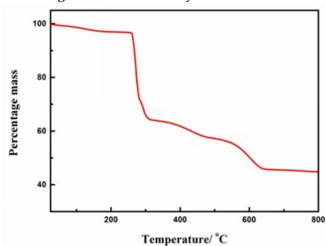
**Figure S43.** Thermal analysis of PTC-139
