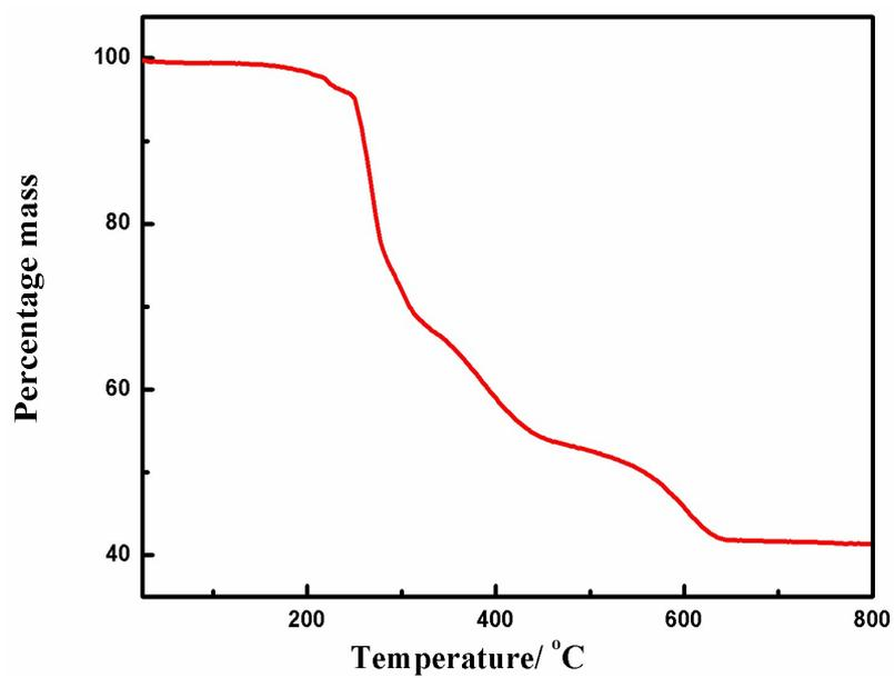
Figure S93. Thermal analysis of PTC-149
