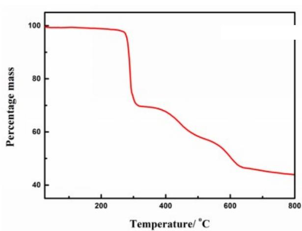
**Figure S48.** Thermal analysis of PTC-140
