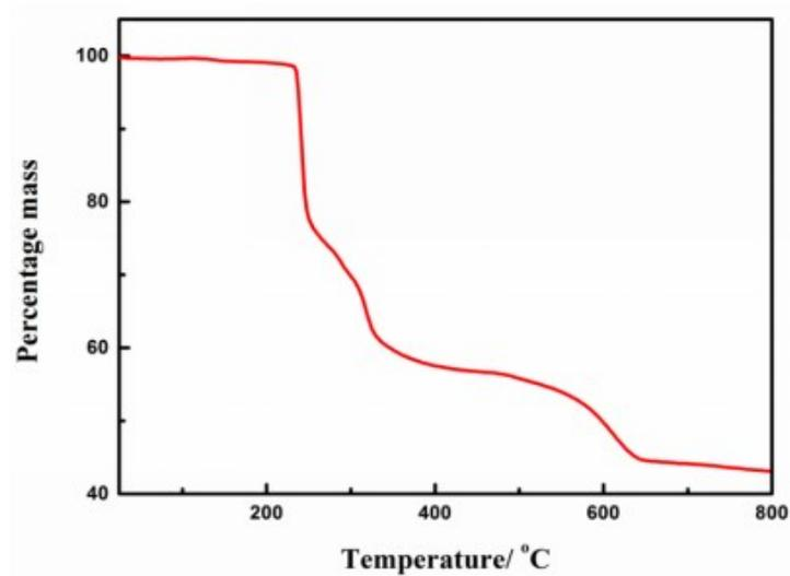
**Figure S18.** Thermal analysis of PTC-134
