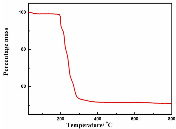
**Figure S98.** Thermal analysis of PTC-150
