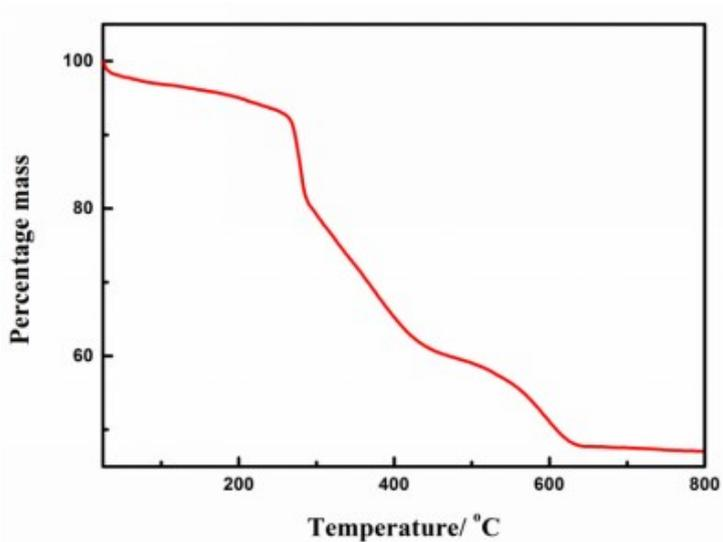
Figure S23. Thermal analysis of PTC-135
