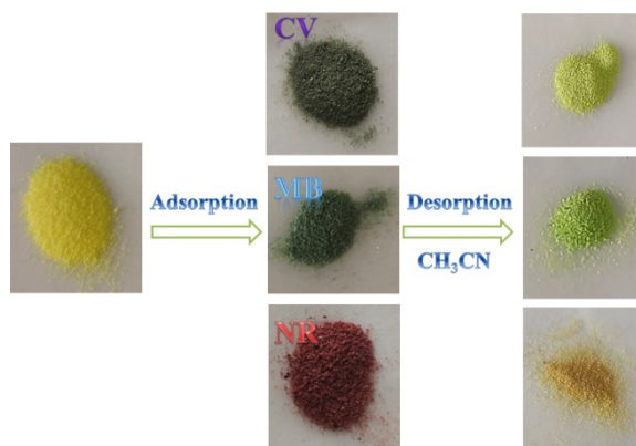
Fig. S7. The color change after adsorbing CV, MB, NR of 1 as adsorbent.
