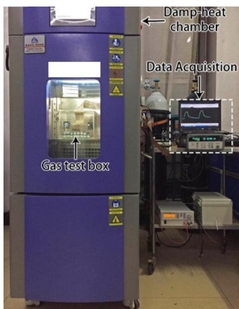
Fig. S1 Homemade chemical gas sensing analysis system. The gas test box is placed in a cyclic damp heat test instrument (left) with the controllable temperature and relative humidity.
