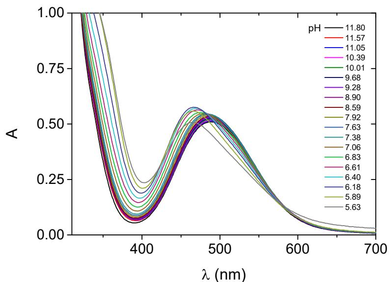
**Figure S5.** pH-dependent UV-vis spectra recorded in the Ni(II)/wtPen system at 0.9:1 metal to ligand ratio.  $l = 10$  mm,  $I = 0.2$  M KCl,  $T = 25$  °C,  $c_{\text{wtPen}} = 2$  mM
