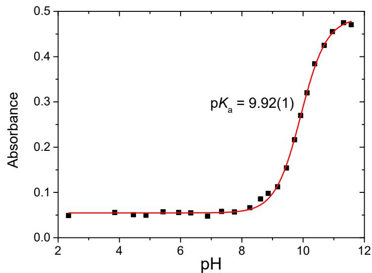
**Figure S3.** Experimental (squares) and fitted (solid line) absorbances at 291 nm as a function of pH recorded in the  $\text{H}^+/\text{wtPen}$  system.  $l = 2\text{mm}$ ,  $I = 0.2\text{ M KCl}$ ,  $T = 25\text{ }^\circ\text{C}$ ,  $c_{\text{wtPen}} = 1\text{ mM}$
