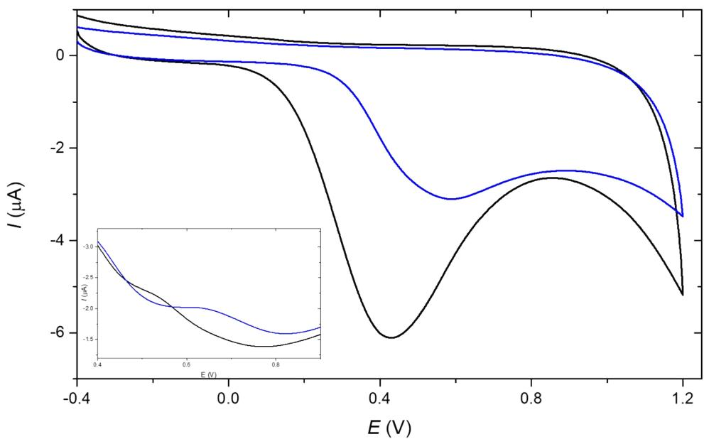
**Figure S10.** CV and DPC (inset) curves recorded in the Ni/wtPen (blue) and Ni/wtSOD (black) systems at pH 7.6 in 0.1 M NaClO<sub>4</sub>.  $c_{\text{complex}} = 2 \text{ mM}$
