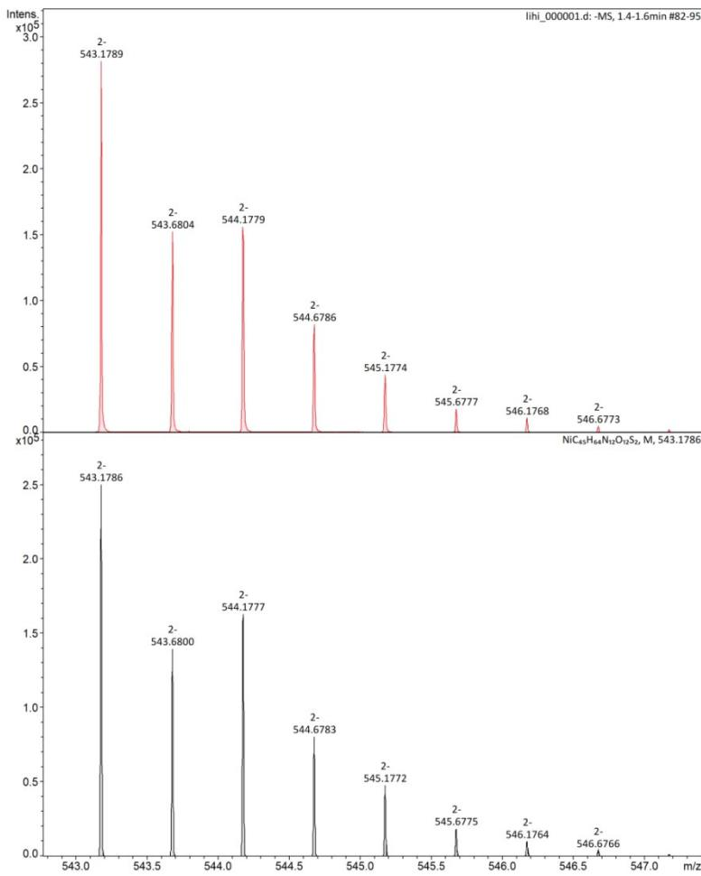
**Figure S8.** Experimental (top) and calculated isotopic patterns of the  $[\text{NiH}_{-1}\text{L}]^{2-}$  species (bottom), L refers to wtPen.
