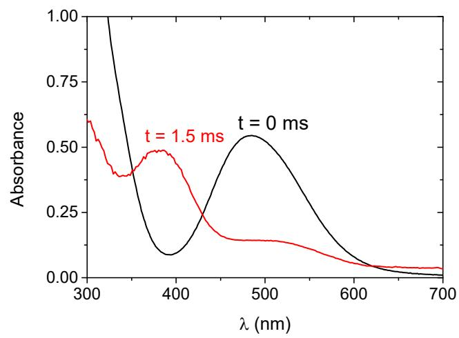
**Figure S13.** Electronic absorption spectra recorded in the Ni(II)/wtPen system in 1:1 aqueous HEPES buffer (50 mM, pH 7.6) / DMSO mixture before (black) and after mixing with  $\text{KO}_2$ .  $c(\text{complex})^0 = 0.2 \text{ mM}$ ;  $c(\text{O}_2^-)^0 = 0.41 \text{ mM}$ ,  $l = 10 \text{ mm}$
