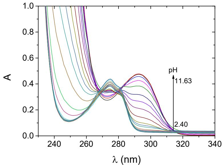
**Figure S2.** pH-dependent UV-vis spectra recorded in the  $\text{H}^+/\text{wtPen}$  system.  $l = 2 \text{ mm}$ ,  $I = 0.2 \text{ M KCl}$ ,  $T = 25^\circ\text{C}$ ,  $c_{\text{wtPen}} = 1 \text{ mM}$
