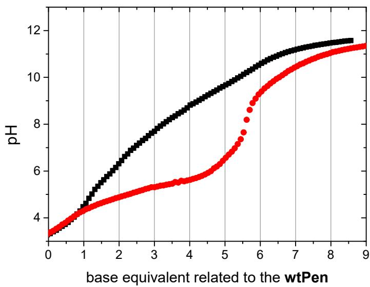
**Figure S1.** Representative titration curves of the  $\text{H}^+/\text{wtPen}$  (black) and  $\text{Ni}(\text{II})/\text{wtPen}$  (red) systems at 0.9:1 metal to ligand ratio.  $I = 0.2 \text{ M KCl}$ ,  $T = 25^\circ\text{C}$ ,  $c_{\text{wtPen}} = 2 \text{ mM}$
