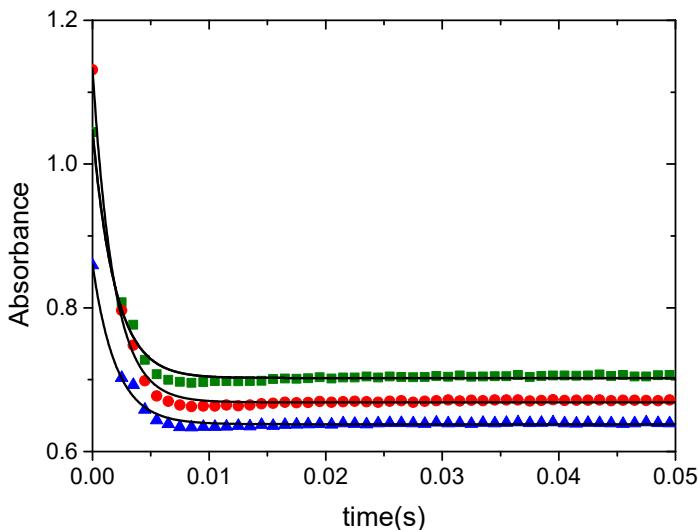
**Figure S16.** Kinetic traces recorded in the presence of Ni(wtNiSOD) complex at comparable concentrations of superoxide anion.  $c(\text{complex})^0 = 0.20$  mM;  $c(\text{O}_2^-)^0 = 0.51$  mM (blue), 0.86 mM (red) and 1.02 mM (green). Solid lines represent the fitted kinetic traces on the basis of the proposed kinetic model. Solvent 1:1 aqueous HEPES buffer (50 mM, pH 7.6) / DMSO mixture.  $\lambda = 260$  nm,  $l = 2$  mm.
