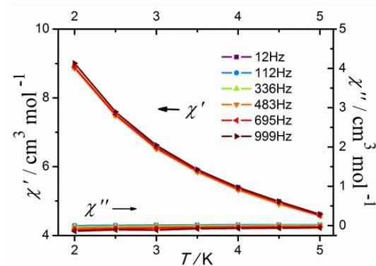
**Fig. S27.** Temperature-dependent  $\chi'$  and  $\chi''$  ac susceptibilities under zero dc field for **1**.
