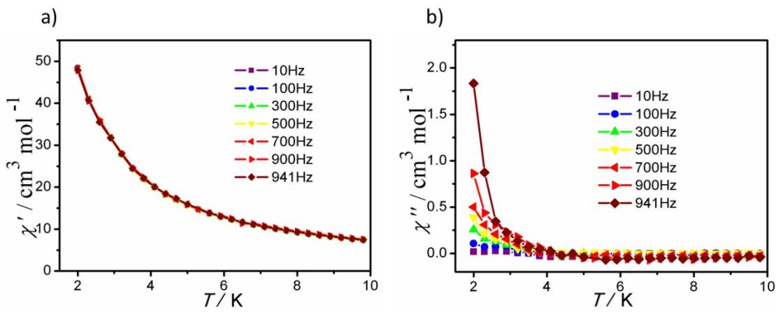
**Fig. S28.** Temperature-dependent  $\chi'$  (a) and  $\chi''$  (b) ac susceptibilities under zero dc field for **2**.
