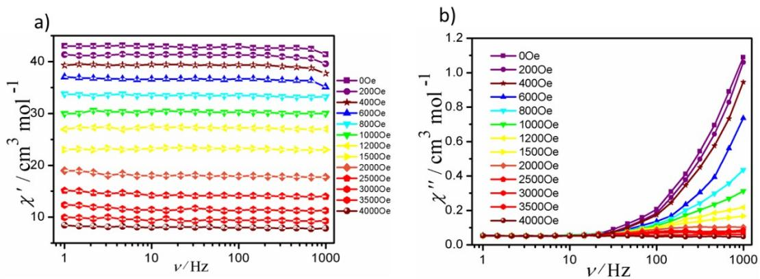
**Fig. S25.** Plots of  $\chi'$  and  $\chi''$  vs  $\nu$  at 2-5.0 K under different dc field of 0 Oe for **2**.
