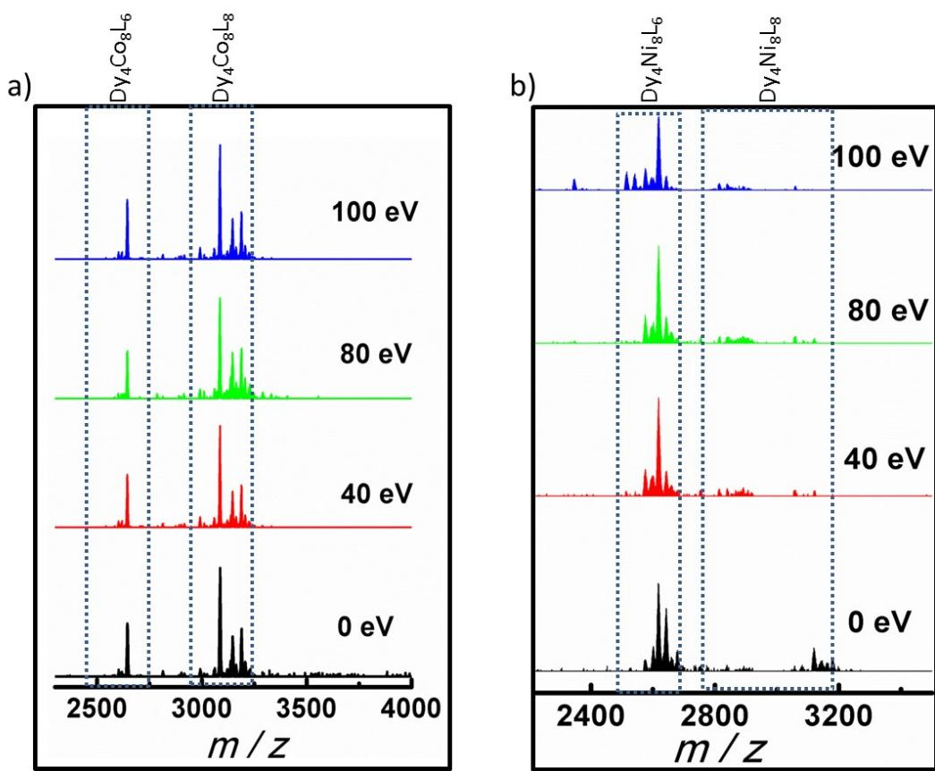
**Fig. S12.** Molecular ion peaks of 1 (a) and 2 (b) in cation modes obtained by HRESI-MS test with different ion source voltages (0, 40, 80 and 100 eV).
