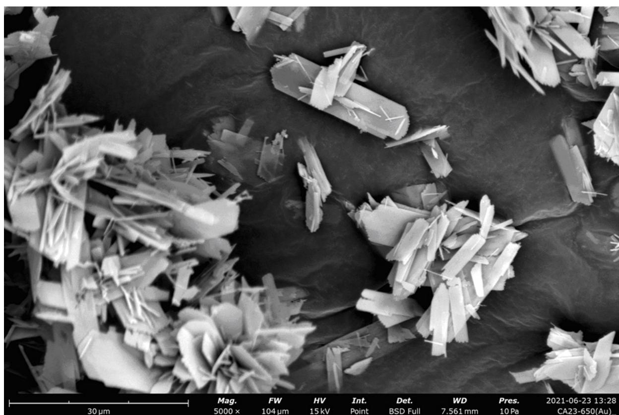
Fig. S2 SEM images of CAP microcrystals (Table 1, Entry 1), sintered at 650 °C.
