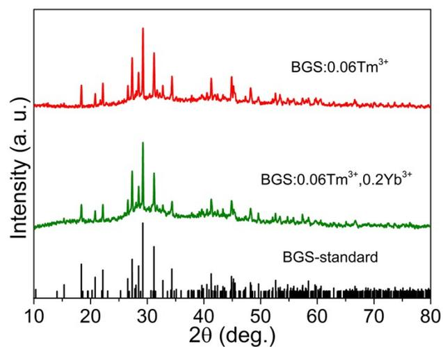
Figure S1 XRD patterns of BGS:0.06Tm<sup>3+</sup> and BGS:0.06Tm<sup>3+</sup>,0.2Yb<sup>3+</sup>
