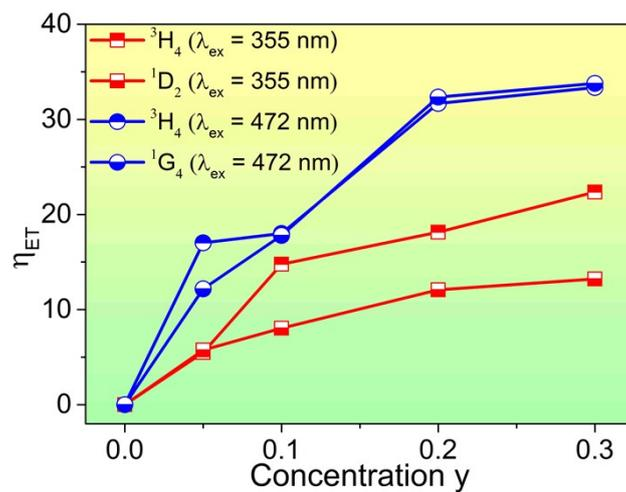
Figure S9 ET efficiencies ( $\eta_{ET}$ ) of BGS:0.06 $\text{Tm}^{3+}$ , $y\text{Yb}^{3+}$  ( $0 \leq y \leq 0.3$ ) from different excited states of  $\text{Tm}^{3+}$  to  $\text{Yb}^{3+}$  excited by different wavelengths
