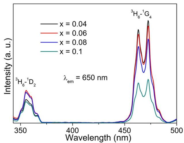
Figure S7 Excitation spectra of BGS:xTm<sup>3+</sup> ( $0.04 \leq x \leq 0.1$ ) monitored at 650 nm
