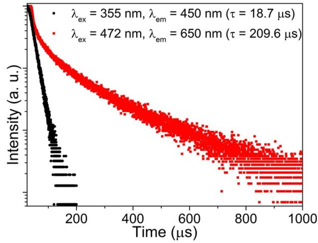
Figure S3 Decay curves of BGS:0.06Tm<sup>3+</sup>
