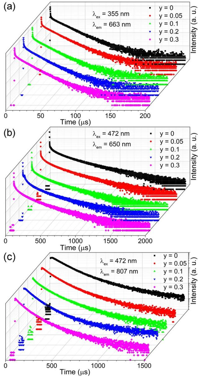
Figure S8 Decay curves of BGS:0.06Tm<sup>3+</sup>,yYb<sup>3+</sup> (0 ≤ y ≤ 0.3) measured under different conditions: (a)  $\lambda_{\text{ex}} = 355 \text{ nm}$ ,  $\lambda_{\text{em}} = 663 \text{ nm}$ ; (b)  $\lambda_{\text{ex}} = 472 \text{ nm}$ ,  $\lambda_{\text{em}} = 650 \text{ nm}$ ; (c)  $\lambda_{\text{ex}} = 472 \text{ nm}$ ,  $\lambda_{\text{em}} = 807 \text{ nm}$
