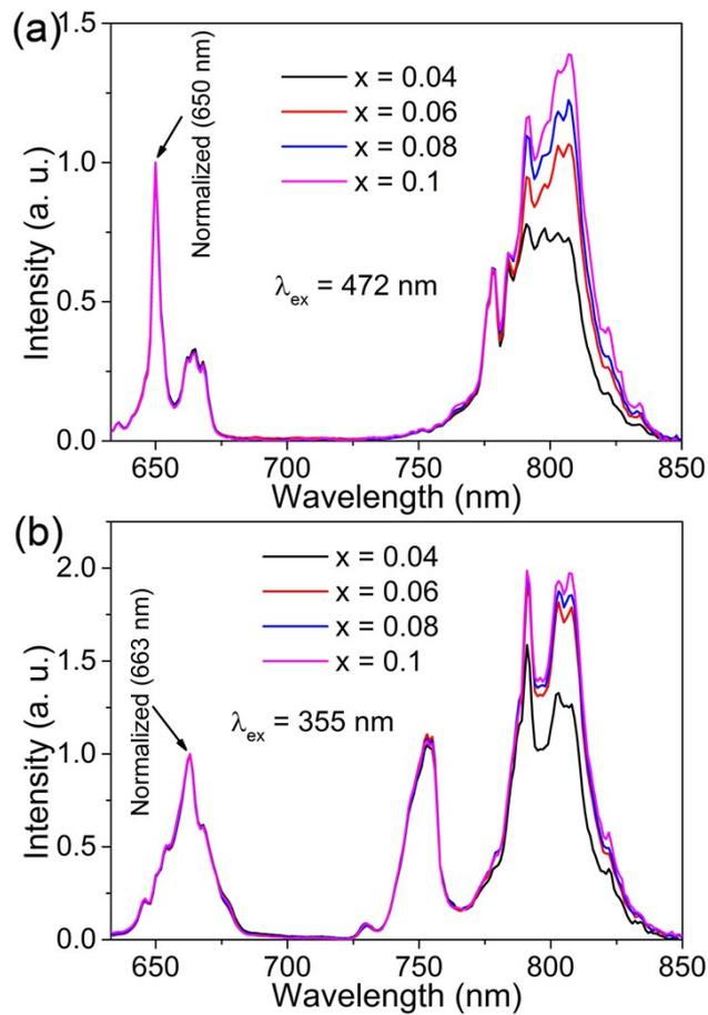
Figure S4 Normalized emission spectra of BGS:xTm<sup>3+</sup> ( $0.04 \leq x \leq 0.1$ ) under (a) 472 and (b) 355 nm excitation
