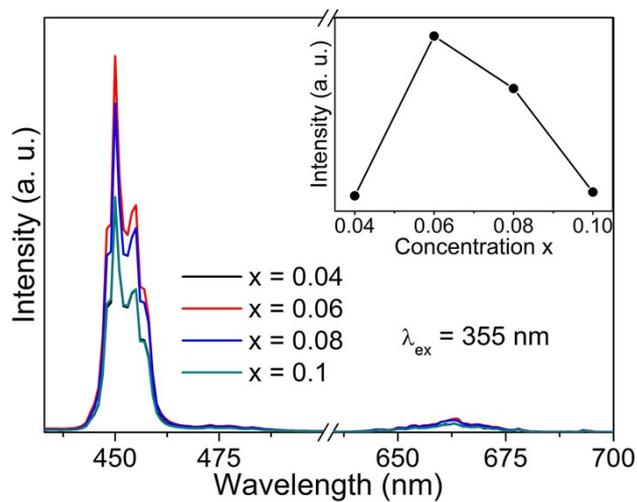
Figure S5 Emission spectra of BGS: $x\text{Tm}^{3+}$  ( $0.04 \leq x \leq 0.1$ ) under 355 nm excitation, inset shows the dependence of 450 nm emission intensity on  $\text{Tm}^{3+}$  concentration
