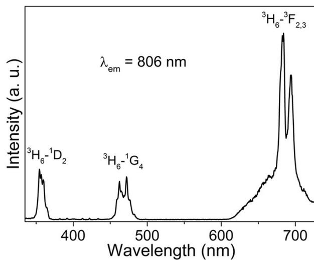
Figure S2 Excitation spectrum of BGS:0.06Tm<sup>3+</sup> monitored at 806 nm
