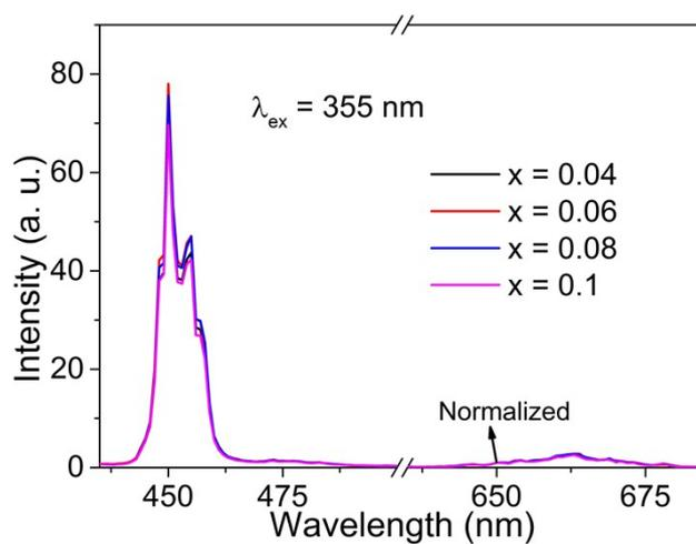
Figure S6 Normalized (for 650 nm) emission spectra of BGS: $x\text{Tm}^{3+}$  ( $0.04 \leq x \leq 0.1$ ) under 355 nm excitation
