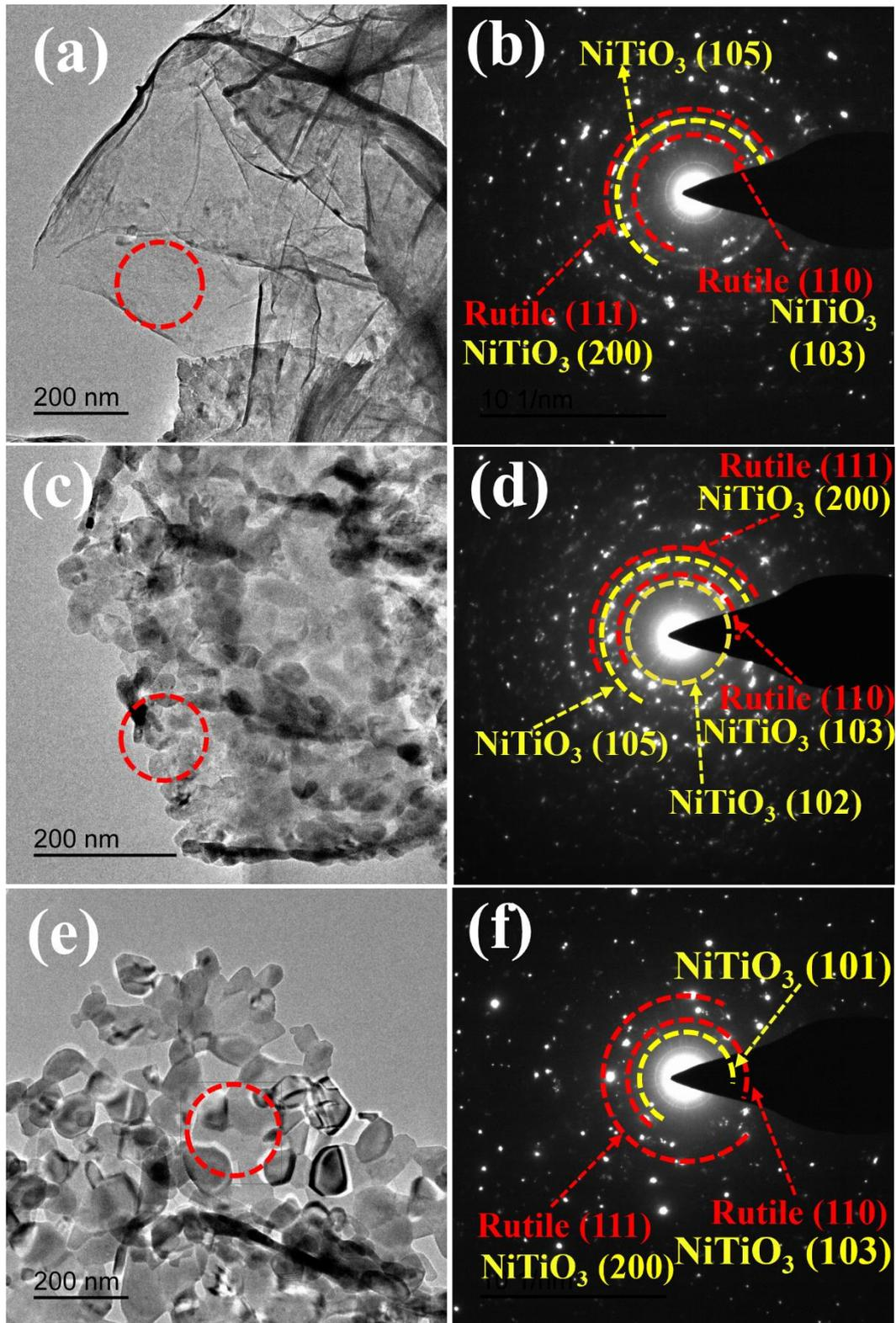
Fig.S3 TEM images and SAED patterns of (a, b) Ni-H<sub>2</sub>O<sub>2</sub>-HTO-ns-500, (c, d) Ni-H<sub>2</sub>O<sub>2</sub>-HTO-ns-600, (e, f) Ni-H<sub>2</sub>O<sub>2</sub>-HTO-ns-700
