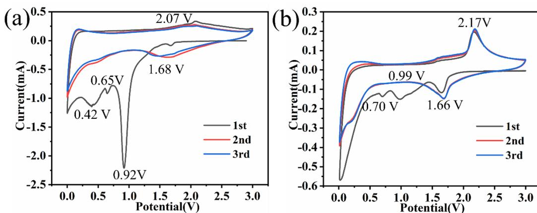
**Fig. S10** Cyclic voltammetry (CV) curves of (a) Ni-H<sub>2</sub>O<sub>2</sub>-HTO-ns-600 and (b) Ni-H<sub>2</sub>O<sub>2</sub>-HTO-600 at scan rate of 0.1 mV/s.
