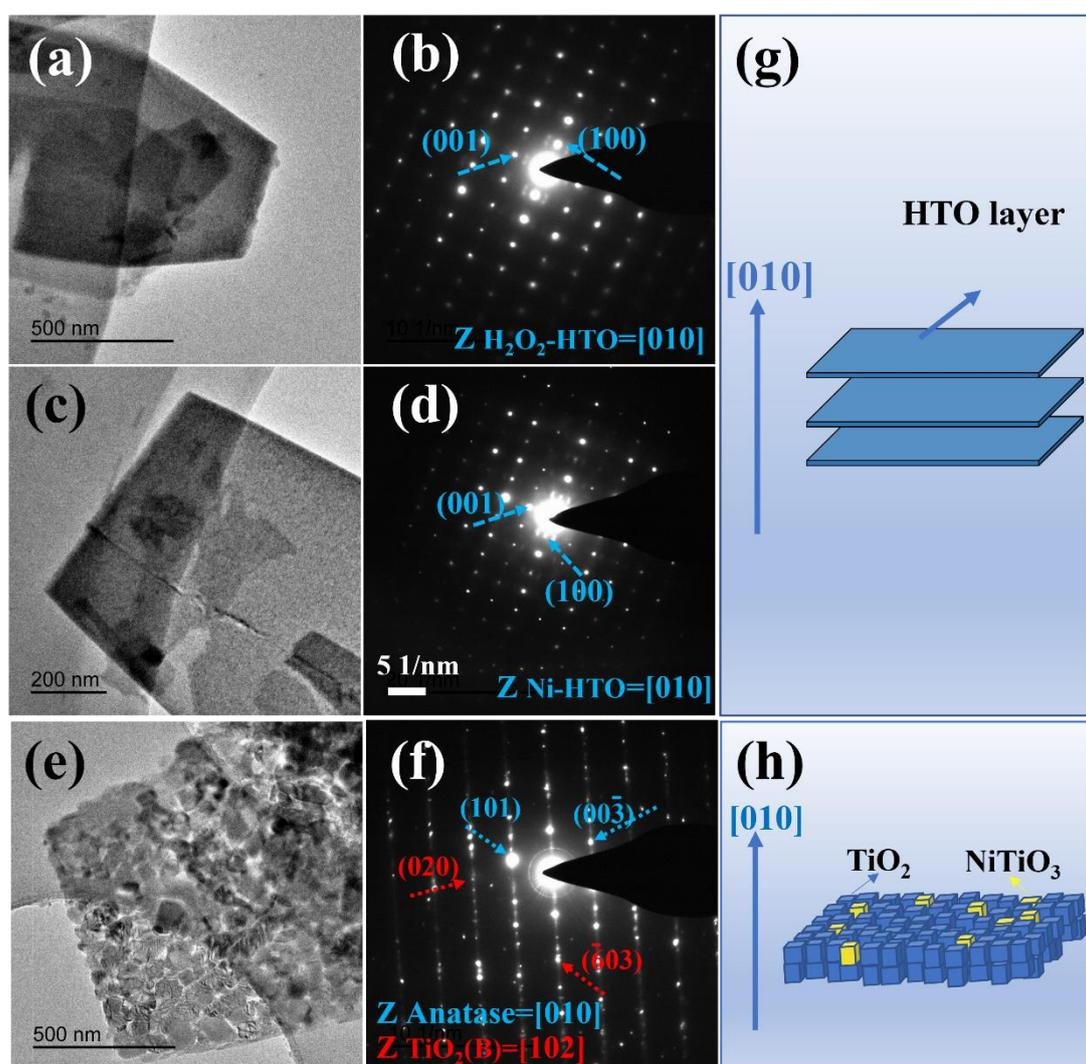
**Fig. S5** TEM images and SAED patterns of (a, b) H<sub>2</sub>O<sub>2</sub>-HTO, (c, d) Ni-HTO, (e, f) Ni-HTO-600, and (g, h) corresponding layered structures.
