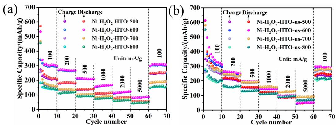
Fig. S7 Rate capabilities of (a) mesocrystalline  $\text{NiTiO}_3/\text{TiO}_2$  nanocomposites and (b) polycrystalline  $\text{NiTiO}_3/\text{TiO}_2$  nanocomposites obtained by heat-treatment of  $\text{Ni-H}_2\text{O}_2\text{-HTO}$  and  $\text{Ni-H}_2\text{O}_2\text{-HTO-ns}$  at 500, 600, 700 and 800 °C, respectively.
