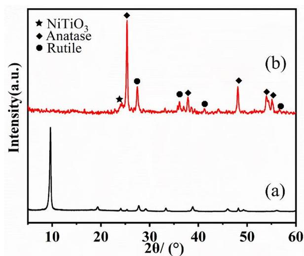
**Fig. S2** XRD patterns of (a) Ni-HTO and (b) product after heat-treatment of Ni-HTO at 600 °C.
