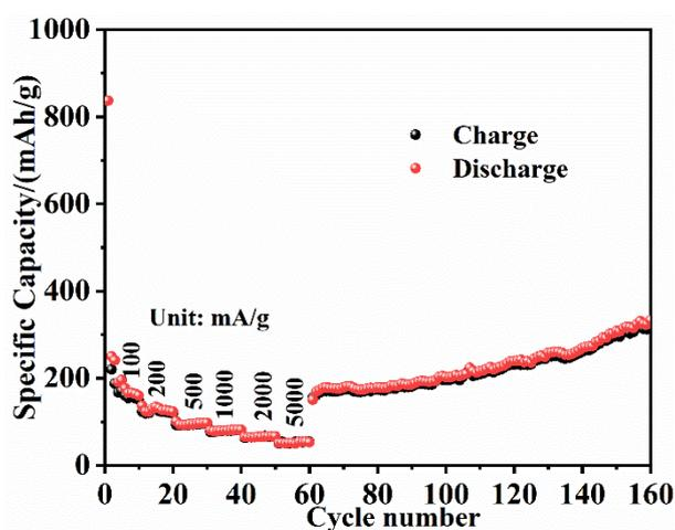
**Fig. S8** Rate capabilities and cycle performance at 100 mA/g for pure NiTiO<sub>3</sub> obtained by solid-state reaction.
