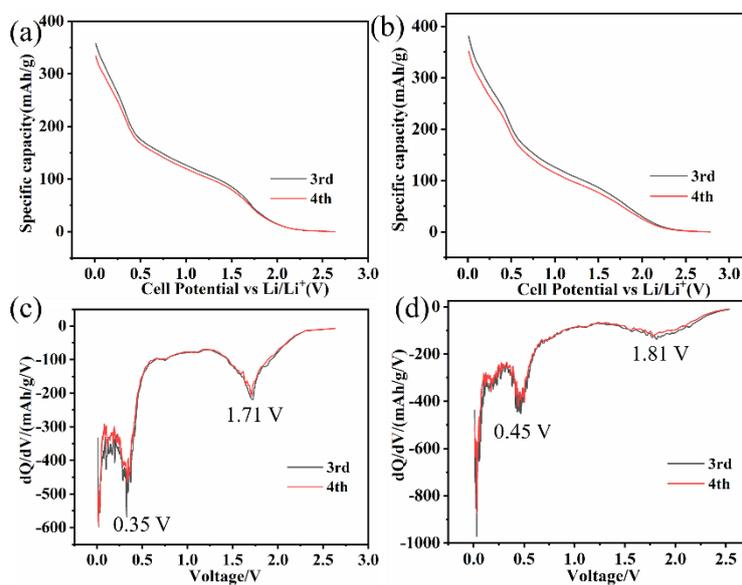
**Fig. S11** Discharge profiles at a current density of 100 mA/g for (a) Ni-H<sub>2</sub>O<sub>2</sub>-HTO-600 and (b) Ni-H<sub>2</sub>O<sub>2</sub>-HTO-ns-600; dQ/dV discharge curves for (c) Ni-H<sub>2</sub>O<sub>2</sub>-HTO-600 and (d) Ni-H<sub>2</sub>O<sub>2</sub>-HTO-ns-600 obtained from their discharge profiles.
