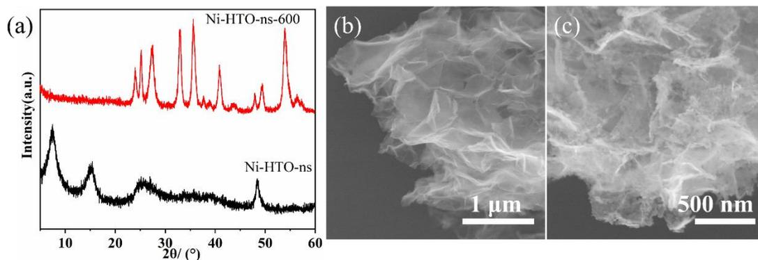
**Fig. S4** XRD patterns of (a) Ni-HTO-ns and its heat-treated product at 600°C, FE-SEM images of (b) Ni-HTO-ns and (c) its heat-treated product at 600°C.
