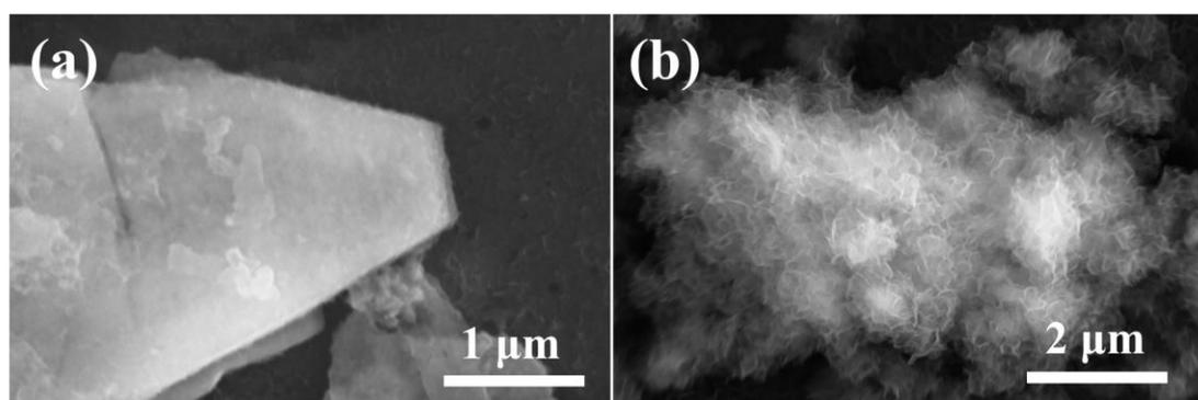
**Fig. S9** *Ex-situ* SEM images of (a) Ni-H<sub>2</sub>O<sub>2</sub>-HTO-600 (b) Ni-H<sub>2</sub>O<sub>2</sub>-HTO-ns-600 after 100 cycles at 100 mA/g.
