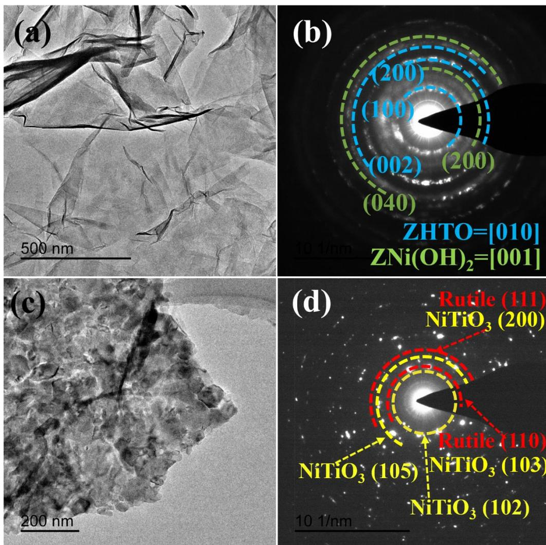
Fig. S6 TEM images and SAED patterns of (a, b) Ni-HTO-ns, (c, d) Ni-HTO-ns-600.
