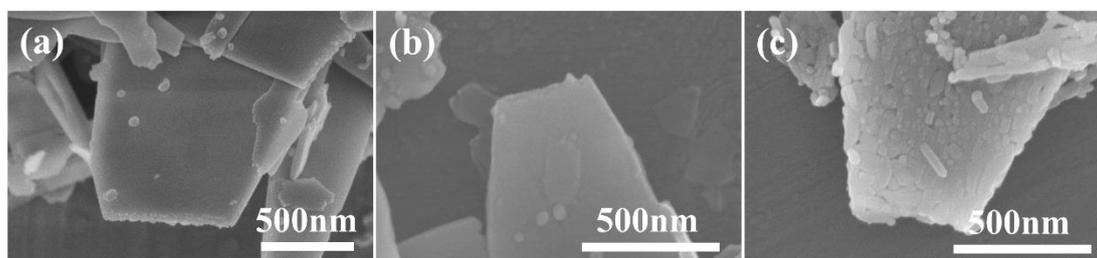
**Fig. S1** FE-SEM images of (a) H<sub>2</sub>O<sub>2</sub>-HTO, (b) Ni-HTO and (c) products after heated Ni-HTO at 600 °C.
