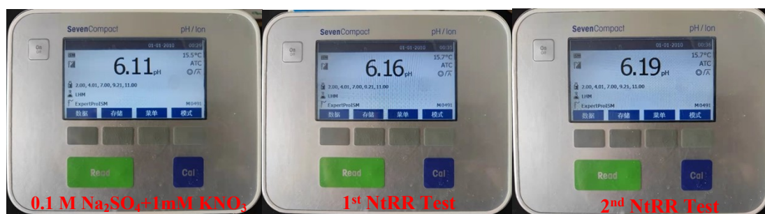
Fig. S12. Photograph of the pH value of cathodic electrolyte for two replicated tests after 2 h NiRR at -0.85 V vs. RHE.
