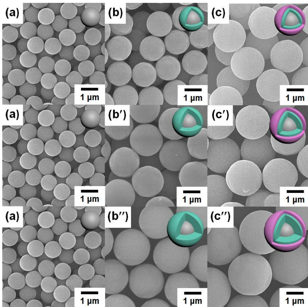
**Fig. S13.** Preparation of three different silica@TbCP@GdCP samples with various TbCP thicknesses. SEM images of (a) carboxylic acid-terminated silica, (b, b', b'') three different silica@TbCP samples with TbCP thicknesses of 255, 435, or 550 nm, and (c, c', c'') three different silica@TbCP@GdCP samples with various TbCP thicknesses.
