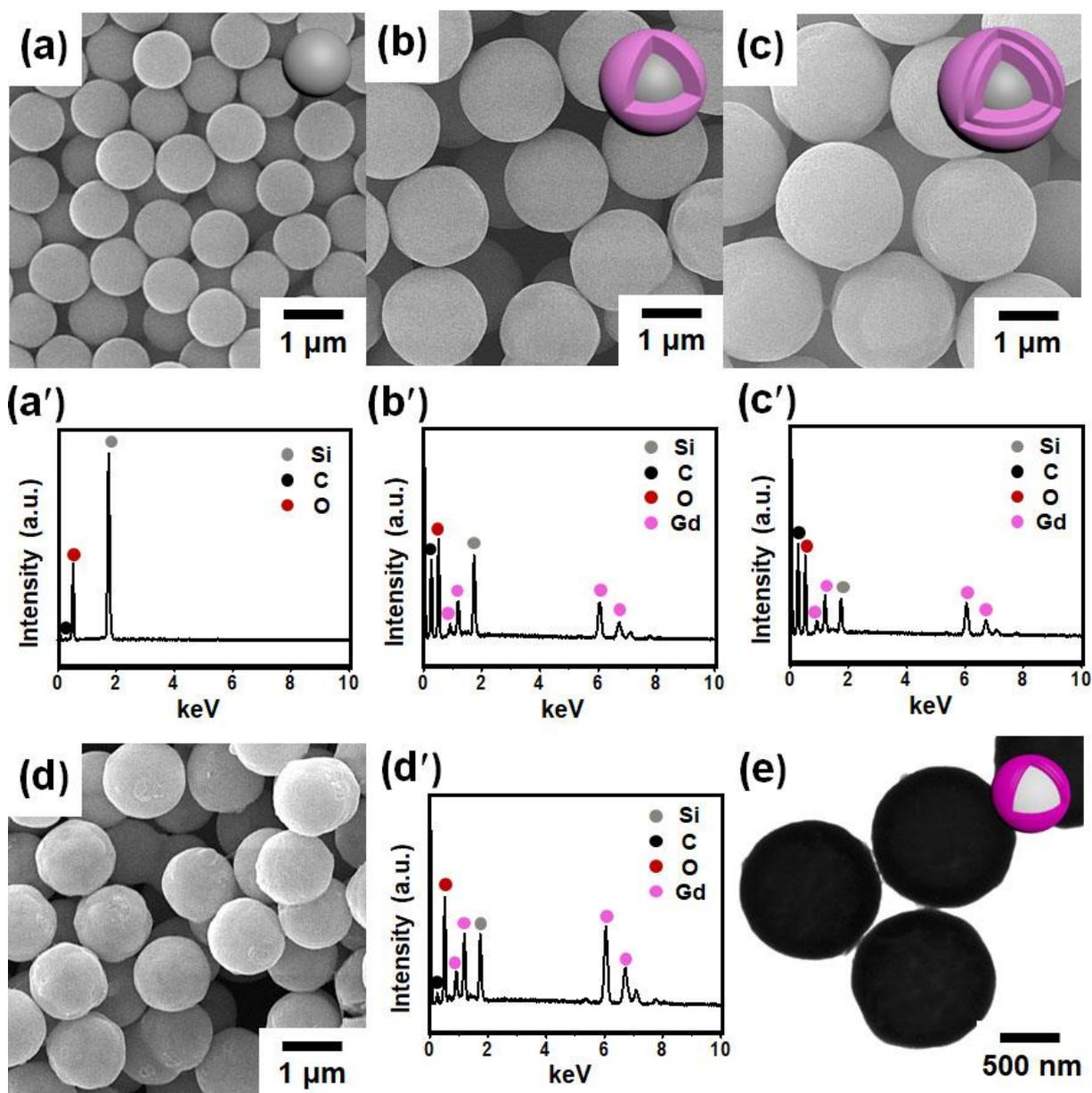
**Fig. S7.** SEM images of (a) carboxylic acid-terminated silica, (b) core-shell of silica@GdCP, and (c) silica@GdCP@GdCP. EDX spectra of (a') carboxylic acid-terminated silica, (b') silica@GdCP, and (c') silica@GdCP@GdCP. (d) SEM image, (d') EDX spectrum, and (e) TEM image of core-shell-type metal oxide of silica@Gd<sub>2</sub>O<sub>3</sub>@Gd<sub>2</sub>O<sub>3</sub>.
