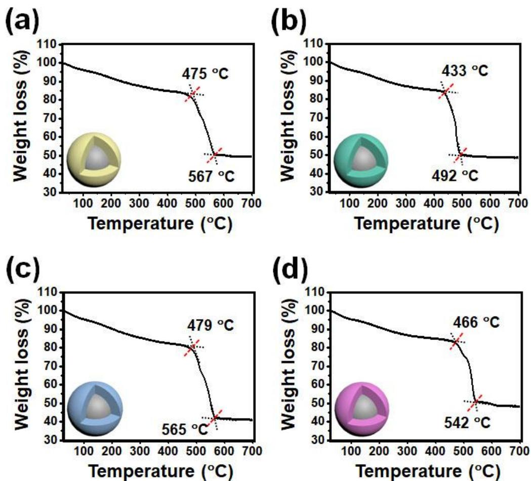
**Fig. S10.** TGA curves of single-layered core-shell microspheres of (a) silica@ErCP, (b) silica@TbCP, (c) silica@YCP, and (d) silica@GdCP.
