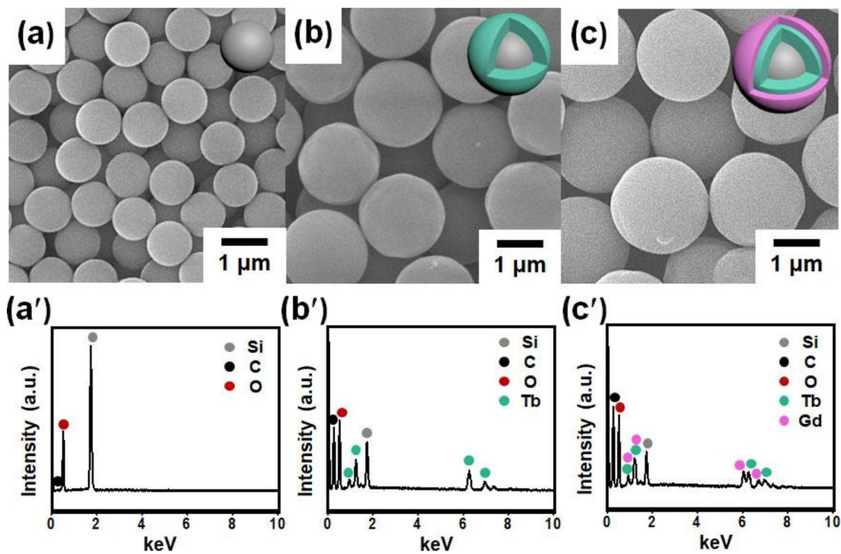
**Fig. S3.** SEM images of (a) carboxylic acid-terminated silica, (b) core-shell of silica@TbCP, and (c) silica-templated CP double layer of silica@TbCP@GdCP. EDX spectra of (a') carboxylic acid-terminated silica, (b') silica@TbCP, and (c') silica@TbCP@GdCP.
