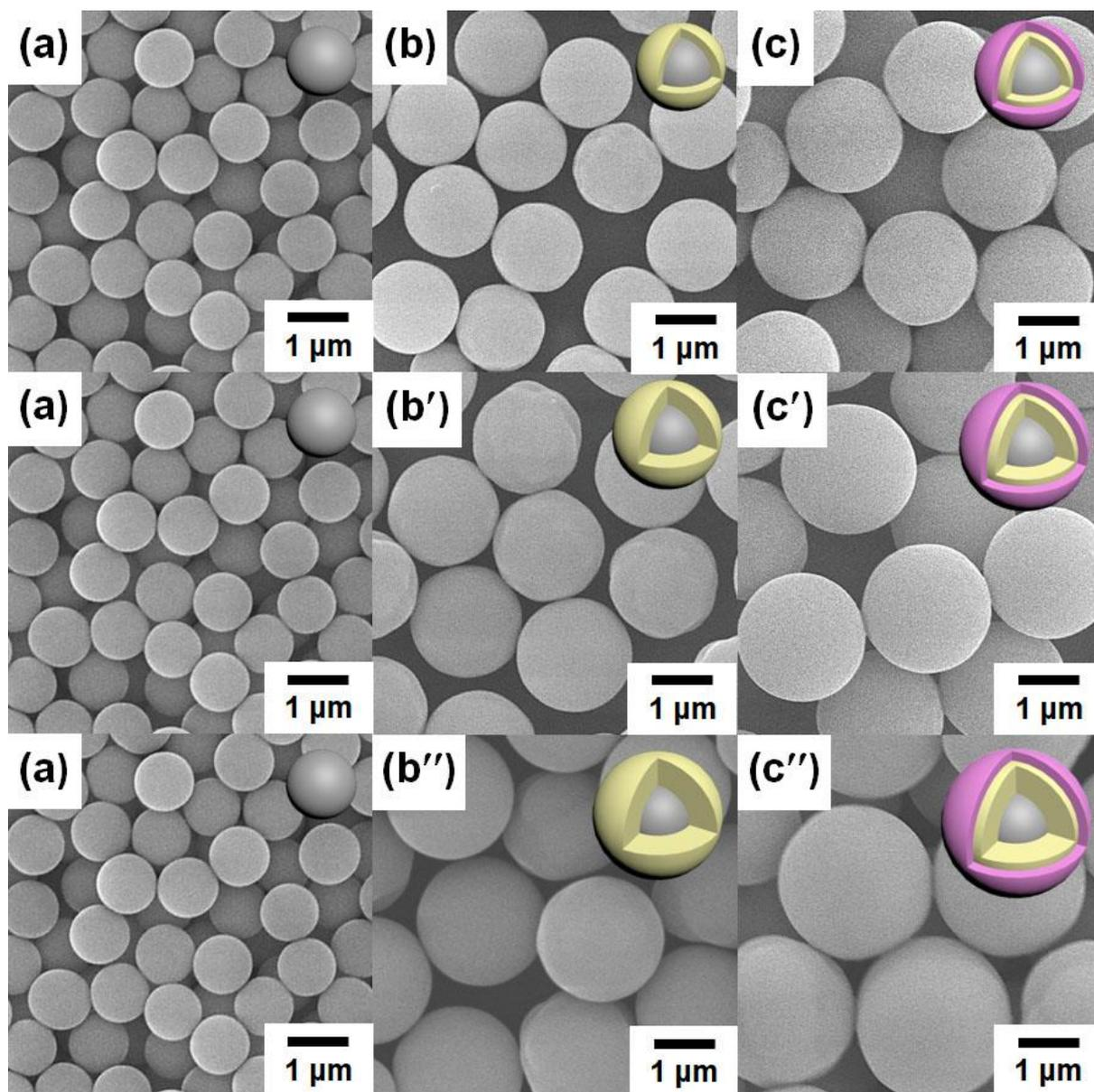
**Fig. S12.** Preparation of three different silica@ErCP@GdCP samples with various ErCP thicknesses. SEM images of (a) carboxylic acid-terminated silica, (b, b', b'') three different silica@ErCP samples with ErCP thicknesses of 265, 435, or 570 nm, and (c, c', c'') three different silica@ErCP@GdCP samples with various ErCP thicknesses.
