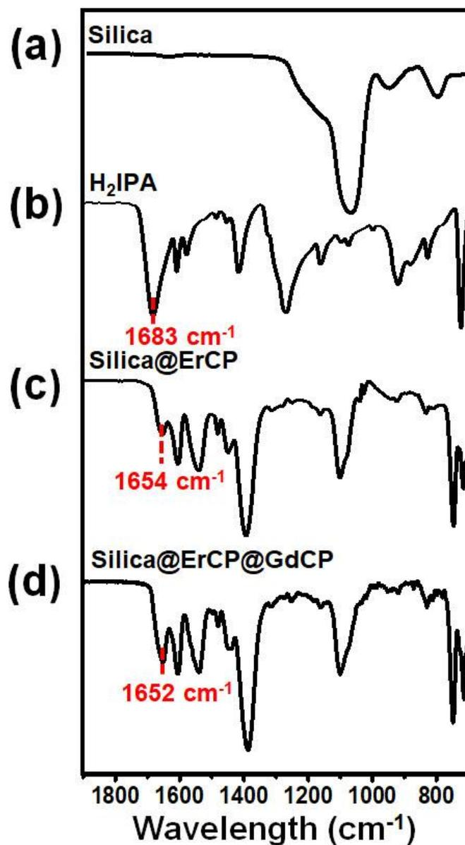
**Fig. S1.** IR spectra of (a) carboxylic acid-terminated silica, (b) H<sub>2</sub>IPA, (c) core-shell of silica@ErCP, and (d) silica-templated CP double layer of silica@ErCP@GdCP.
