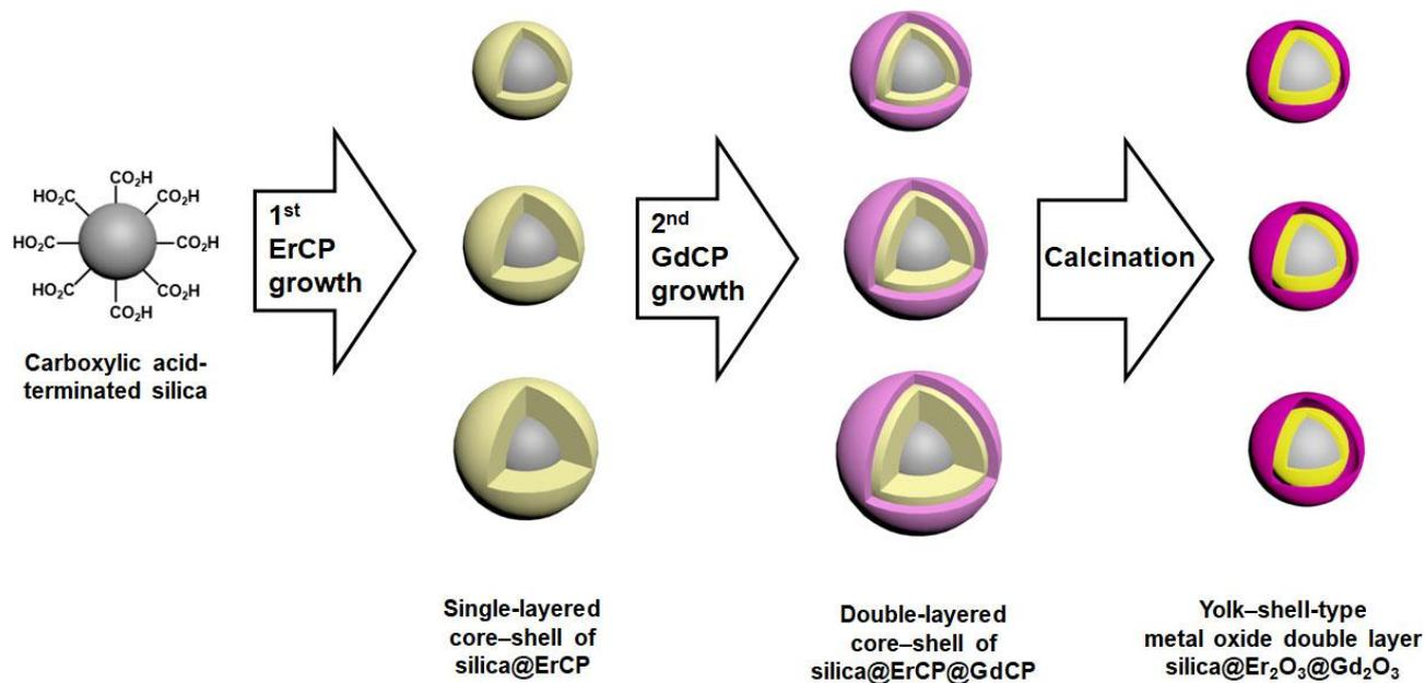
**Scheme S1.** Schematic representation for the construction of yolk-shell-type metal oxide double layers (silica@M<sub>x</sub>O<sub>y</sub>@M'<sub>x'</sub>O<sub>y'</sub>) with various intervals between the yolk and shell metal oxide.
