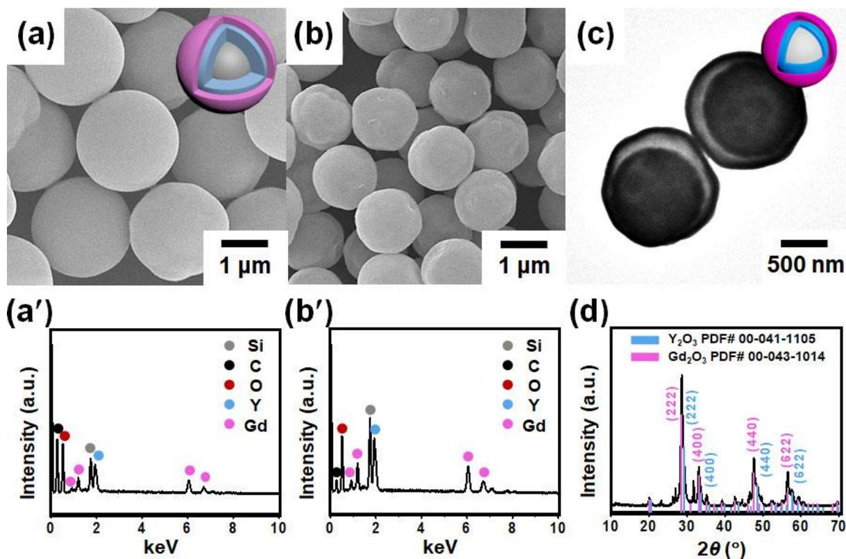
**Fig. S5.** (a) SEM image and (a') EDX spectrum of silica@YCP@GdCP. (b) SEM image, (b') EDX spectrum, (c) TEM image, and (d) PXRD pattern of yolk–shell-type metal oxide double layer of silica@Y<sub>2</sub>O<sub>3</sub>@Gd<sub>2</sub>O<sub>3</sub>.
