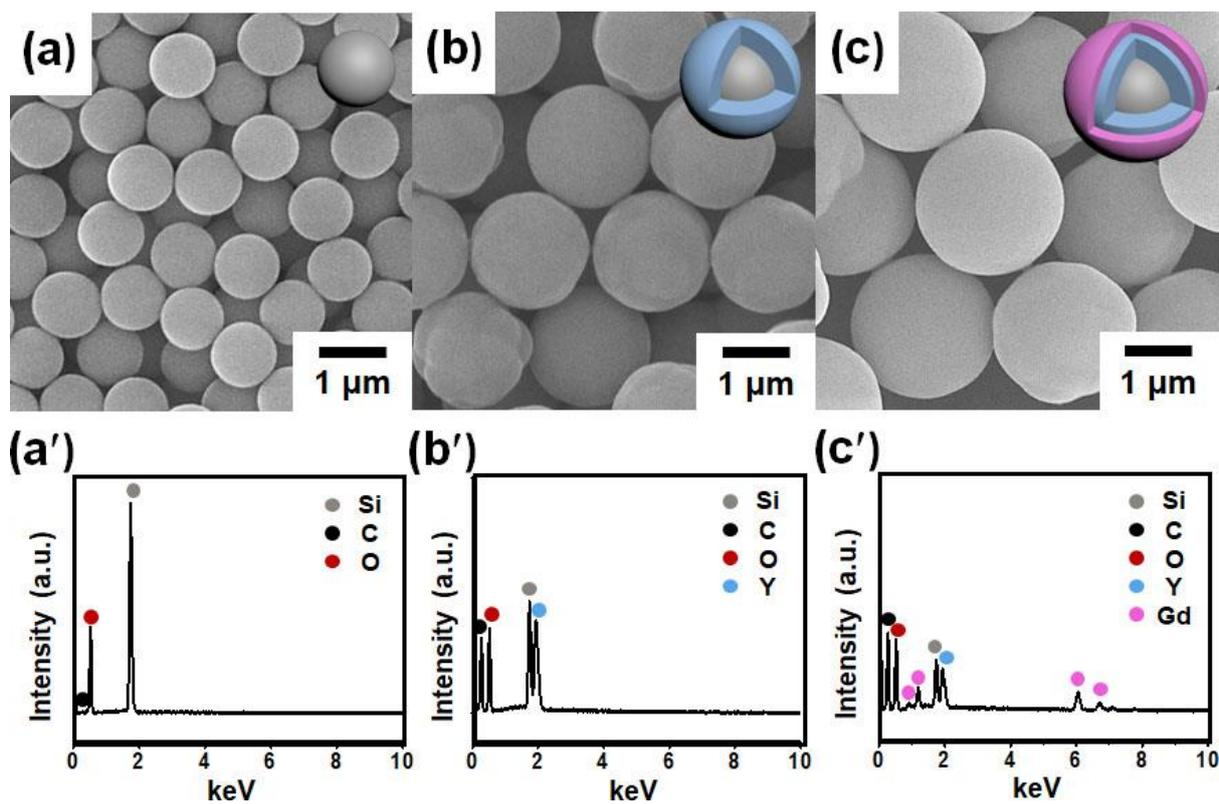
**Fig. S4.** SEM images of (a) carboxylic acid-terminated silica, (b) core-shell of silica@YCP, and (c) silica-templated CP double layer of silica@YCP@GdCP. EDX spectra of (a') carboxylic acid-terminated silica, (b') silica@YCP, and (c') silica@YCP@GdCP.
