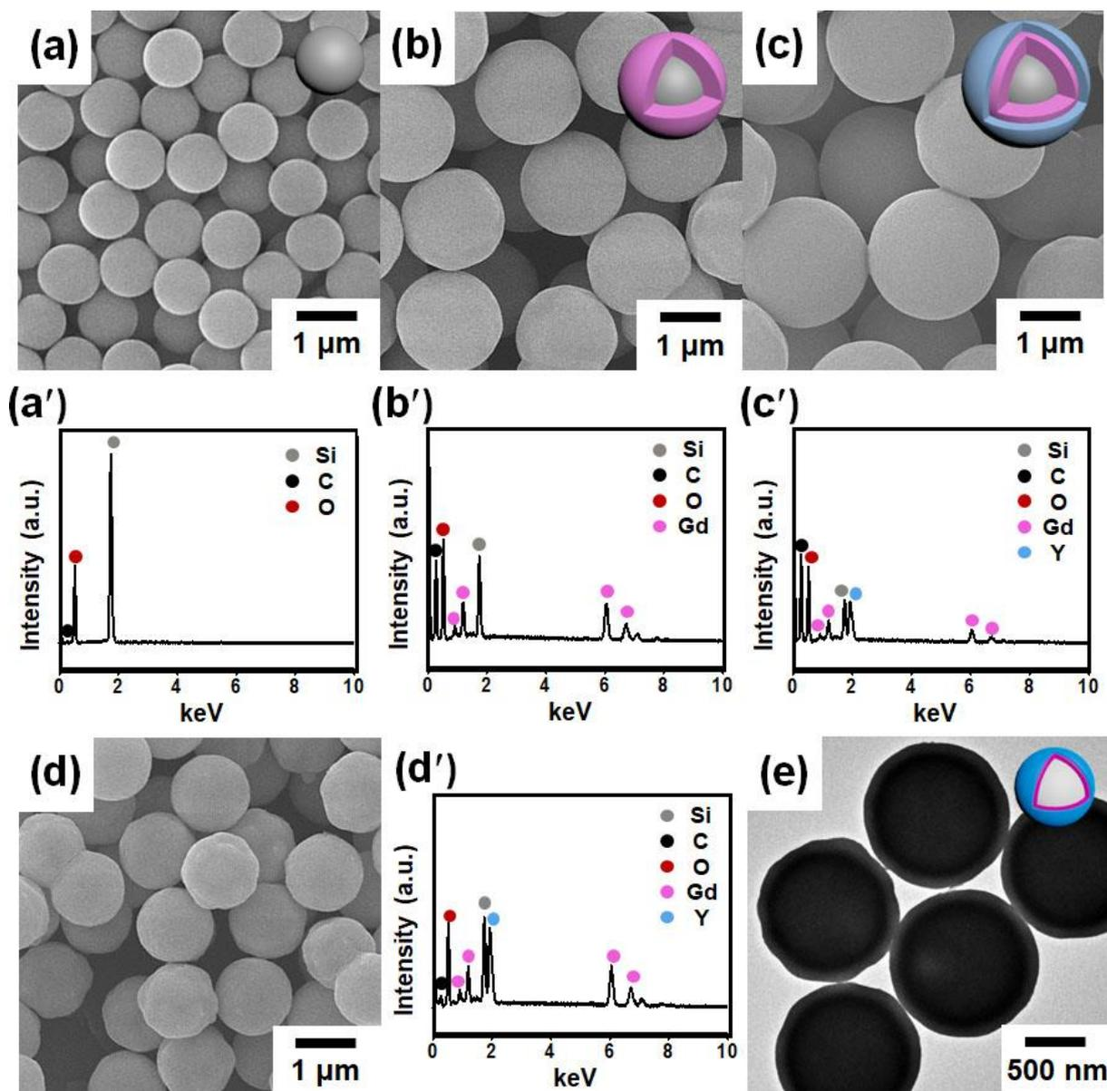
**Fig. S9.** SEM images of (a) carboxylic acid-terminated silica, (b) core-shell of silica@GdCP, and (c) silica-templated CP double layer of silica@GdCP@YCP. EDX spectra of (a') carboxylic acid-terminated silica, (b') silica@GdCP, and (c') silica@GdCP@YCP. (d) SEM image, (d') EDX spectrum, and (e) TEM image of core-shell-type metal oxide double layers of silica@Gd<sub>2</sub>O<sub>3</sub>@Y<sub>2</sub>O<sub>3</sub>.
