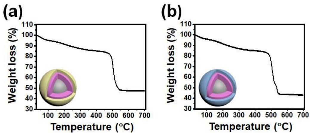
**Fig. S11.** TGA curves of double-layered core-shell microspheres of (a) silica@GdCP@ErCP and (b) silica@GdCP@YCP.
