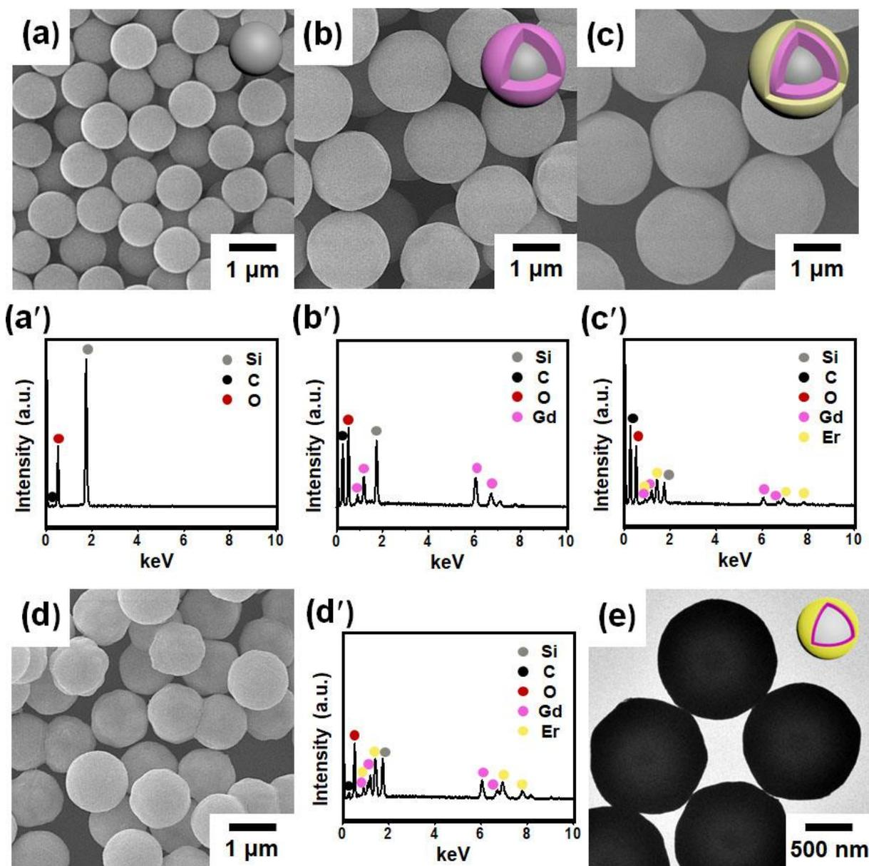
**Fig. S8.** SEM images of (a) carboxylic acid-terminated silica, (b) core-shell of silica@GdCP, and (c) silica-templated CP double layer of silica@GdCP@ErCP. EDX spectra of (a') carboxylic acid-terminated silica, (b') silica@GdCP, and (c') silica@GdCP@ErCP. (d) SEM image, (d') EDX spectrum, and (e) TEM image of core-shell-type metal oxide double layers of silica@Gd<sub>2</sub>O<sub>3</sub>@Er<sub>2</sub>O<sub>3</sub>.
