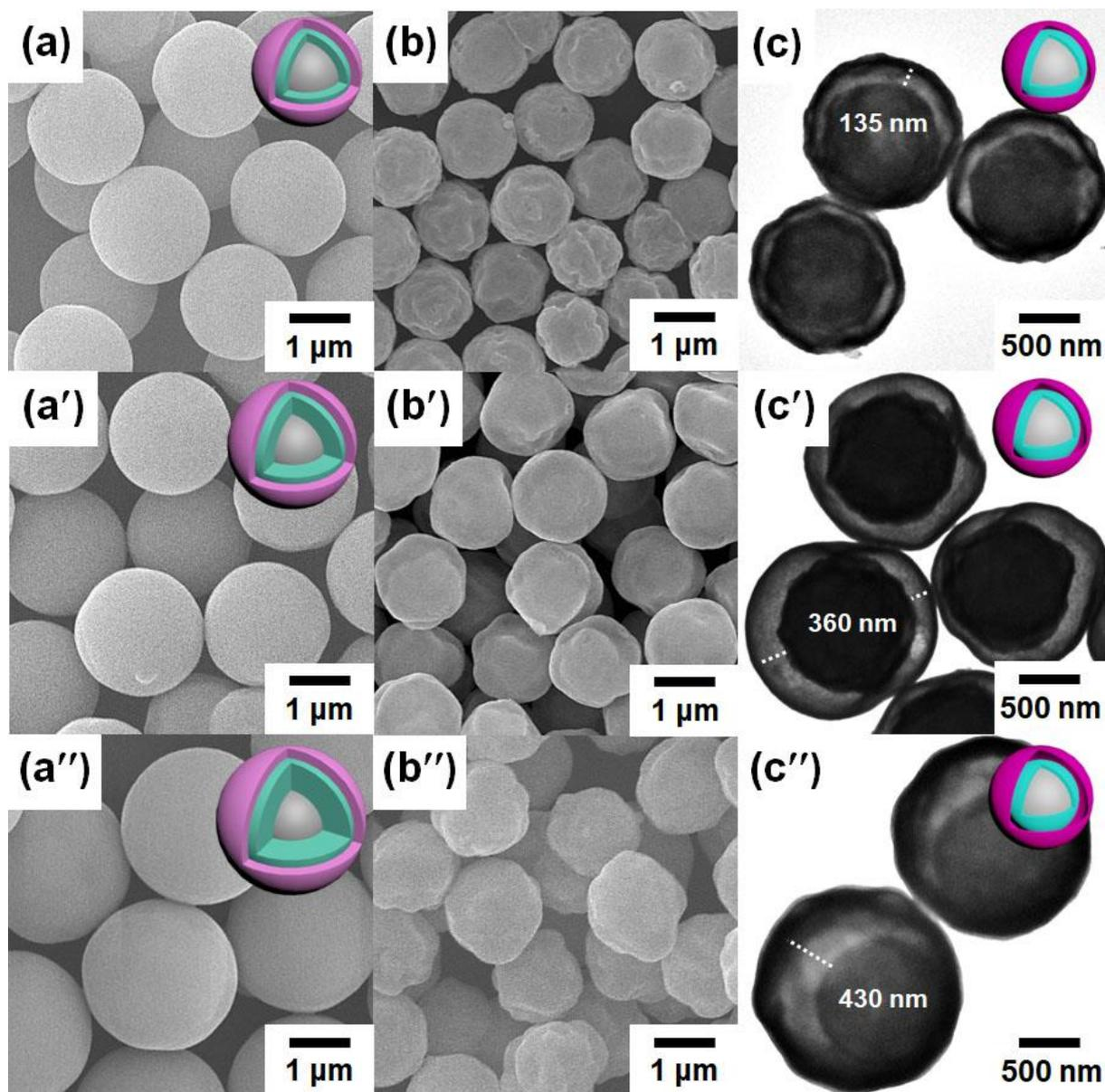
**Fig. S14.** Preparation of yolk–shell-type metal oxide double layers (silica@Tb<sub>4</sub>O<sub>7</sub>@Gd<sub>2</sub>O<sub>3</sub>) with various intervals between the yolk and shell metal oxide. (a, a', a'') SEM images of three different silica@TbCP@GdCP samples with various TbCP thicknesses of 255, 435, or 550 nm. (b, b', b'') SEM images and (c, c', c'') TEM images of the resulting yolk–shell-type metal oxide double layers of silica@Tb<sub>4</sub>O<sub>7</sub>@Gd<sub>2</sub>O<sub>3</sub>.
