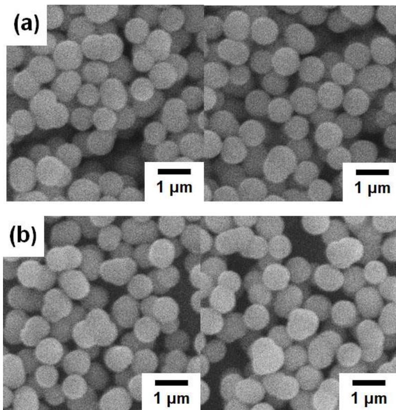
**Fig. S2.** SEM images showing the formation of (a) ErCP and (b) GdCP with large size distribution.
