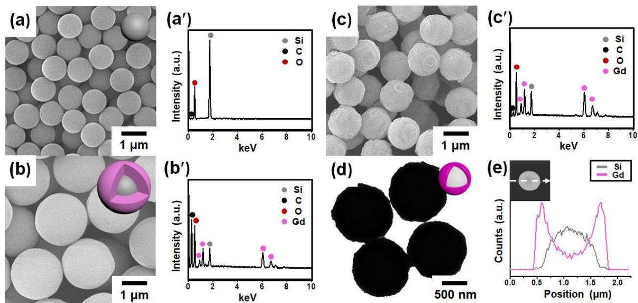
**Fig. S6.** SEM images of (a) carboxylic acid-terminated silica, (b) core-shell of silica@GdCP, and (c) silica@Gd<sub>2</sub>O<sub>3</sub>. EDX spectra of (a') carboxylic acid-terminated silica and (b') silica@GdCP, and (c') silica@Gd<sub>2</sub>O<sub>3</sub>. (d) TEM image and (e) elemental line-scanning profiles of silica@Gd<sub>2</sub>O<sub>3</sub>.
