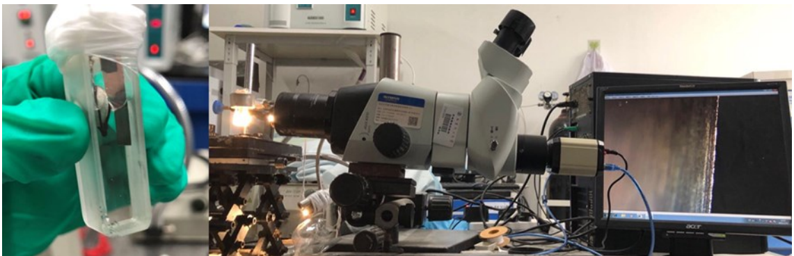
Figure S8. Photograph of the battery undergoing in-situ Li plating measurement.
