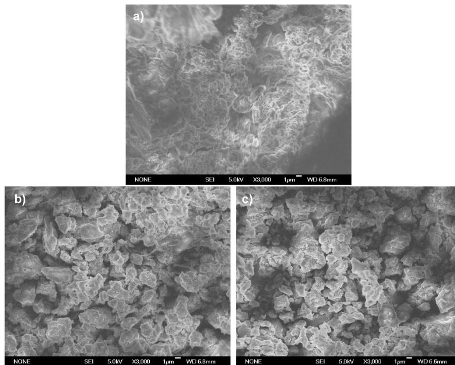
**Fig. S1** Scanning electron microscopy (SEM) images: (a) CMP-1, (b) KCMP-F1 and (c) KCMP-M1.
